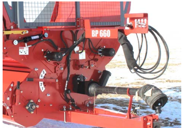
Route Hoses through Non-Abrasion Cover and through Hose Holder
