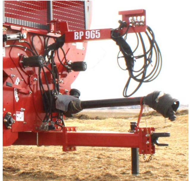
Route Hoses in Abrasion Cover and Holder
