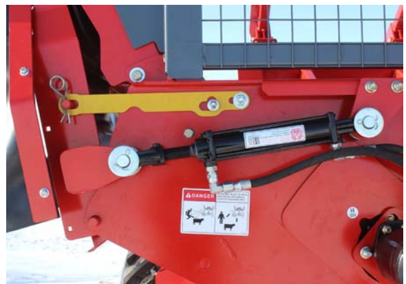
Installed Cylinder Bracket and Lock Strap
