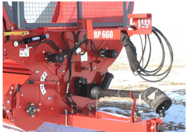
Route Hoses Through Non-Abrasion Cover and Hose Holder
