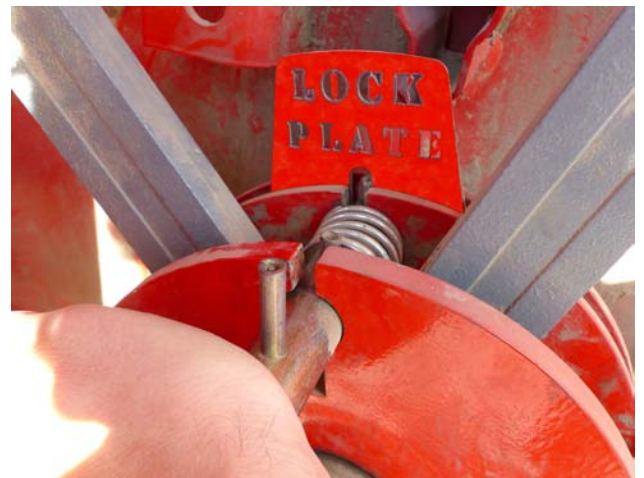
Push and Twist Clutch Pin
