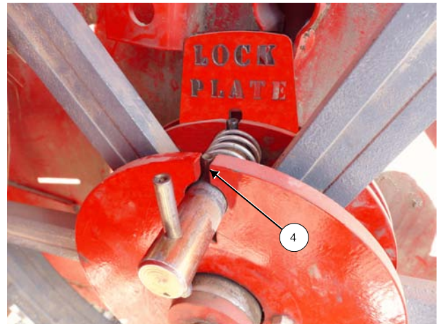
Twist Clutch Pin to Disengage Drive
