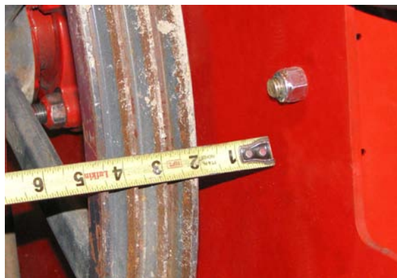
Measure Distance - Large Sheave to Tub Wall
