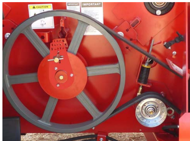
Check Chopper Drive Belt Tension
