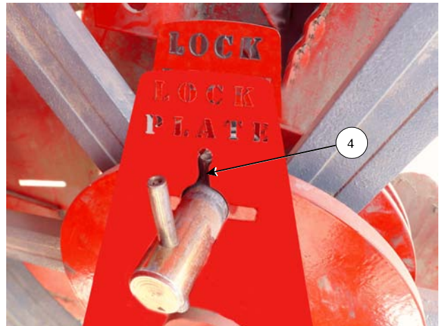
Twist Clutch Pin to Disengage Drive
