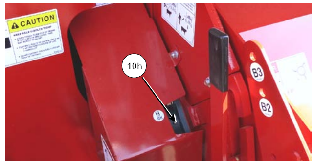
Grease Rear Rotor Bearing
