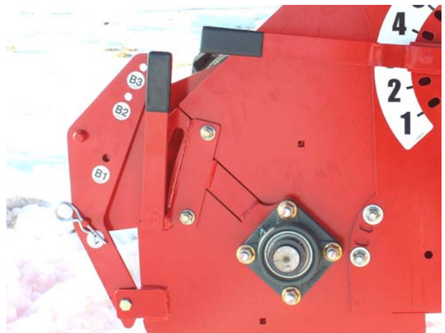
Replace Door and Connect Door Supports
