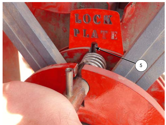
Push and Twist Clutch Pin (Front Lock Plate Not Shown for Clarity)
