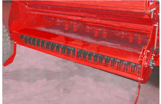
Disconnect Discharge Door Supports
