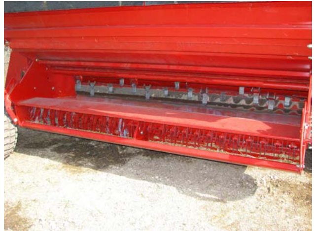
Remove Twine/Wrap from Knives & Rotor
