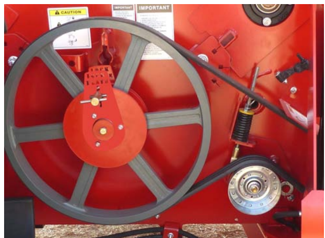
Put the New Drive Belt in Place
