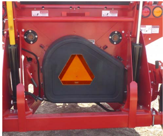
Close and Fasten the Drive Guard Door
