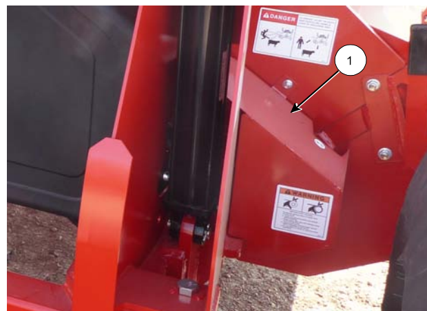
Remove Rear Sheave Shield
