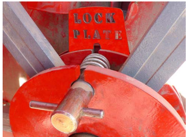
Locked Clutch Pin (Front Lock Plate Not Shown for Clarity)
