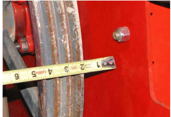
Measure Distance - Large Sheave to Tub Wall
