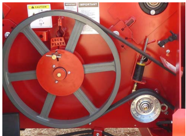
Put the New Drive Belt in Place
