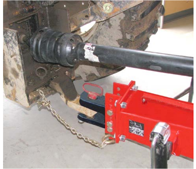
Adjust the Height of Hitch Tongue
