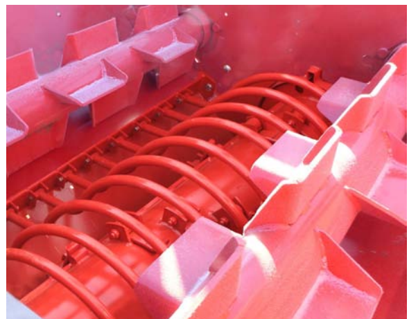
Remove Wrap/Twine from Feed Rollers
