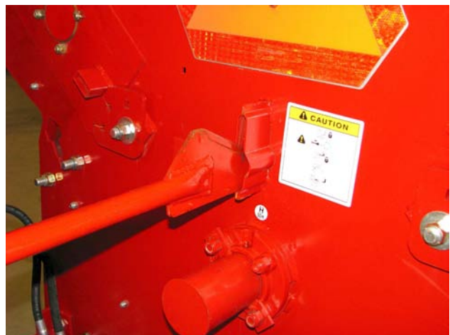
Insert Twine/Wrap Cutter with Blade Up
