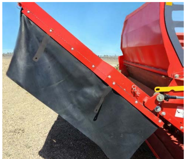
Side Curtains Loosened for Bunk or Windrow
