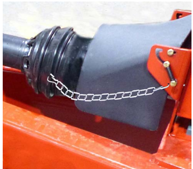
Connect Driveline Cover Chains
