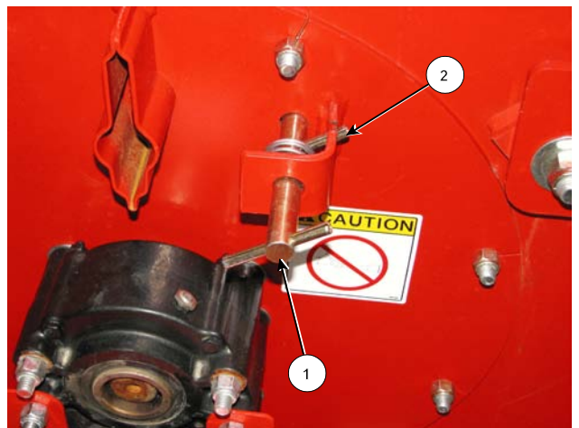
Remove the Flail Drum Lock
