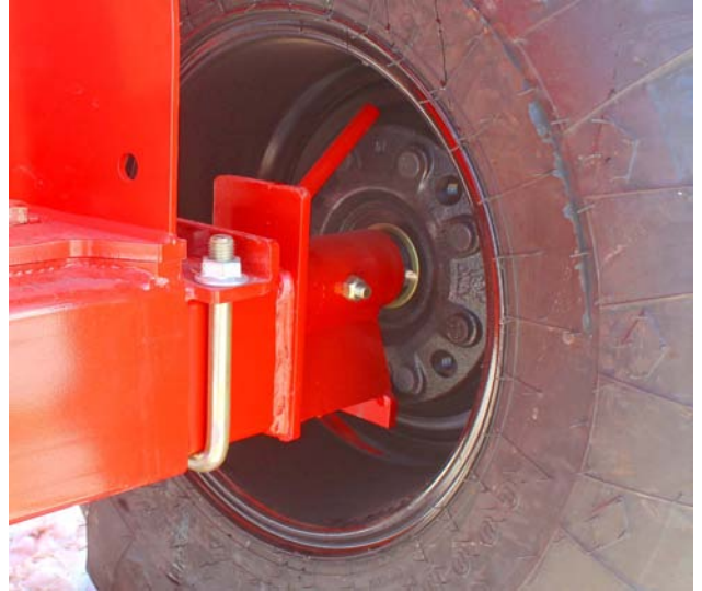
Remove Twine/Wrap from Spindle and Hub
