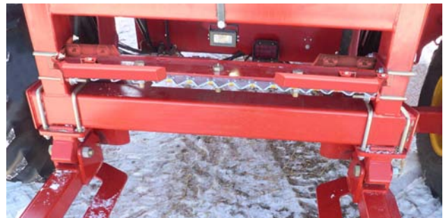
Forks Moved Out for Round Bales
