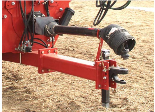
Place the Driveline in the Holder
