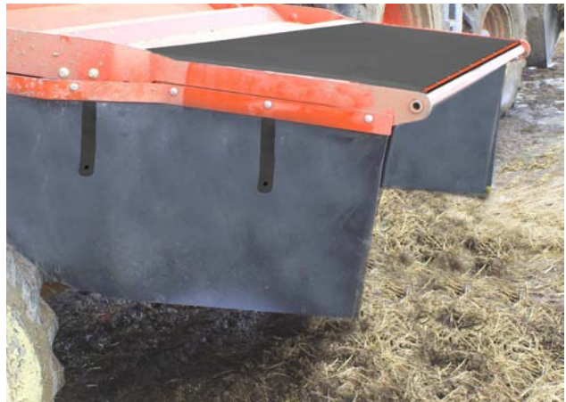
Rubber On Top of Door for Bedding
