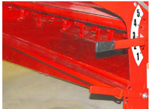
Re-Adjust Discharge Rate Lever (If needed)
