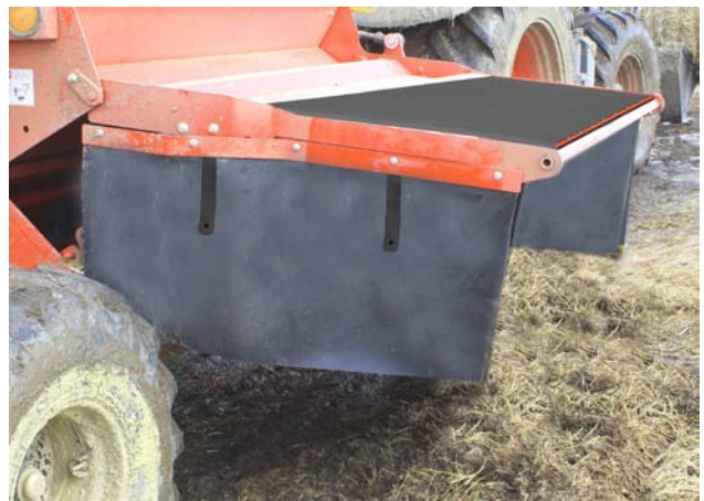
Rubber On Top of Door for Bedding
