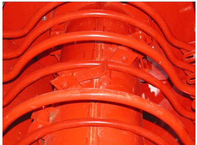
Move Flails Blocking the Knife Path
