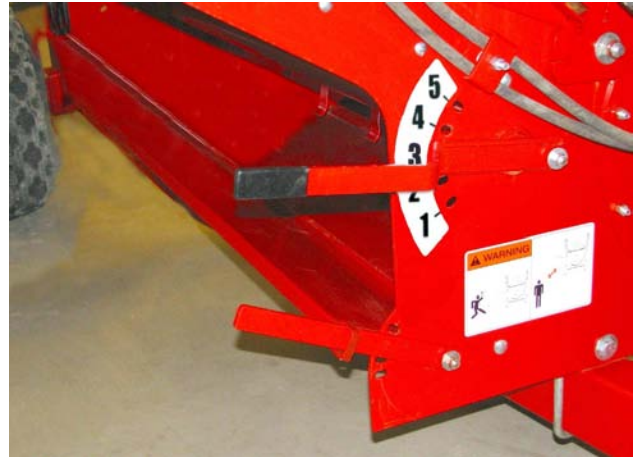
Move Flail Guard Rod Lever (to less than 5)
