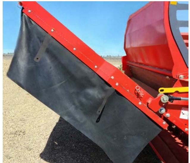
Side Curtains Loosened for Bunk or Windrow
