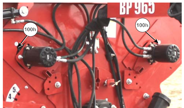
Grease Front Feed Roller Bearings (Motor Guards Not Shown for Clarity)
