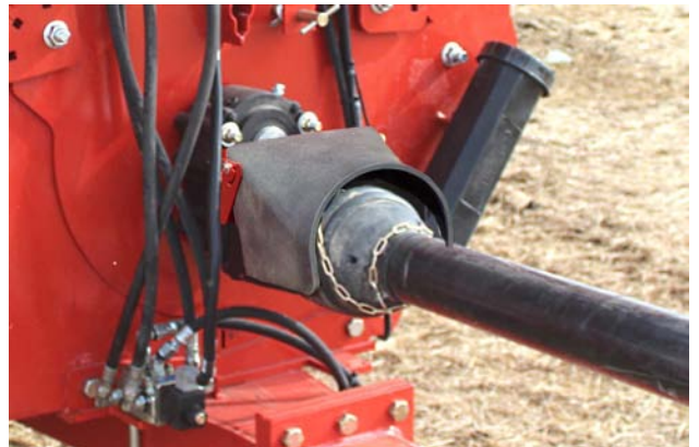
Ensure Driveline Shield is in Place
