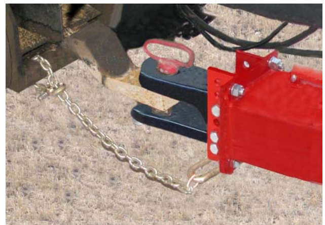
Disconnect Safety Chain and Hitch Pin
