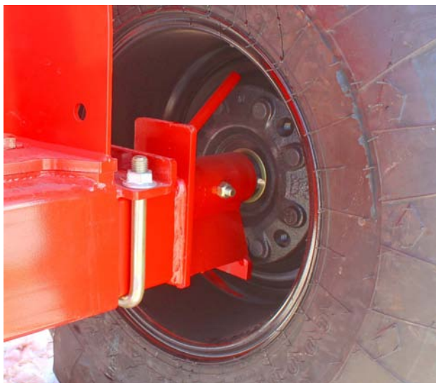
Remove Twine From the Spindle and Hub
