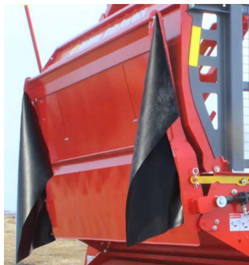
Discharge Door Raised - Rubber Secured
