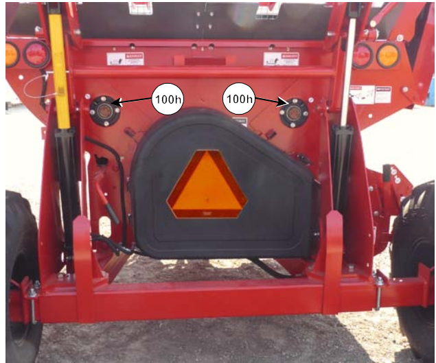
Grease Rear Feed Roller Bearings
