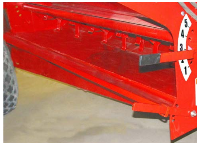
Set the Level of Lower Discharge Deflector
