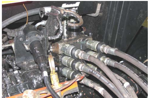
Disconnect Hydraulic Hoses & Electrical
