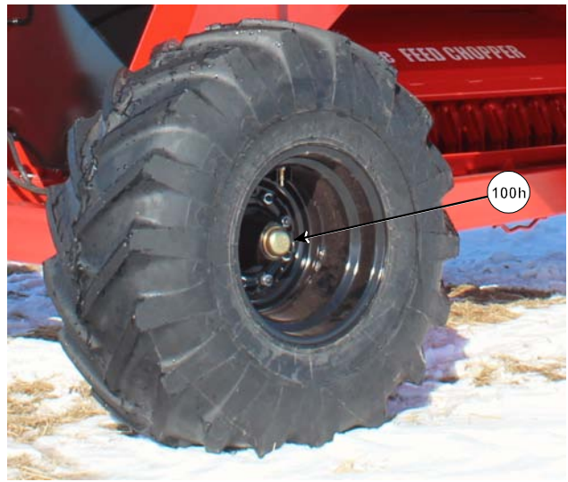
Grease Hubs on Spindles
