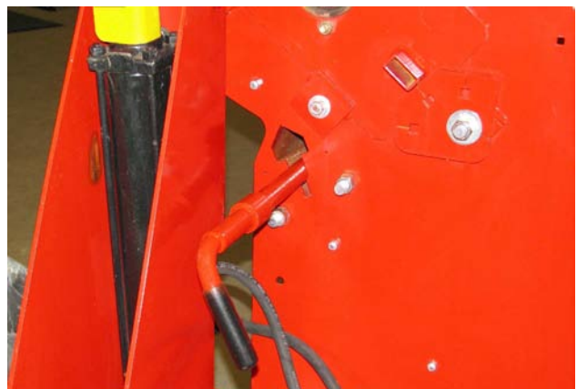
Replace Twine Cutter Into Storage Position
