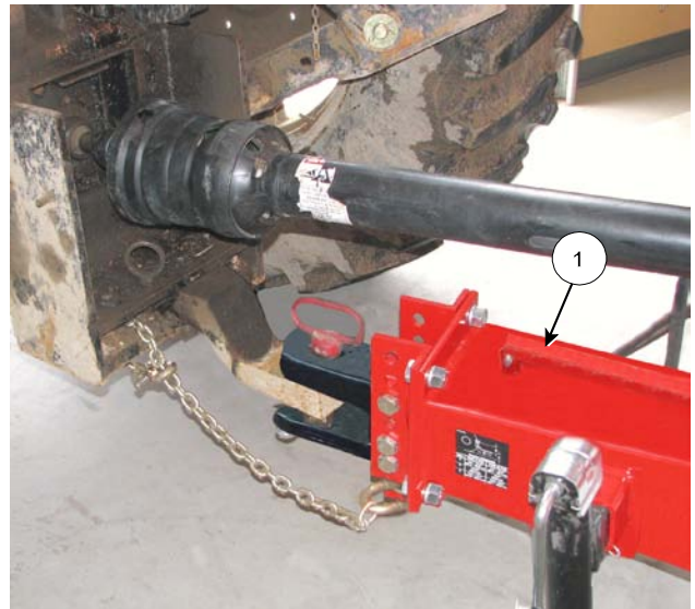
Connect Driveline to PTO
