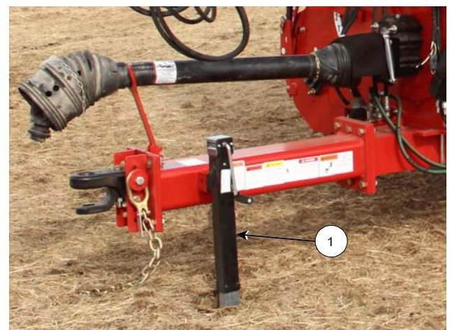
Lift Hitch with the Jack
