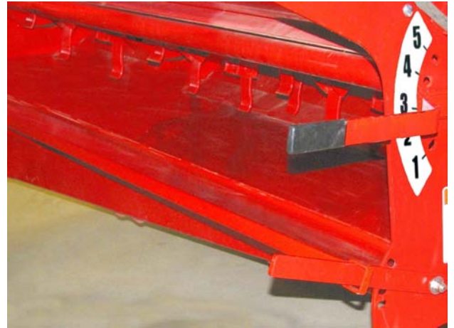
Re-Adjust Discharge Rate Lever (If needed)
