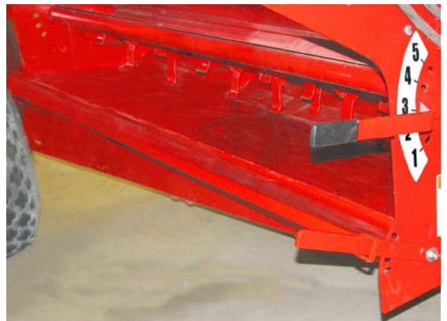
Set the Level of Lower Discharge Deflector
