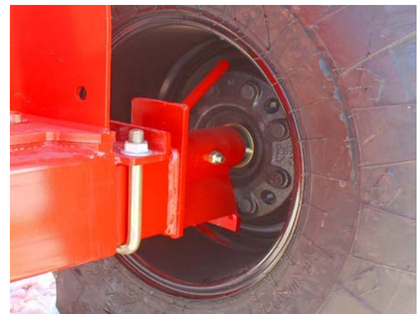
Remove Twine/Wrap from Spindle and Hub
