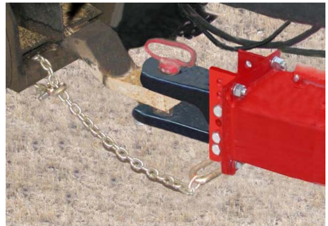
Disconnect Safety Chain and Hitch Pin
