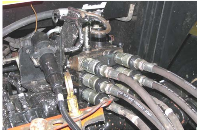
Disconnect Hydraulic Hoses & Electrical
