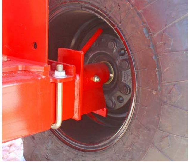
Remove Twine From the Spindle and Hub
