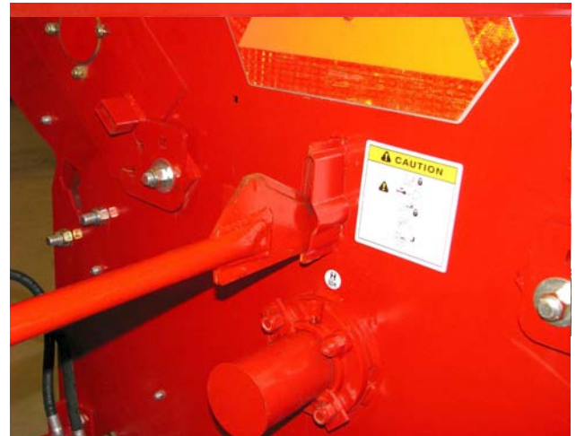
Insert Twine/Wrap Cutter with Blade Up
