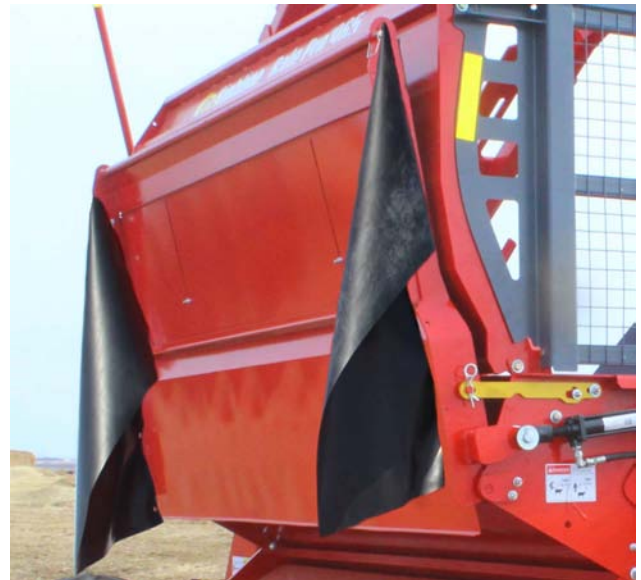
Discharge Door Raised - Rubber Secured
