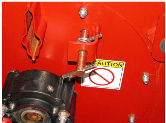
Remove the Flail Drum Lock
