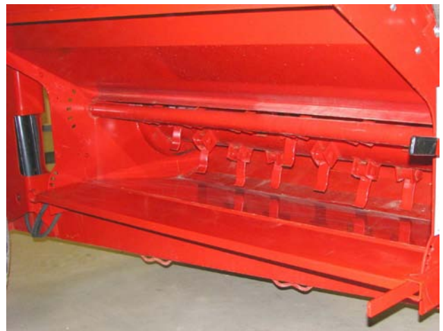
Check and Clean Flail Drum Area
