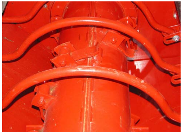
Move Flails Blocking the Knife Path
