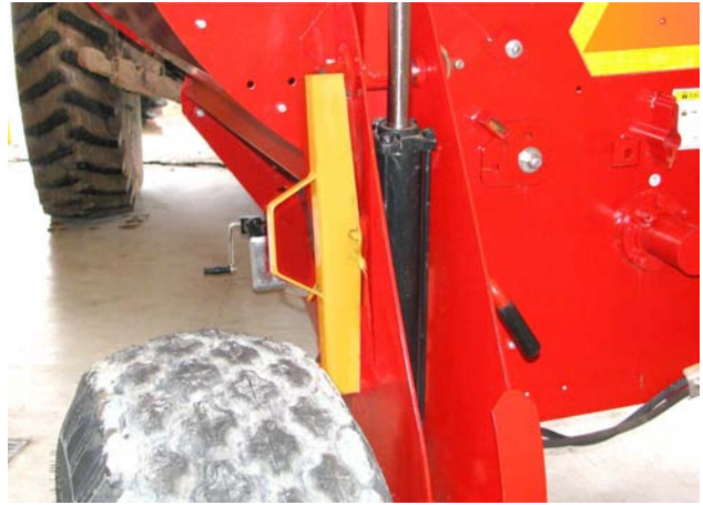
Remove Fork Lock - Place in Storage
