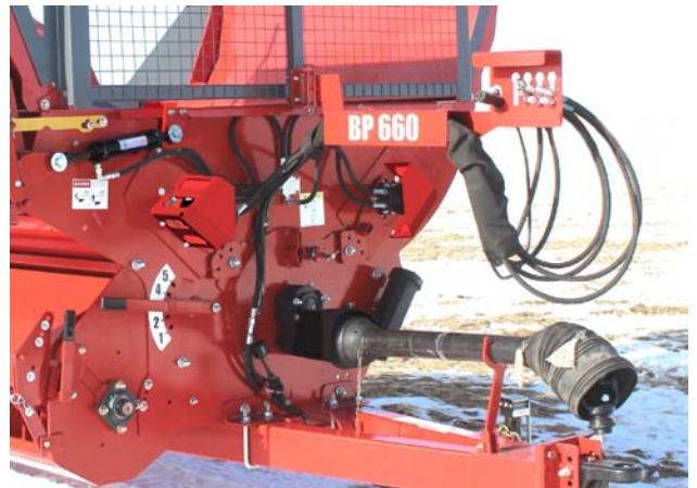
Hoses and Driveline in Supports
