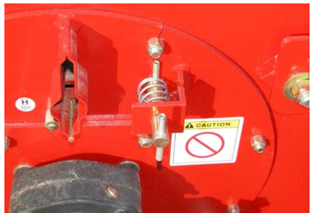
Engage the Flail Drum Lock
