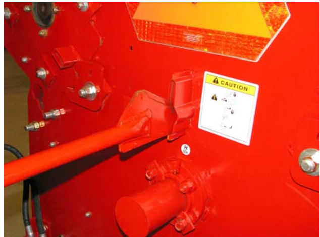
Insert Twine Cutter with Blade Up
