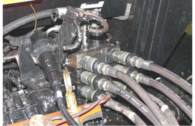
Disconnect Hydraulic Hoses & Electrical
