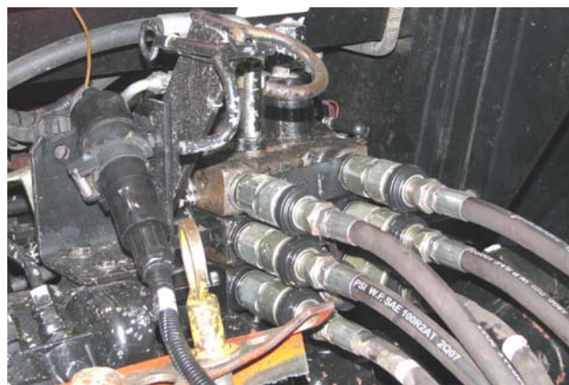
Attach Hydraulics and Electrical
