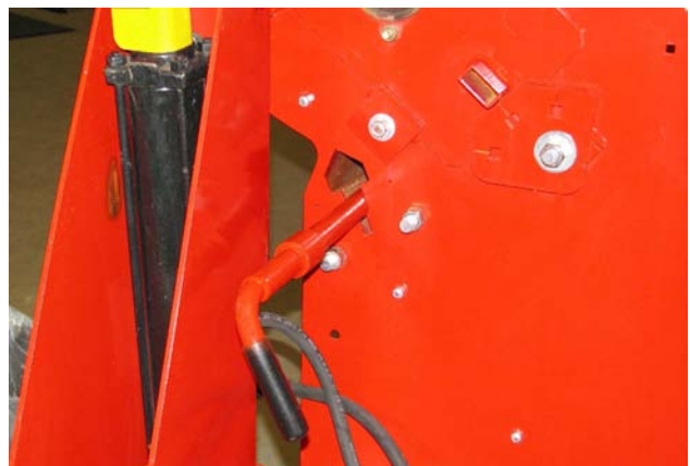
Replace Twine Cutter Into Storage Position
