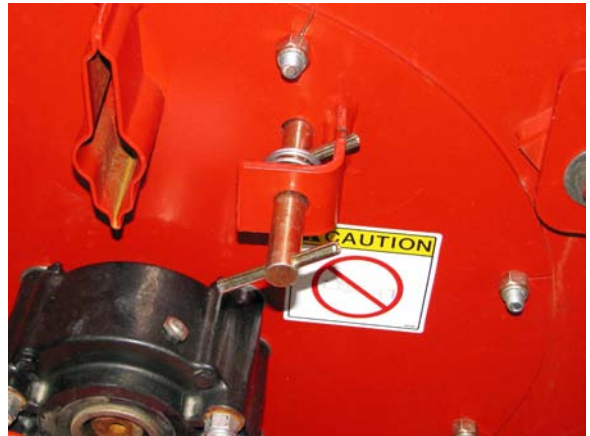
Remove the Flail Drum Lock
