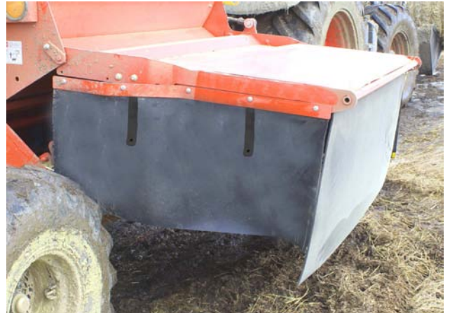
Set the Upper Deflector Door (Windrowing Shown)
