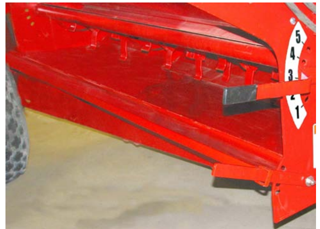
Set Level of the Lower Discharge Deflector
