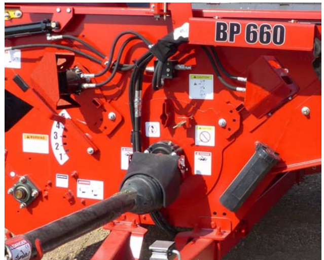
Ensure Driveline Shield is in Place
