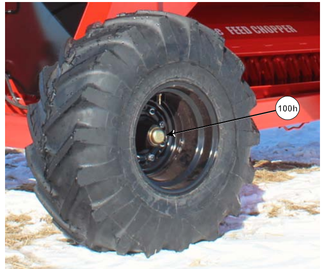
Grease Hubs on Both Spindles
