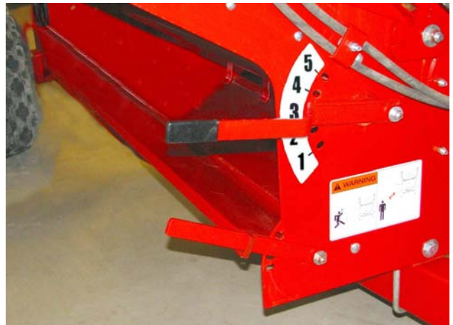
Re-Adjust Discharge Rate Lever (If needed)
