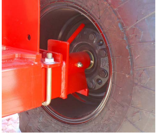
Remove Twine From the Spindle and Hub
