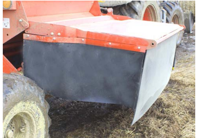
Set the Upper Deflector Door (Windrowing Shown)
