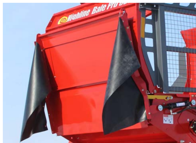
Discharge Door Raised - Rubber on Top of Door
