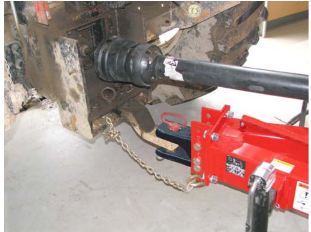
Disconnect from the Tractor
