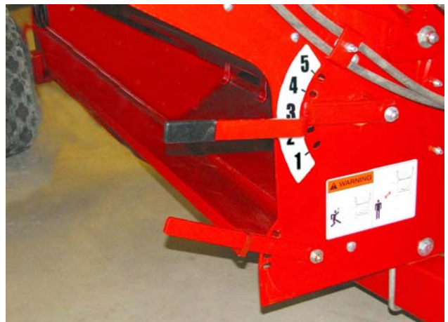
Re-Adjust Discharge Rate Lever (If needed)
