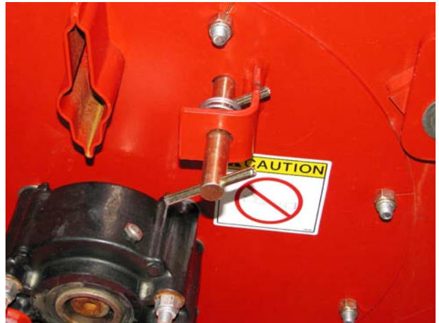
Remove the Flail Drum Lock
