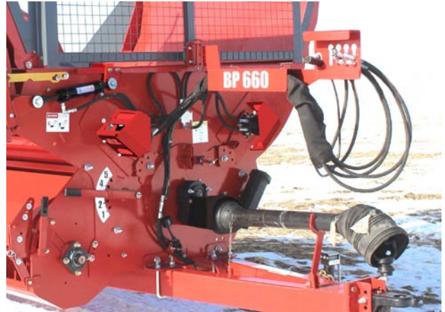
Hoses and Driveline in Supports
