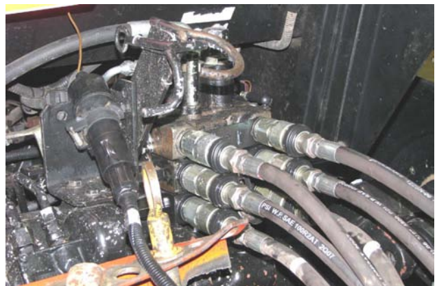
Disconnect Hydraulic Hoses & Electrical
