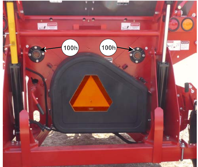
Grease Rear Feed Roller Bearings
