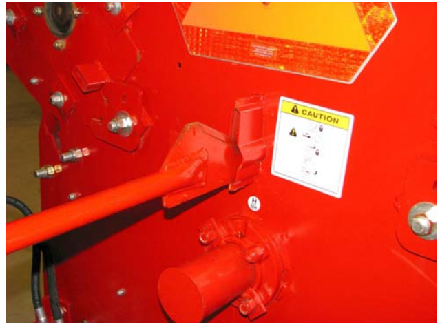
Insert Twine Cutter with Blade Up
