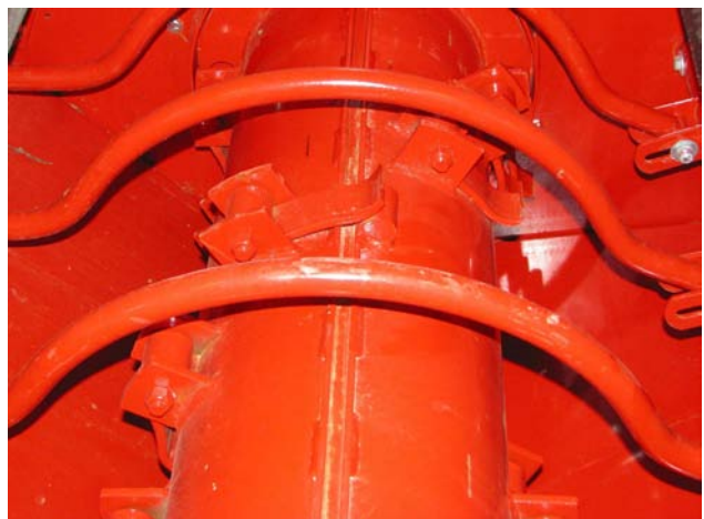
Move Flails Blocking the Knife Path
