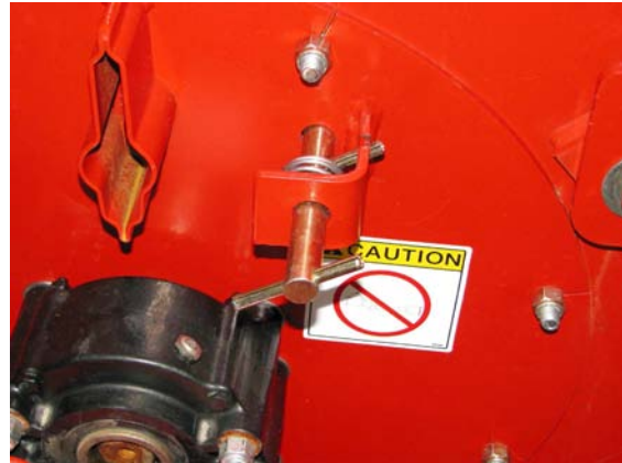
Remove the Flail Drum Lock
