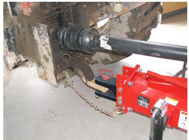
Remove Driveline and Safety Chain
