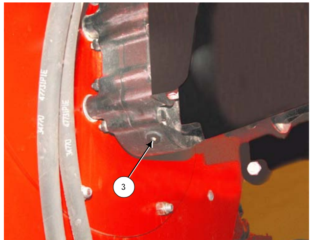
Drain Oil From Gearbox
