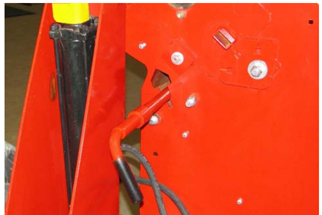
Replace Twine Cutter Into Storage Position
