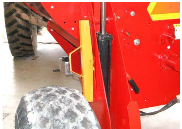
Remove Fork Lock - Place in Storage
