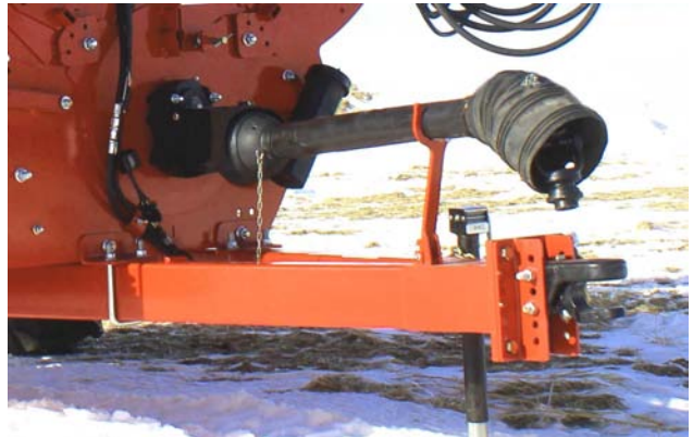
Place the Driveline in the Holder
