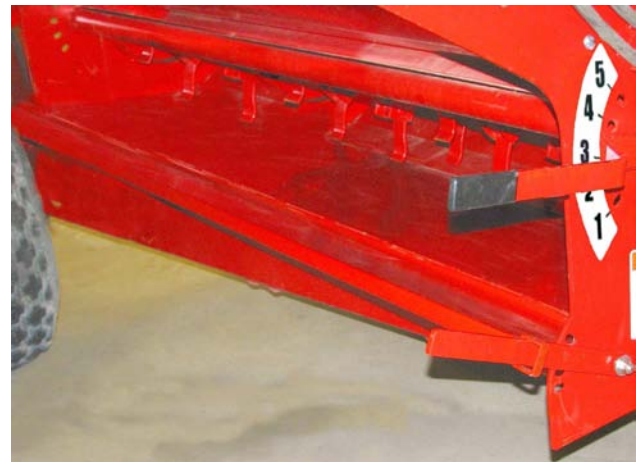
Set Level of the Lower Discharge Deflector
