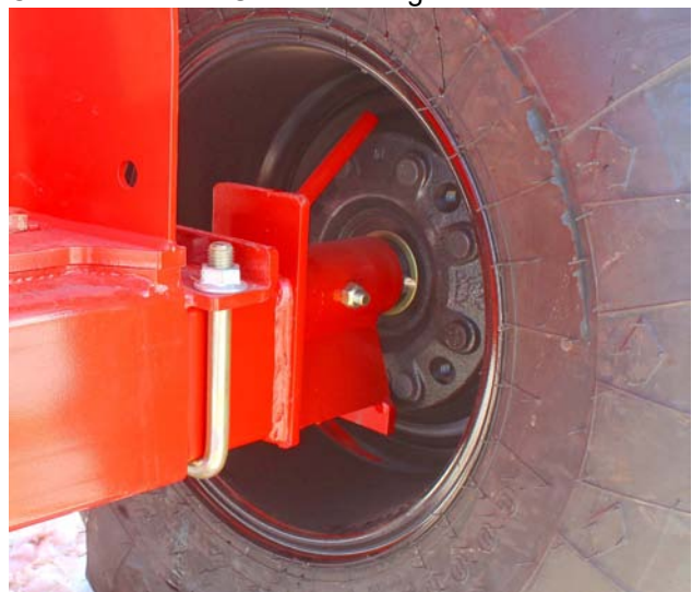
Remove Wrap/twine from Spindle & Hub
