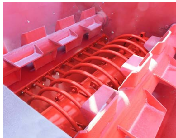
Remove Wrap/Twine from Feed Rollers
