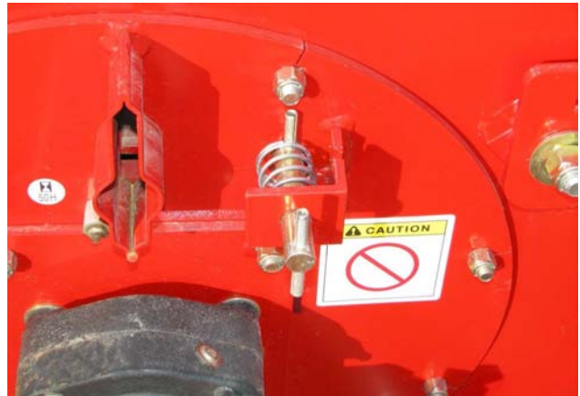
Engage the Flail Drum Lock
