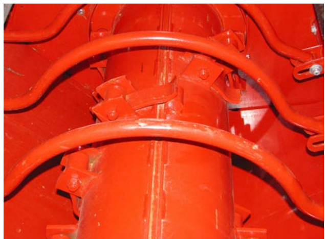
Move Flails Blocking the Knife Path
