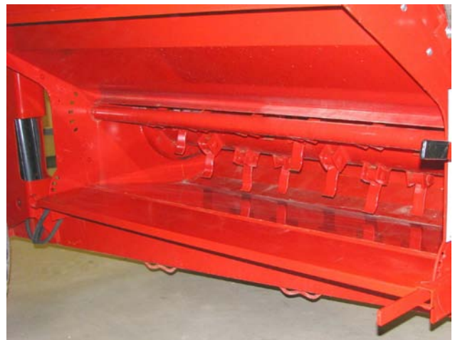
Check and Clean Flail Drum Area
