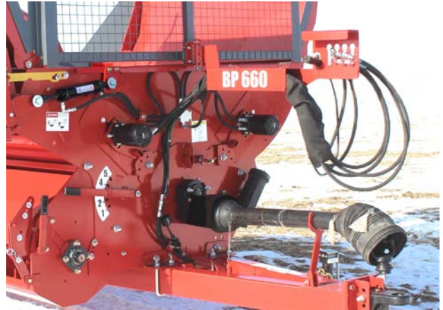
Hoses and Driveline in Supports
