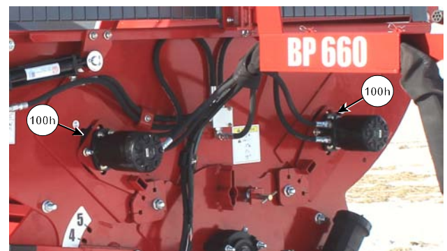
Grease Front Feed Roller Bearings
