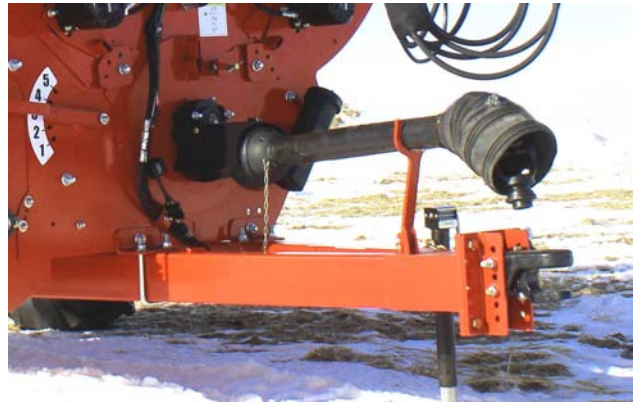
Place the Driveline in the Holder
