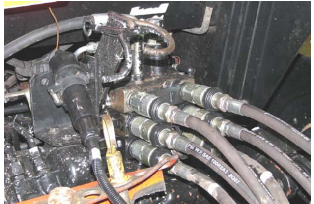
Inspect Hydraulic Hoses
