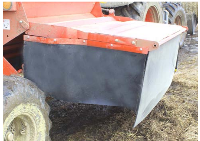
Set the Upper Deflector Door (Windrowing Shown)
