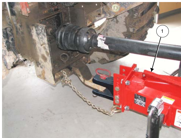
Connect Driveline to PTO
