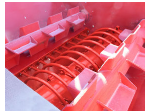
Remove Wrap/Twine from Feed Rollers
