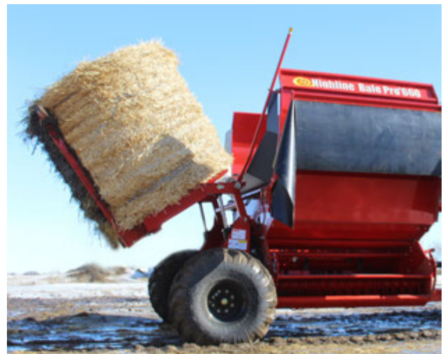
Raise Bale into Processor Tub
