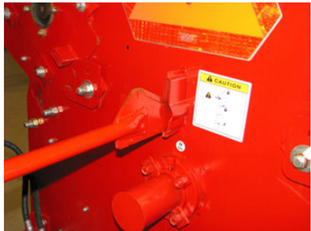
Insert Twine Cutter with Blade Up
