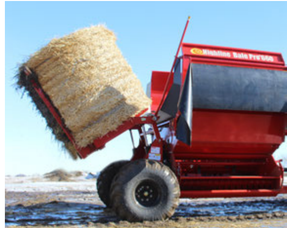
Stop Feed Rollers Before Loading Bale
