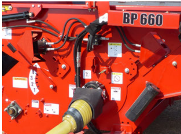
Ensure Driveline Shield is in Place
