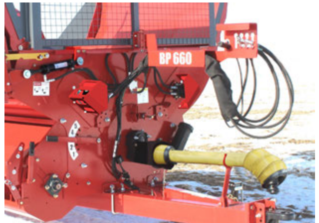
Hoses and Driveline in Supports
