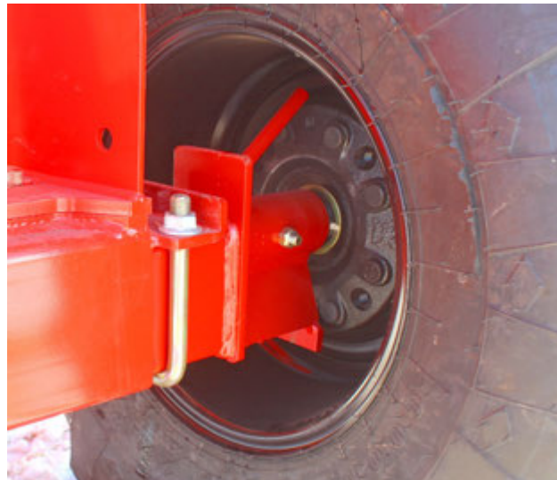
Remove Wrap/twine from Spindle & Hub
