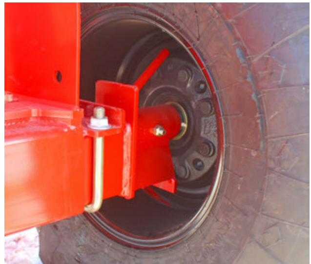
Remove Twine From Spindle and Hub
