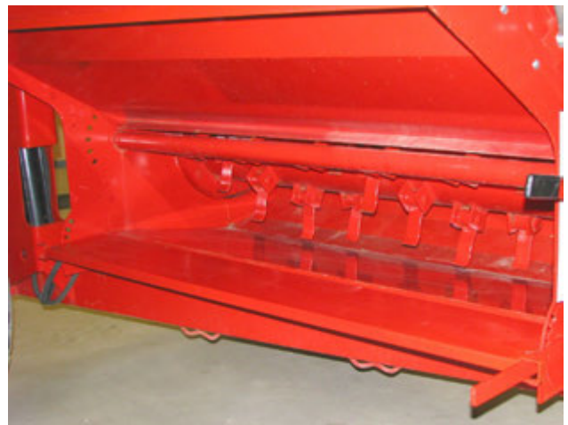
Check and Clean Flail Drum Area
