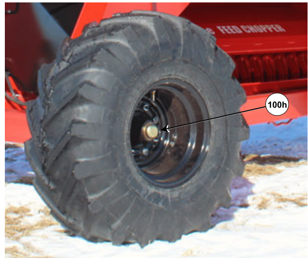
Grease Hubs on Both Spindles
