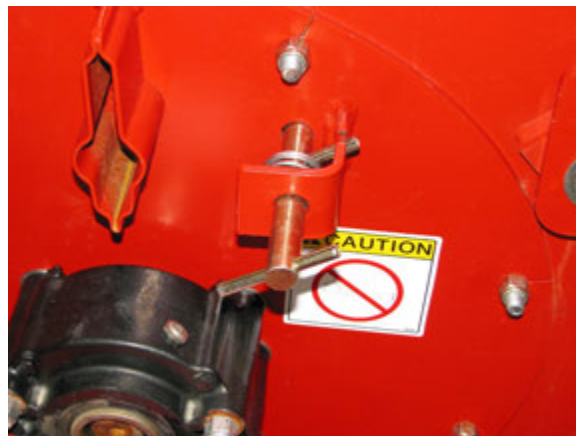
Remove the Flail Drum Lock
