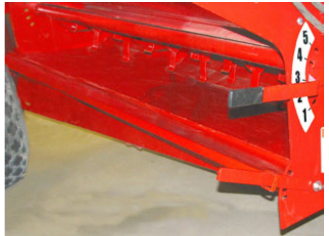
Set Level of the Lower Discharge Deflector
