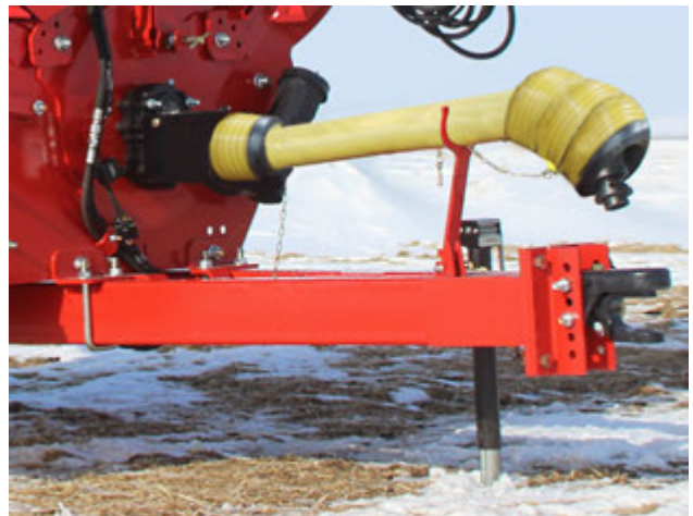
Place the Driveline in the Holder
