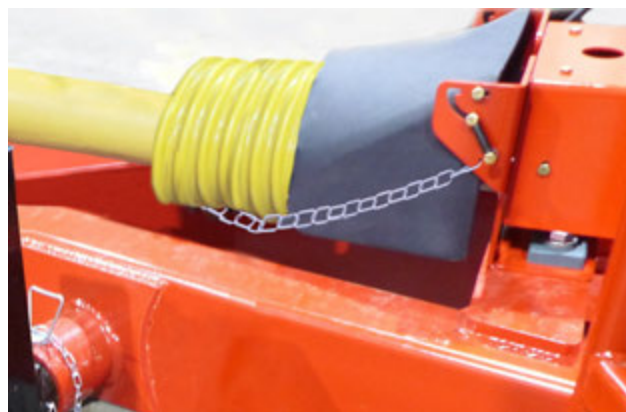
Connect Driveline Cover Chains
