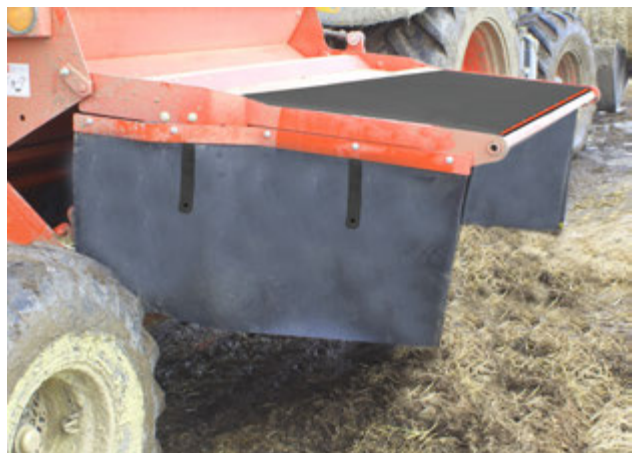
Rubber On Top of Door for Bedding
