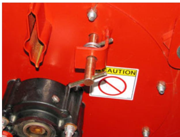
Remove the Flail Drum Lock
