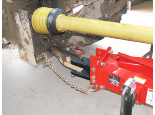
Adjust Height of Hitch Tongue
