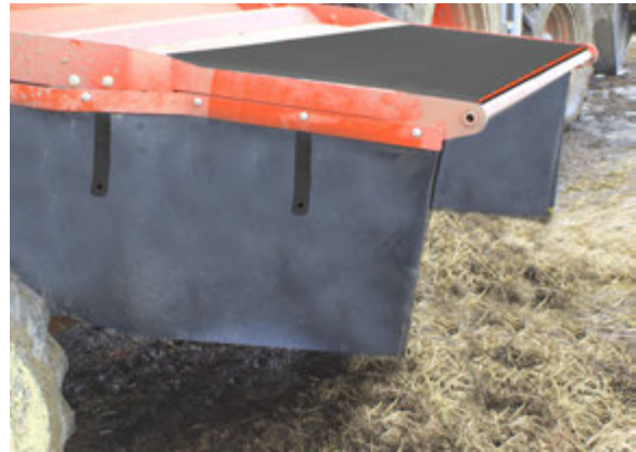
Rubber On Top of Door for Bedding
