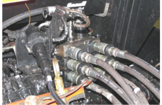
Disconnect Hydraulic Hoses & Electrical
