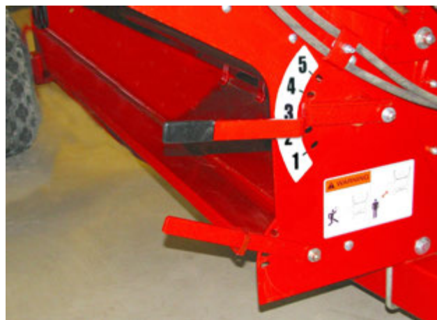
Re-Adjust Discharge Rate Lever (If needed)
