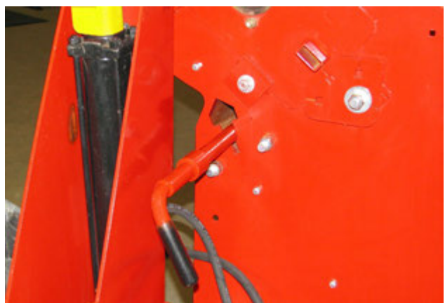
Replace Twine Cutter Into Storage Position
