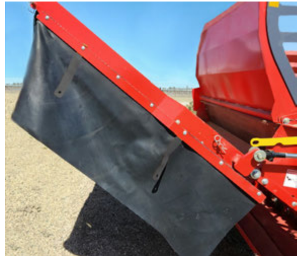
Side Curtains Loosened for Bunk or Windrow
