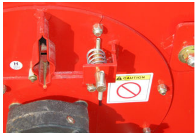
Engage the Flail Drum Lock
