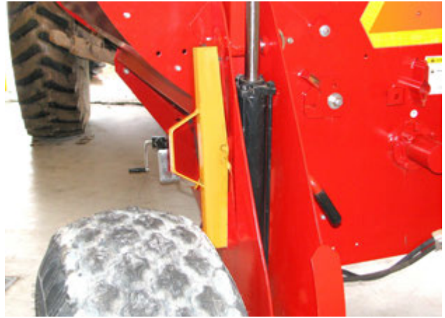
Remove Fork Lock - Place in Storage
