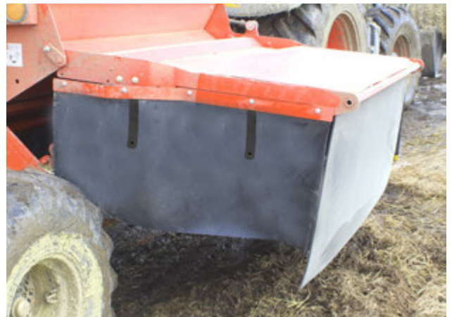
Set the Upper Deflector Door (Windrowing Shown)
