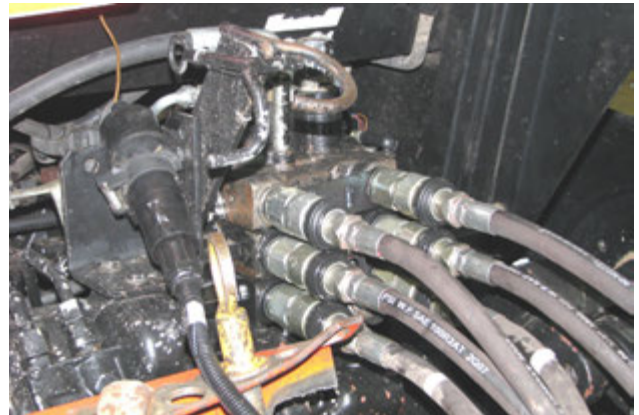
Inspect Hydraulic Hoses
