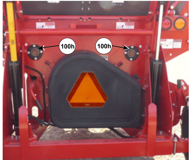
Grease Rear Feed Roller Bearings
