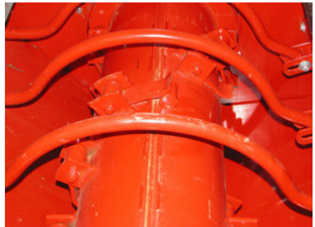
Move Flails Blocking the Knife Path
