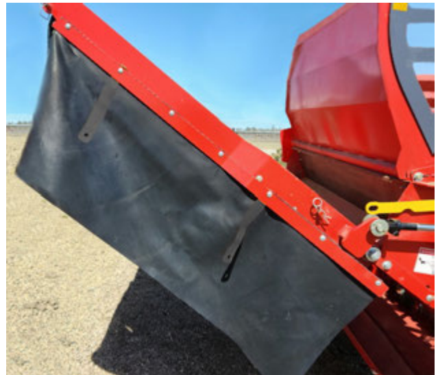
Side Curtains Loosened for Bunk or Windrow
