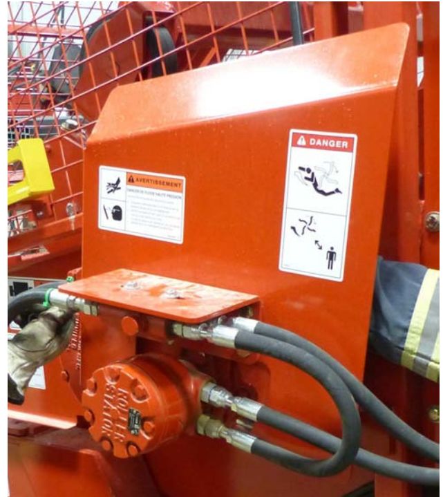
Installed Gearbox Shield
