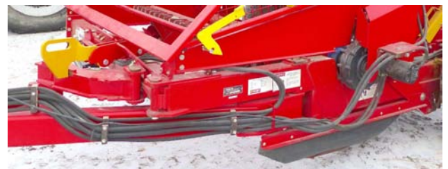
Route Hydraulic Hoses Through Hose Clamps
