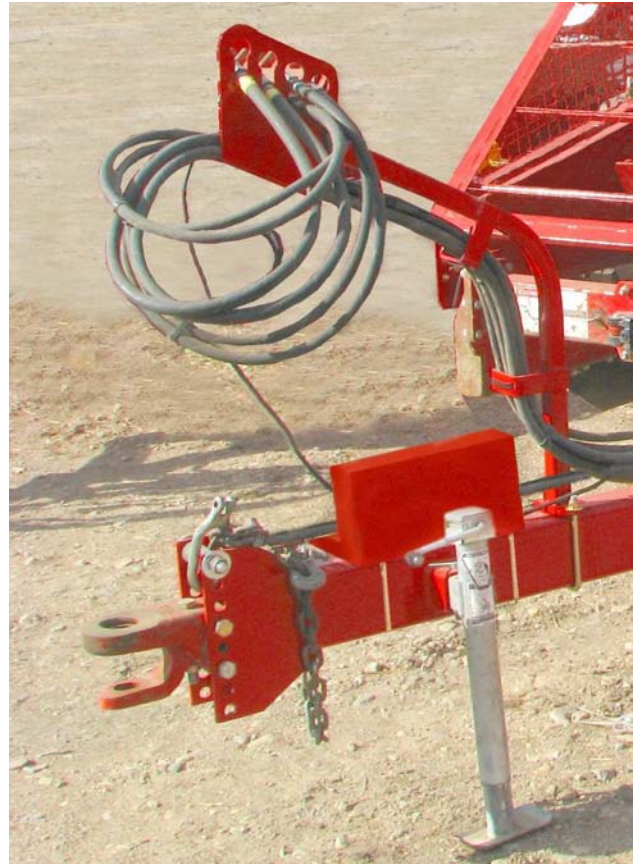
Route the Hoses in the Hitch Holder
