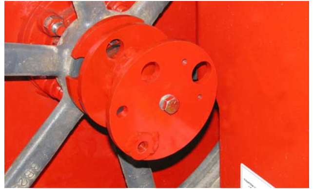
Fasten Clutch Body to Flail Drum Shaft
