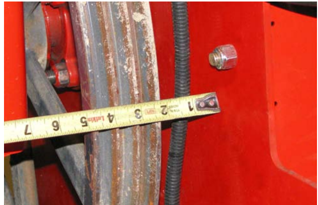
Measure the Sheave Distance
