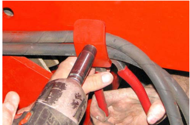
Remove The Rear Hose Clamp
