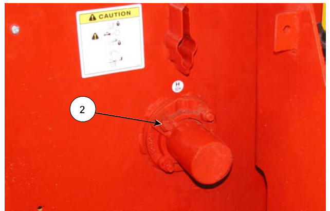
Remove Rear Flail Shaft Cover
