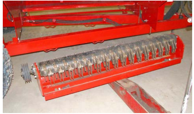
Support The Chopper Housing
