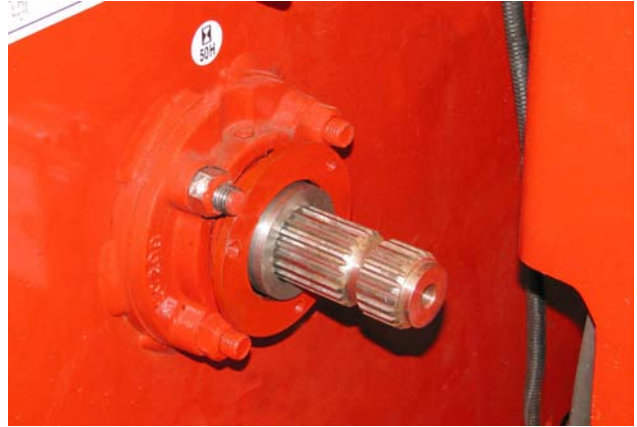
Retaining Plate Over The Spacer Ring
