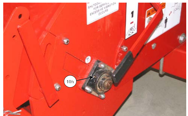
Grease Front Rotor Bearing
