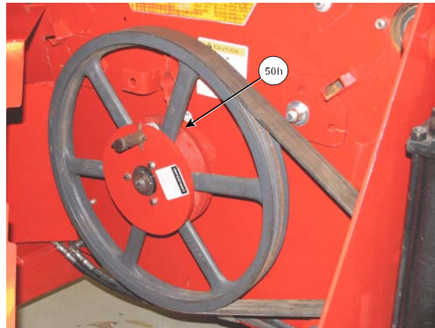
Grease Flail Drum Bearing
