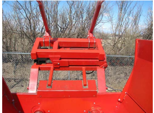
Rotate Forks to Closed Position Before Lowering 218151
