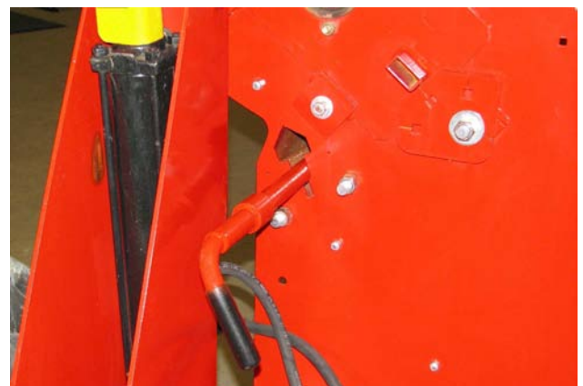
Replace Twine/Wrap Cutter Into Storage
