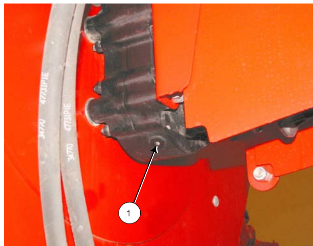
Drain Oil From Gearbox
