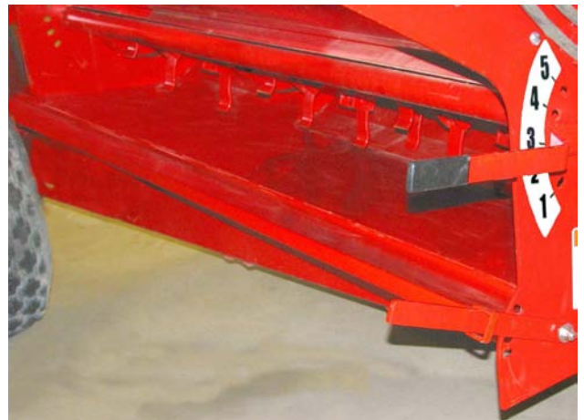
Set Level of Lower Discharge Deflector
