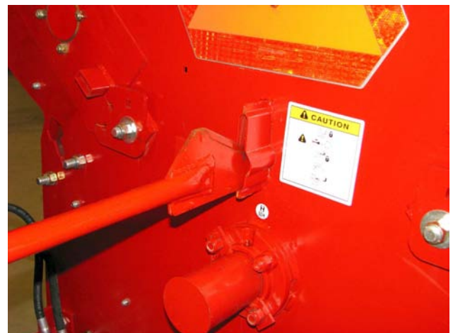
Insert Twine/Wrap Cutter with Blade Up
