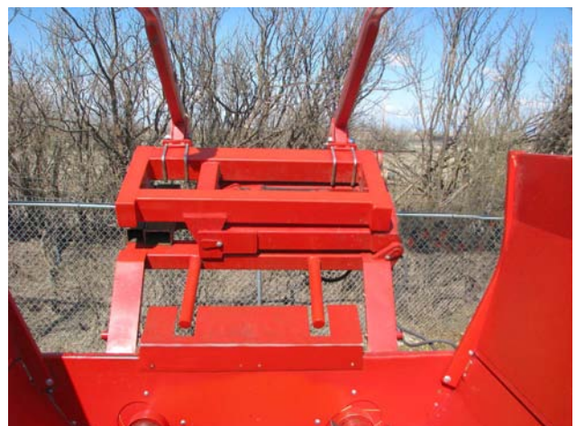
Rotate Forks to Closed Position Before Lowering
