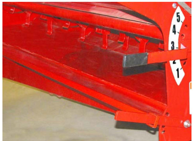
Re-Adjust Discharge Rate Lever (If needed)
