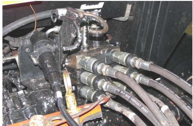
Disconnect Hydraulic Hoses & Electrical
