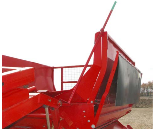
Fully Lower Forks - Indicator Rod
