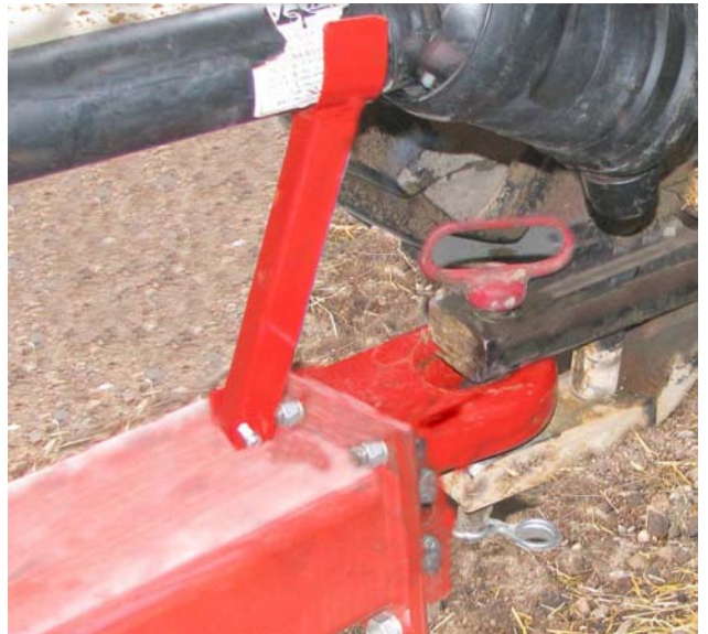
Connect Hitch to Tractor Clevis Drawbar
