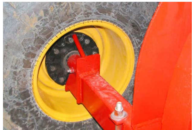
Remove Twine/Wrap from the Spindle and Hub
