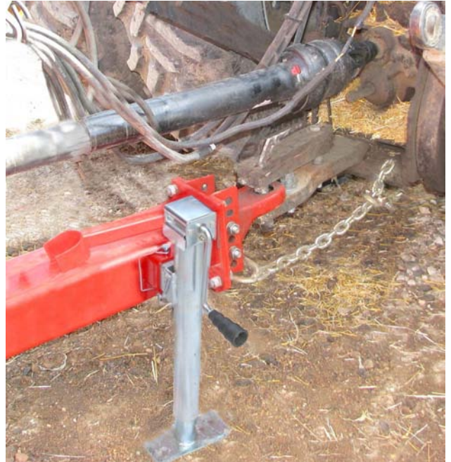
Jack on Hitch, Disconnect Driveline & Chain
