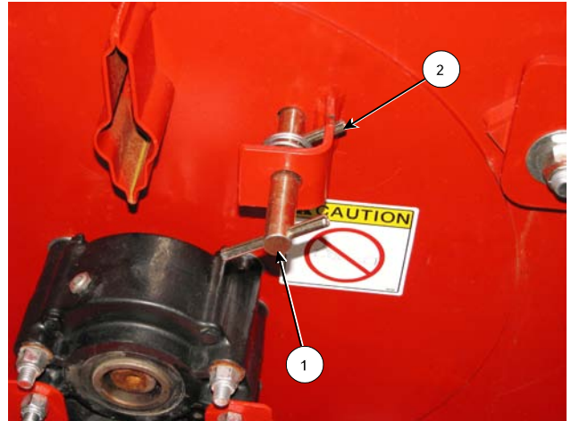
Remove the Flail Drum Lock
