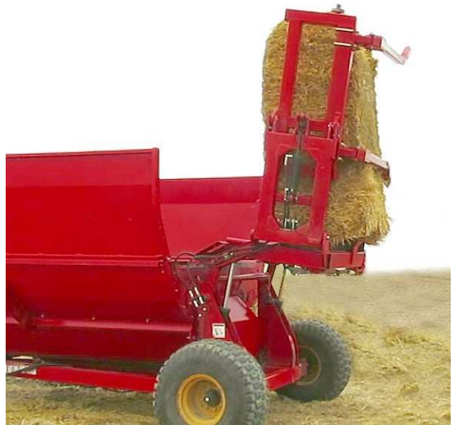
Stop the Feed Rollers Before Loading Bale
