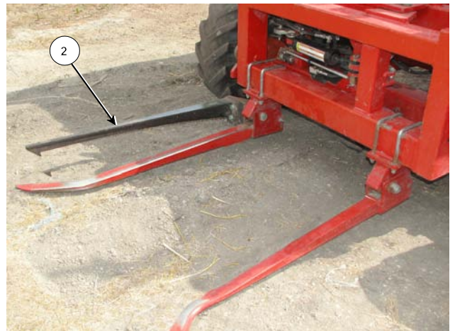
Spear on the Fork Breaks the Bale Twine
