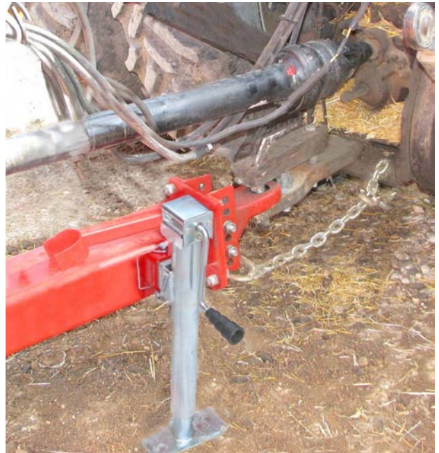
Adjust Height of Hitch Tongue
