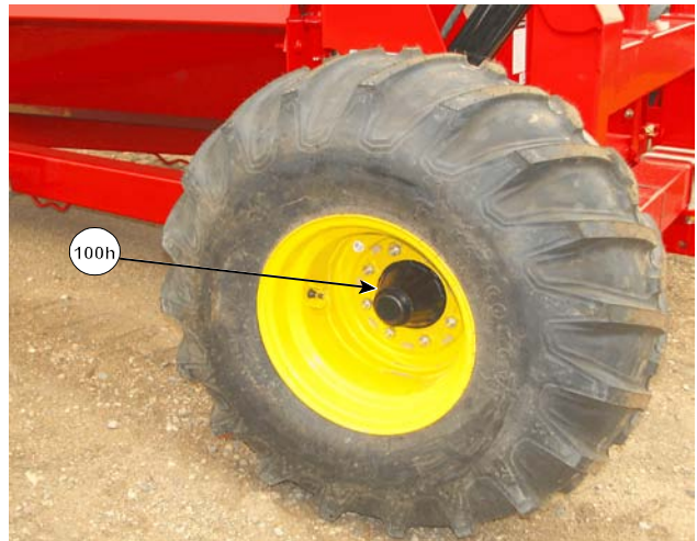
Grease Hubs on Both Spindles
