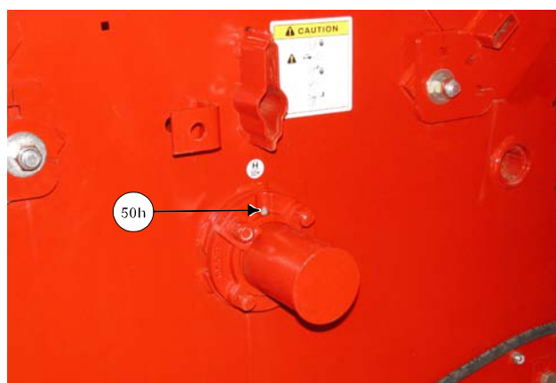
Grease Rear Flail Drum Bearing
