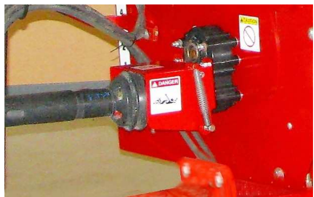
Ensure Driveline Shield is in Place
