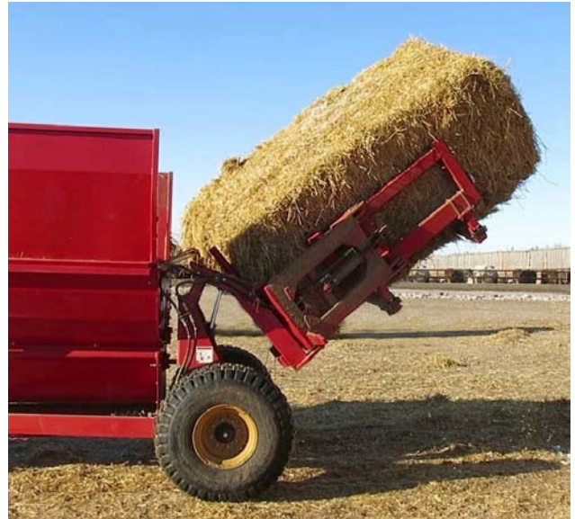
Long Side of Bale In Line With Tub Wall
