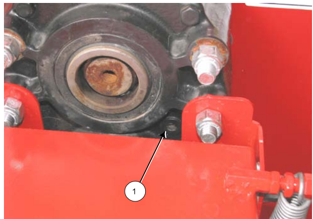
Check Gearbox Oil Level
