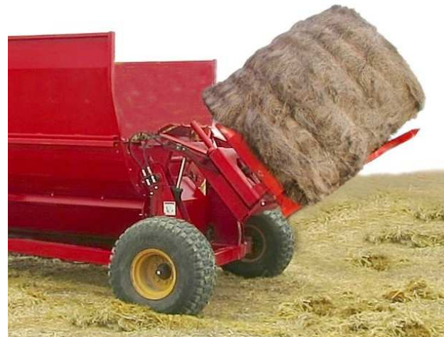
Raise the Bale into the Processor Tub
