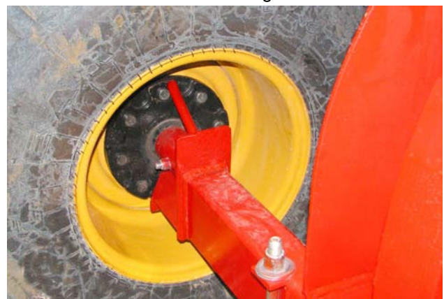
Remove Twine/wrap From the Spindle and Hub
