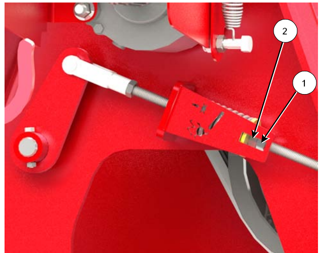
Loosen the Feed Chopper Belt Tension 219130C
