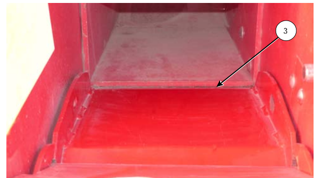
Ensure Door is Below Blower Exit
