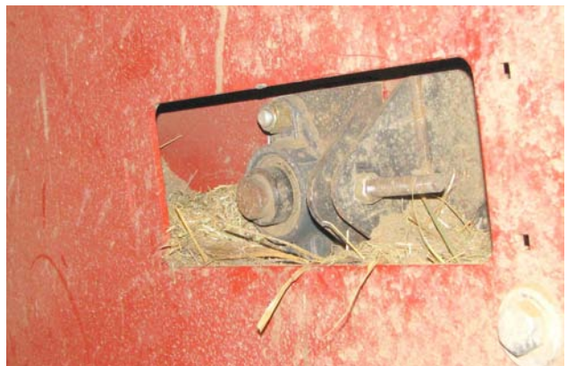
Remove Material - Upper Chain Bearing
