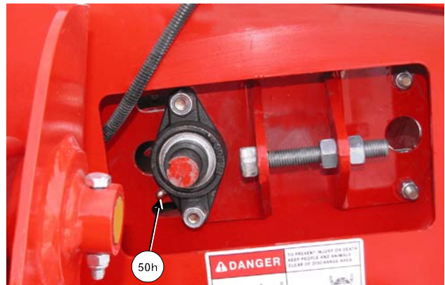
Grease Upper Feeder Chain Bearings
