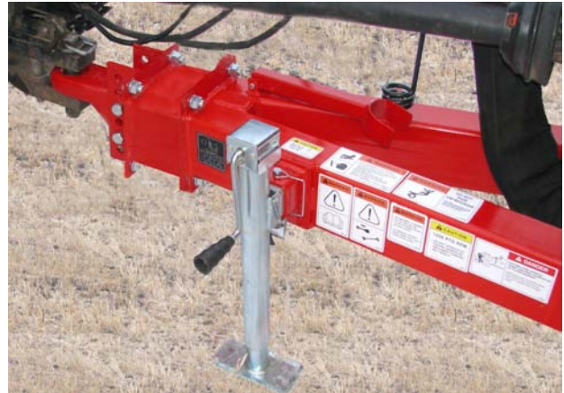
Jack on Hitch - Raise Hitch
