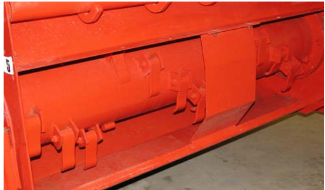
Clean Debris and Check Drum and Flails
