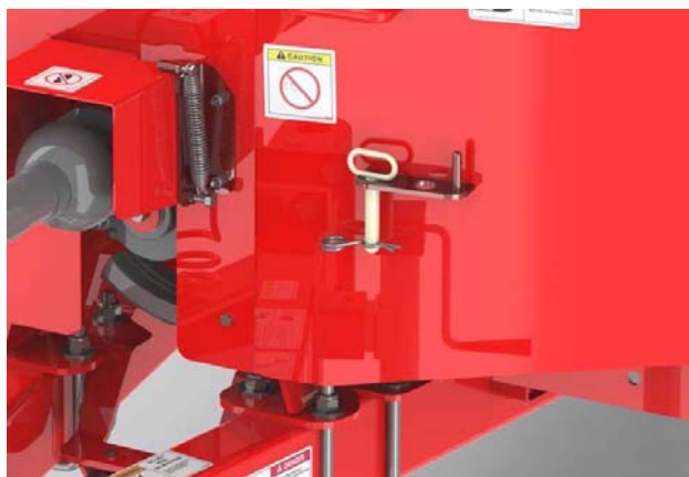
Store Lock Pin on Outside of Shield
