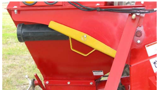
Cylinder Lock Stored (With Grain Tank) 212120
