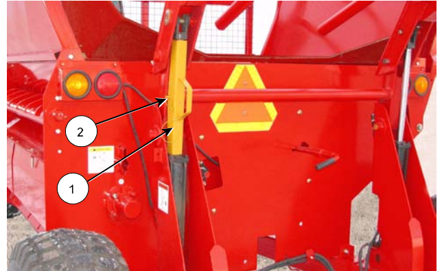
Fork Cylinder Resting on Lock
