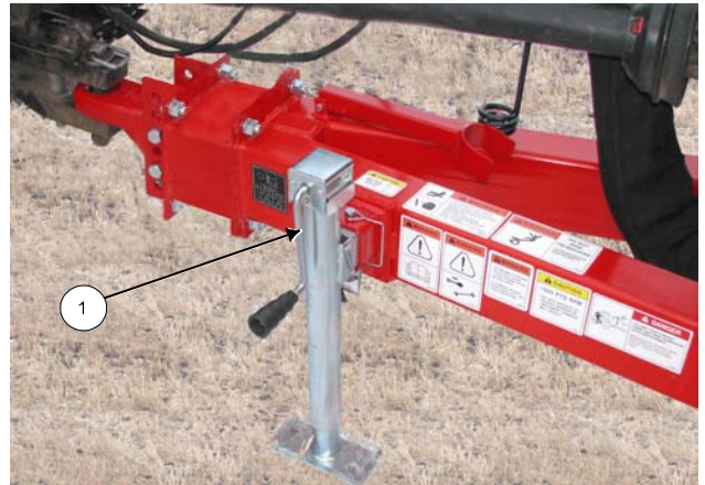
Lift Hitch with the Jack
