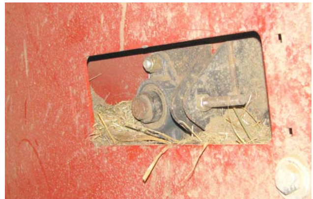
Remove Material - Upper Chain Bearing
