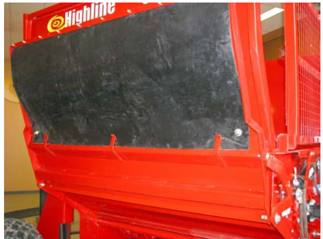
Raise Deflector Door to Transport Position
