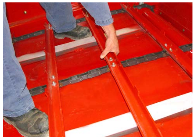
Check Tension of the Feeder Chain
