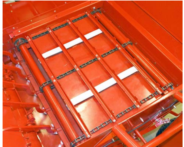
Check Condition of Feeder Chain
