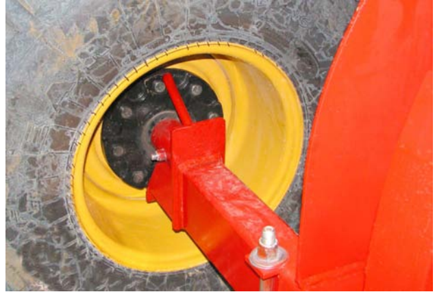
Remove Twine From the Spindle and Hub
