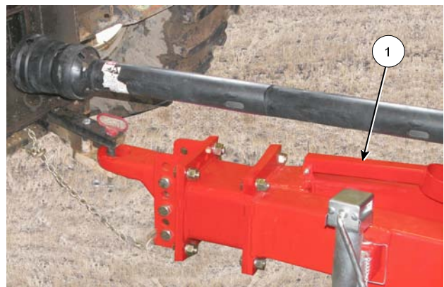
Connect Driveline to PTO
