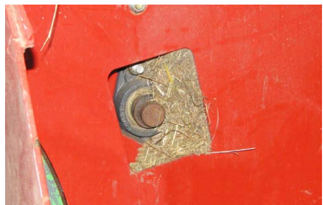
Remove Material - Lower Chain Bearing
