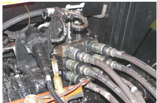
Disconnect Hydraulic Hoses & Electrical
