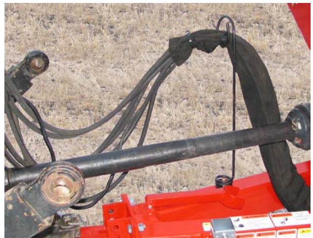
Hoses and Electrical in Support Arm
