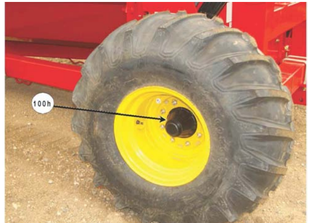
Grease Hubs on Both Spindles
