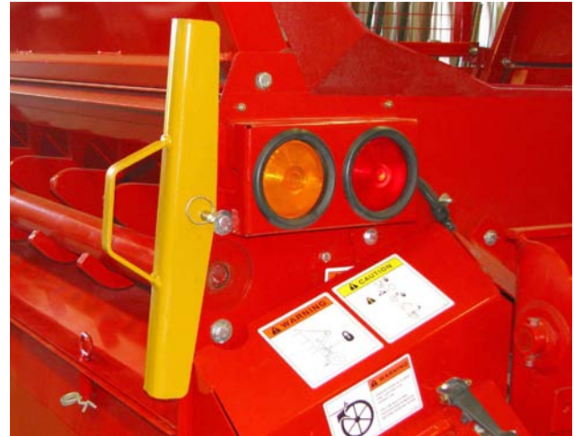
Cylinder Lock Stored (With Feedchopper) 212067
