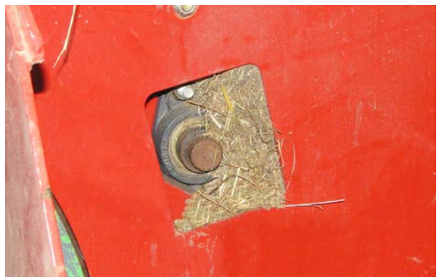
Remove Material - Lower Chain Bearing
