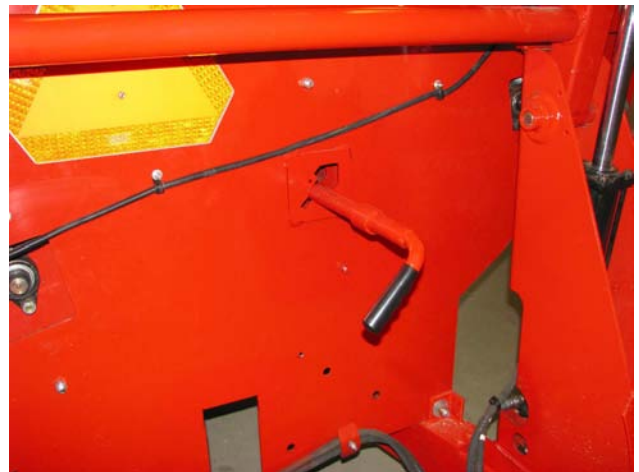
Remove Twine Cutter from Storage
