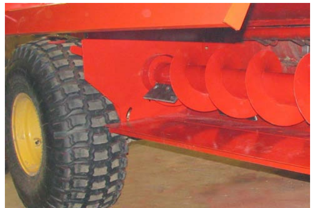
Remove Twine From Auger
