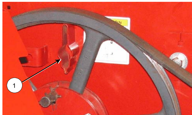
Align Sheave Spokes for Twine Cutter
