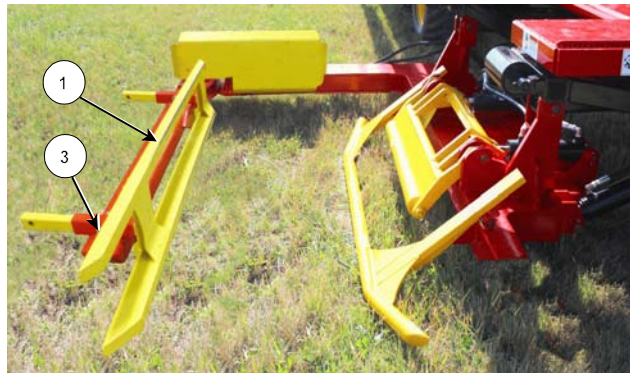
Adjust Arm for 4 Foot (1.2 m) Bales
