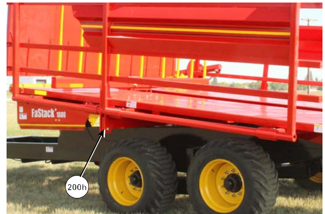
Grease the Side Rail Linkage
