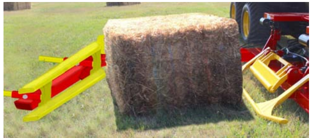
Drive Up to the Bale Until Arm is Around Bale
