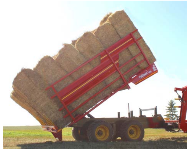
Raise Table, Let Bales Slide, Open Side Rails 217182
