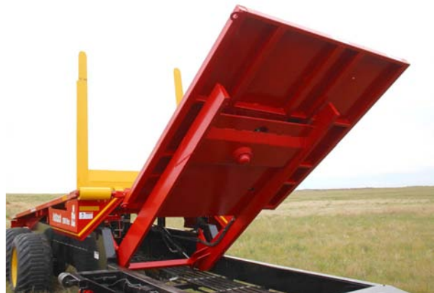
Check The Front Table Raises and Lowers (1200 Flex Shown)
