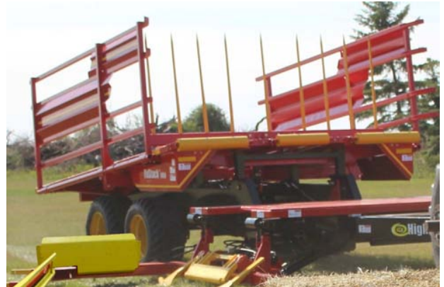
Lower Front Table ,Lower Lift Arm
