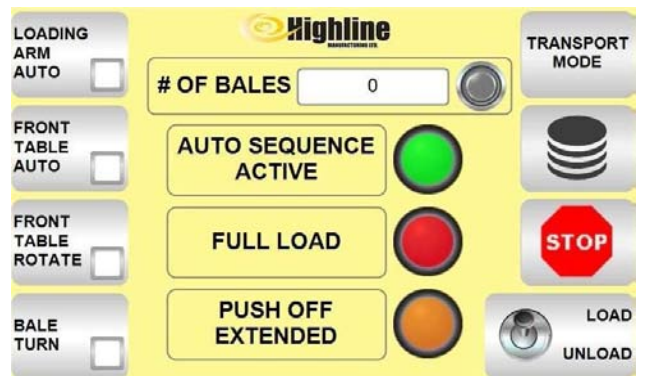
Turn on the Load Function
