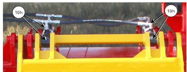
Grease the Bale Turn Cylinders
