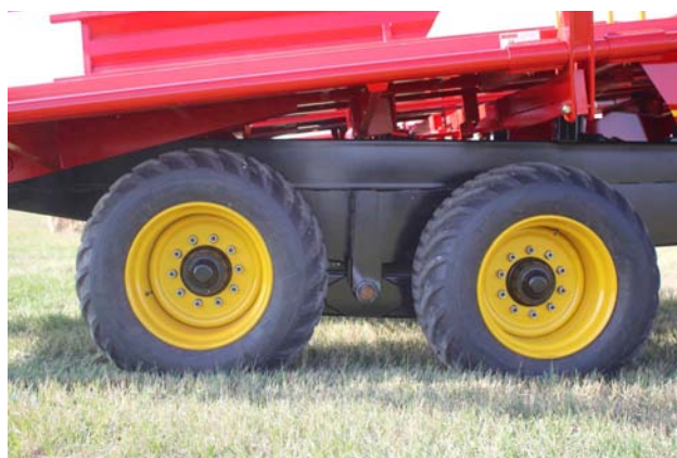
Jack Under Spindle Tube to Change Tire
