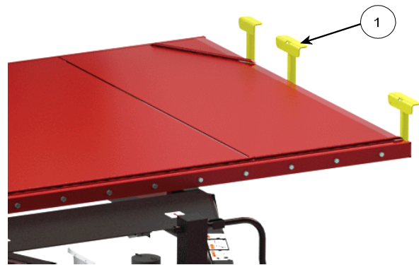
Adjust Front Table Stops
