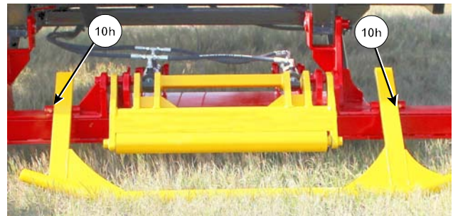
Grease the Bale Support Arm Pivots
