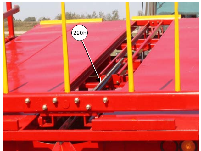
Lubricate the Trolley Chain
