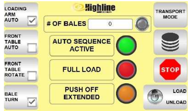
Enable Loading Arm Auto
