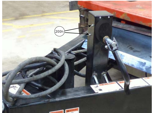
Grease the Hitch Jack
