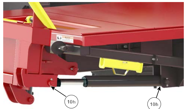
Grease Both Main Lift Arm Cylinders
