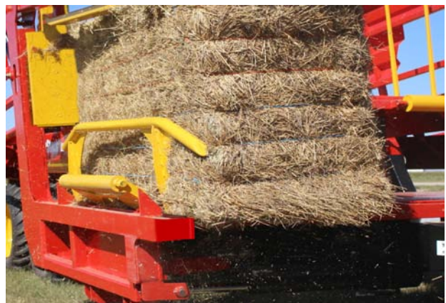
Raise the Lift Arm to Place Bale on the Table
