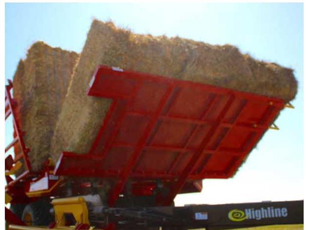
Press Front Table Up - Raise Front Table
