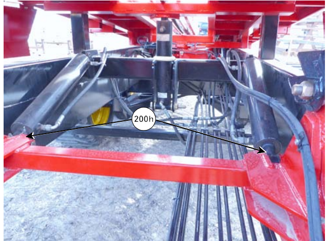
Grease Front Table Cylinders
