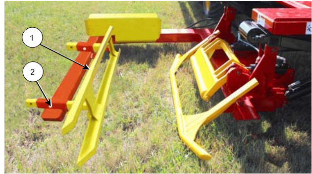
Adjust Arm for 3 Foot (0.9 m) Bales
