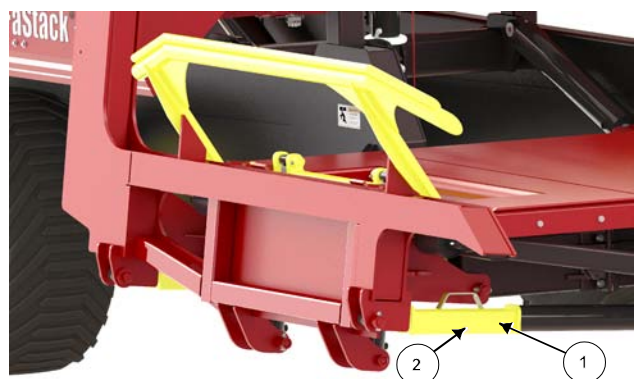
Install the Front Lift Arm Transport Lock
