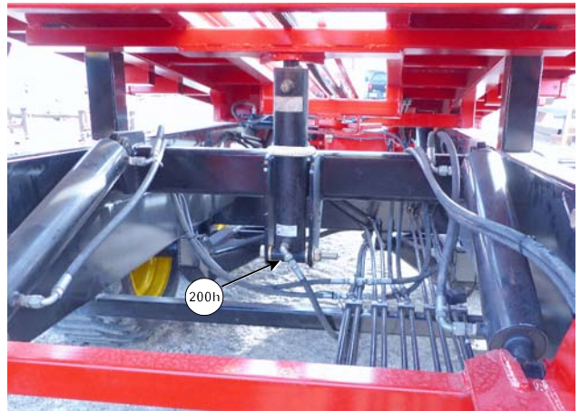
Grease the Rear Table Boost Cylinder
