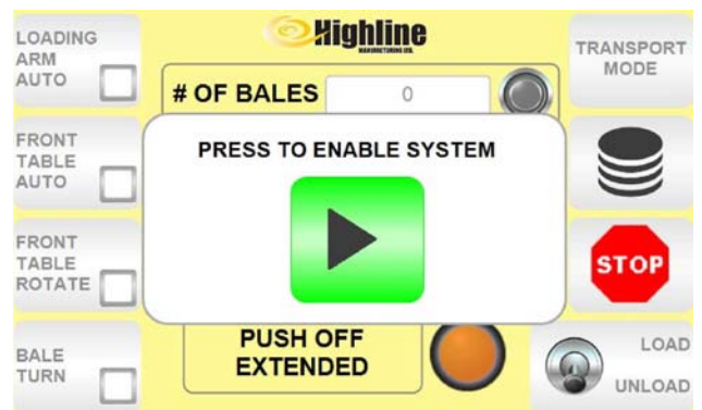
Reactivate System after Pushing Stop
