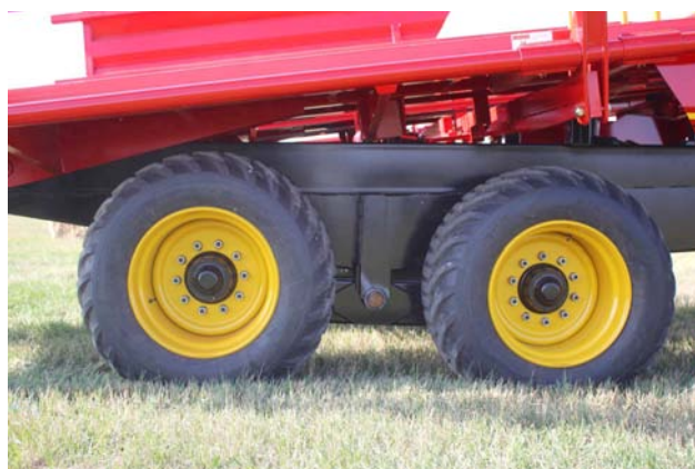
Jack Under Spindle Tube to Change Tire
