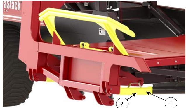
Remove the Front Lift Arm Transport Lock
