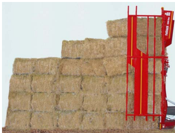
1200 Flex Rotated Bales - Create Staircase for Stability 218076C
