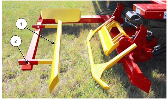
Adjust Arm for 3 Foot (0.9 m) Bales
