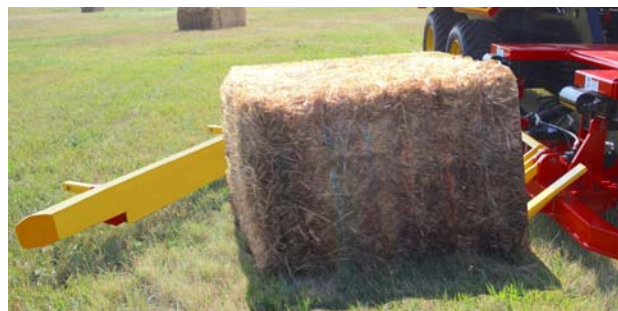
Drive Up to the Bale Until Arm is Around Bale 219039
