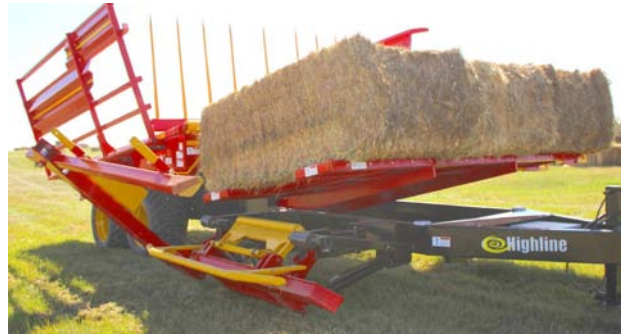
Lower Arm Before Lifting Front Table
