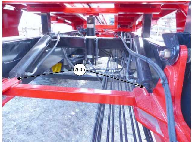
Grease Front Table Cylinders
