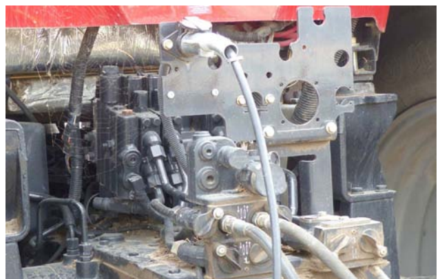
Disconnect Hydraulics and Lighting Cable
