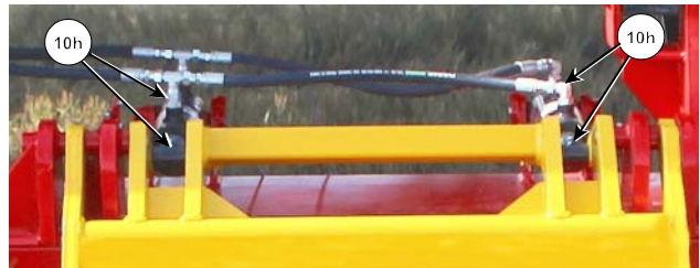
Grease the Bale Turn Cylinders
