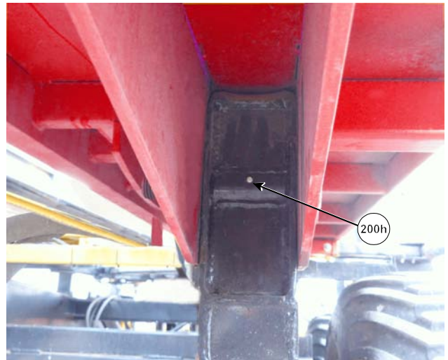
Grease Rear Table Pivots (Right Side Shown)
