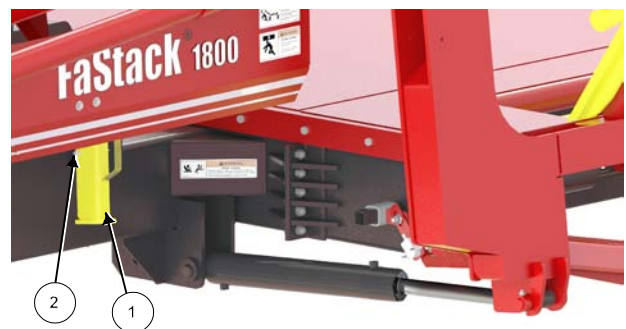
Remove Front Lock, Place In Storage
