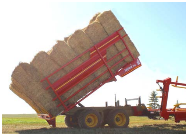
Raise Table, Let Bales Slide, Open Side Rails 217182
