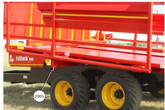
Grease the Side Rail Linkage
