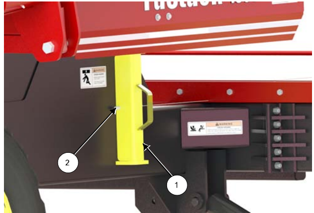
Remove Rear Lift Arm Lock from Storage
