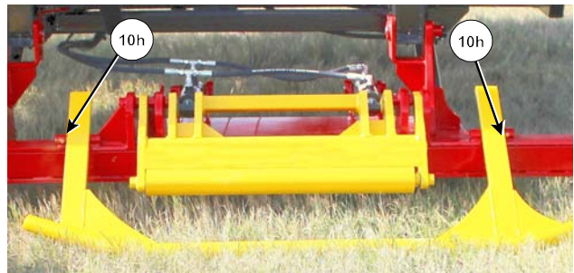
Grease the Bale Support Arm Pivots
