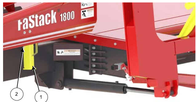
Remove Rear Lock, Place In Storage
