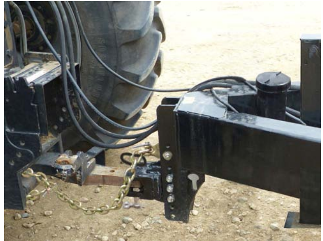
Adjust Clevis. Connect Hitch and Safety Chain 219033
