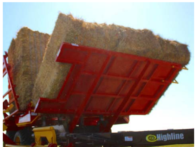
Press Front Table Up - Raise Front Table
