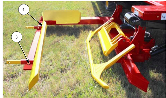
Adjust Arm for 4 Foot (1.2 m) Bales
