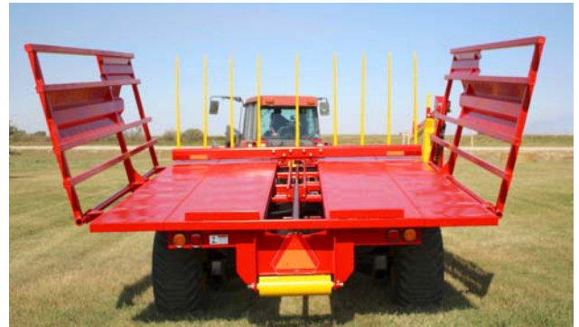
Check that the Side Racks Open and Close
