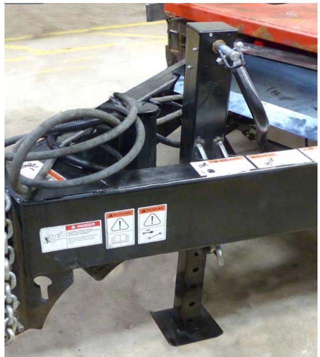
Lower the Hitch Jack to Support the Weight
