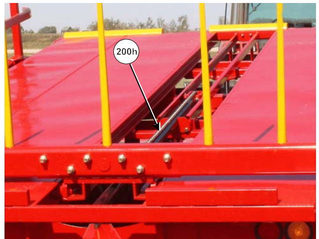
Lubricate the Trolley Chain
