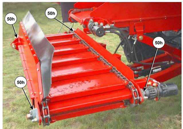
Front Right/Left Conveyor Bearings
