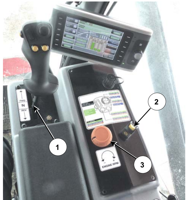
Joystick to Neutral, Park Brake On, Throttle Low Speed
