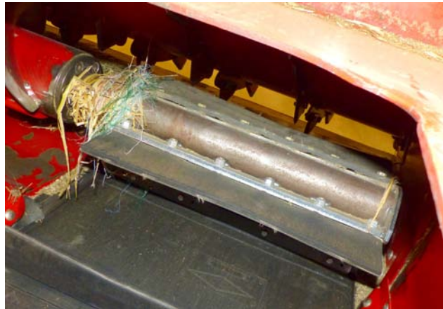
Check the Auger and Loading Paddles. Remove Twine/Wrap Buildup
