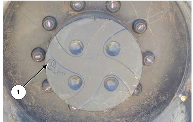
Check Oil Level with Drain Plug Horizontal
