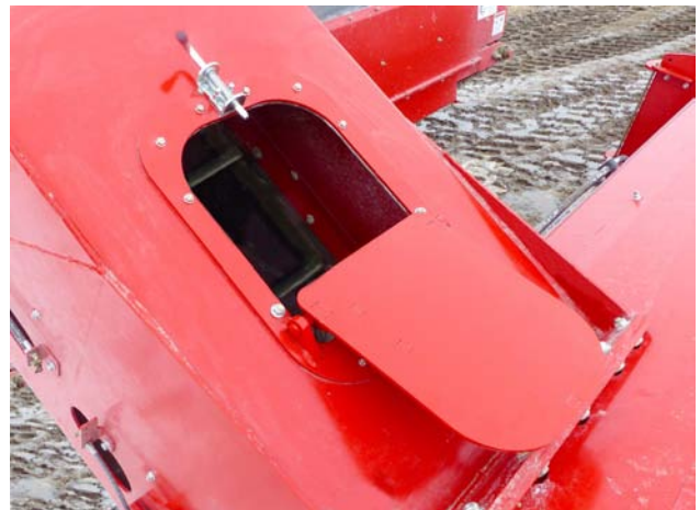
Lift Mineral Loading Door for Access to Auger and Loading Paddles
