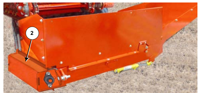
Clean the Conveyor Spill Guard. Use the Joystick Buttons to Raise/Lower the High Bunk Section of the Front Conveyor
