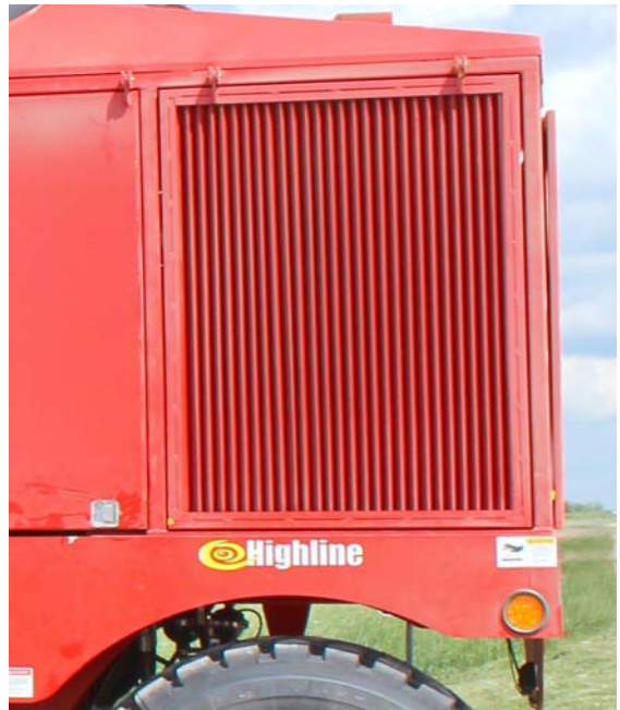
Clean Outer Engine Cooler Screen
