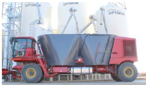
Loading From Overhead Augers
