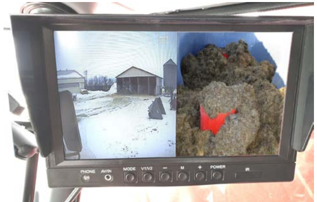
Check Tub Camera for Material Landing Near the Center of Tub 220073
