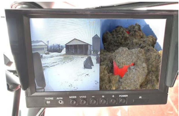
Check Tub Camera for Material Landing Near the Center of Tub
