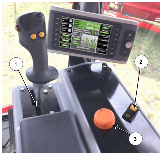
Park Brake On, Joystick to Neutral, Throttle Low Speed 219206C
