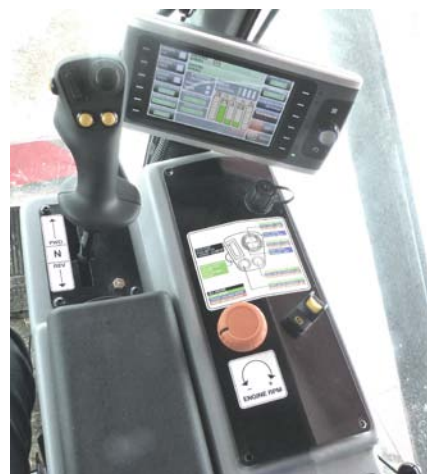
Move Joystick for Direction & Speed of Travel
