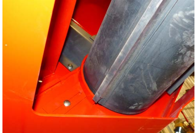
Check Condition of the Loading Arm Belt
