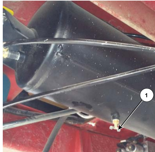
Check For Moisture by Opening Air Tank Drain Valve 222012C
