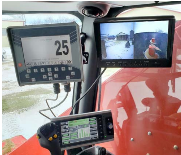
Check the Weigh Scale Monitor Is Working
