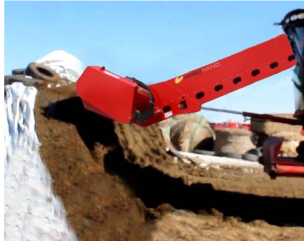
Raise Milling Arm to Top of Pile
