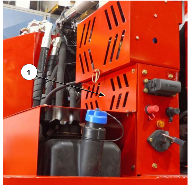
Remove Panel for 24 Volt High Current Fuses 219390C3
