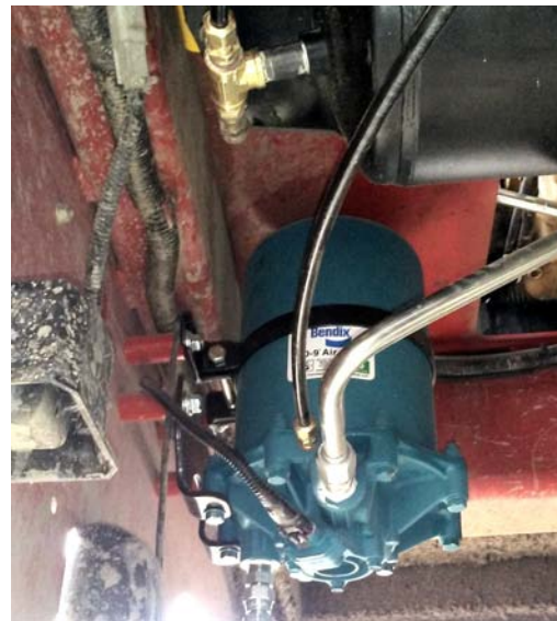
Compressed Air Dryer Check for Oil from Exhaust 222011
