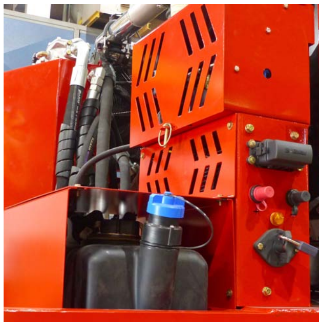
Check DEF Tank Level and Add If Needed
