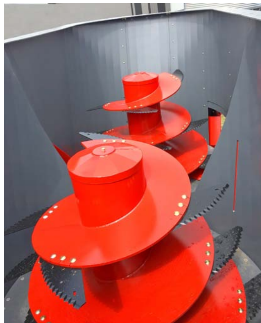
Check for Build Up in the Tub and Condition of the Screws (Optional Knives Shown)
