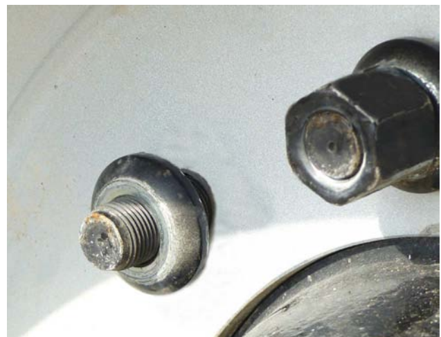
Flat of Washer Against Rim, Torque the Nuts
