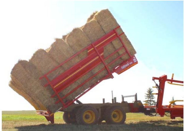
Raise Table, Let Bales Slide, Open Side Rails 217182
