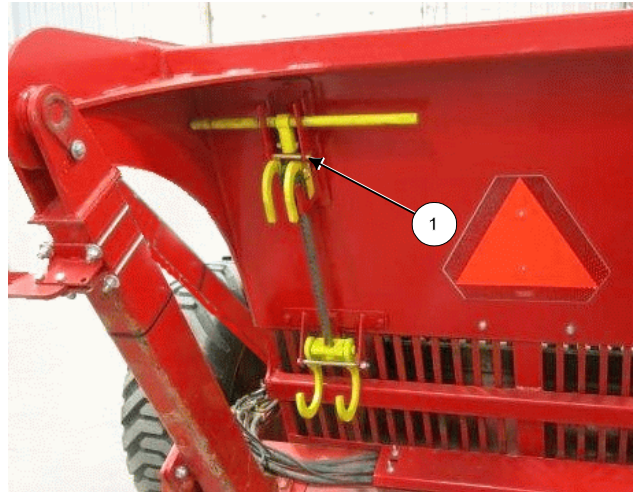
Compressor Tool in Storage Location
