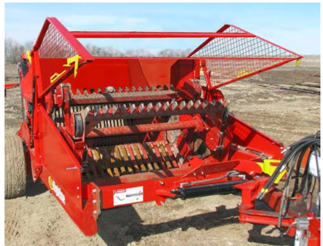
Unlock and Lift the Reel Cage
