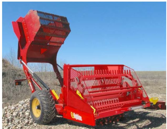
Rock Bucket in Dumping Position
