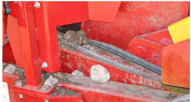
Remove Rocks from the Frame - Left Side
