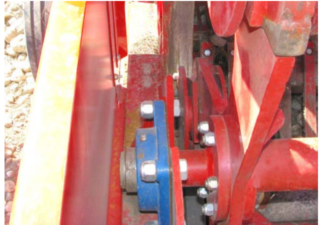
Lubricate Both Reel Bearings (Right Shown)
