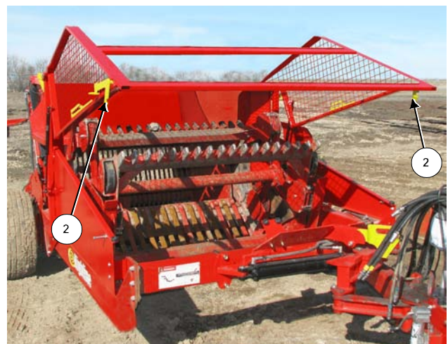
Unlock and Lift Reel Cage
