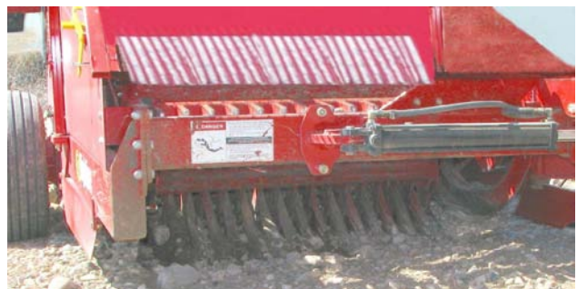
Reverse Reel & Raise Apron to Remove Rock
