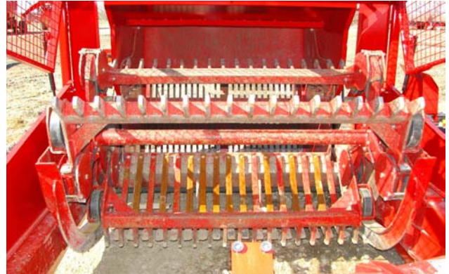
Check Condition of Reel, Apron and Bucket
