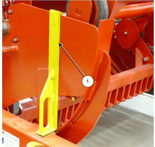
Install Apron Lock - Right Side (Reel Access Panel Shown Open)
