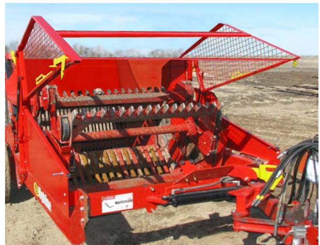
Unlock and Lift the Reel Cage
