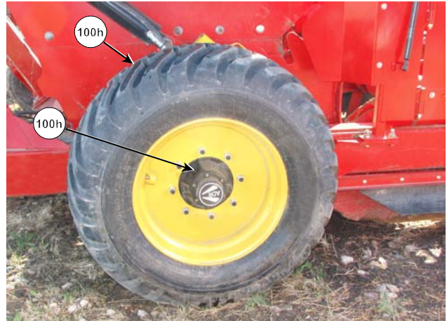
Grease Wheel Hubs
