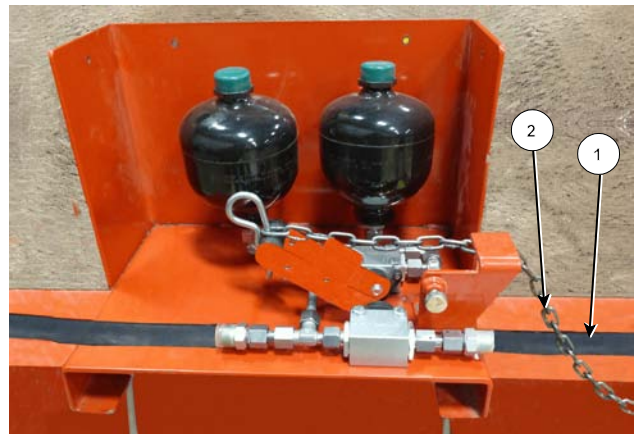
Connect Breakaway Chain to the Tractor (Guard Removed for Clarity)
