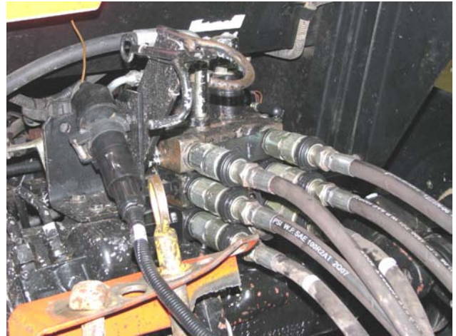
Connect Hydraulic Hoses & Electrical
