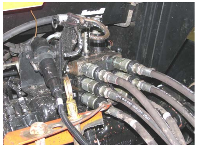
Disconnect Hydraulic Hoses & Electrical
