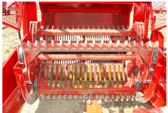
Tighten Upper and Lower Tine Bolts
