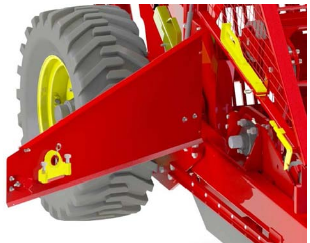
Remove Rocks from the Frame - Right Side
