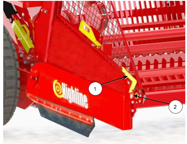
Close Panel, Lower and Lock the Reel Cage
