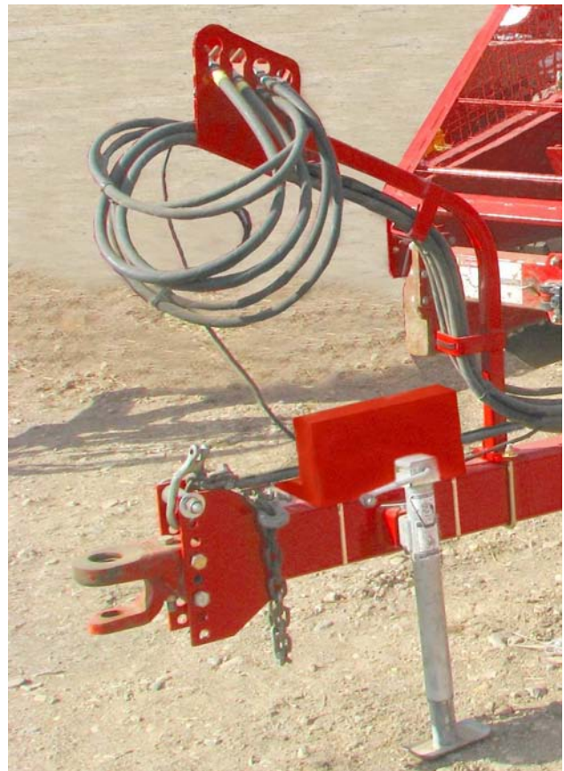
Disconnect Safety Chain and Hitch
