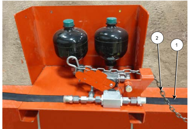
Disconnect Breakaway from the Tractor (Guard Removed for Clarity)
