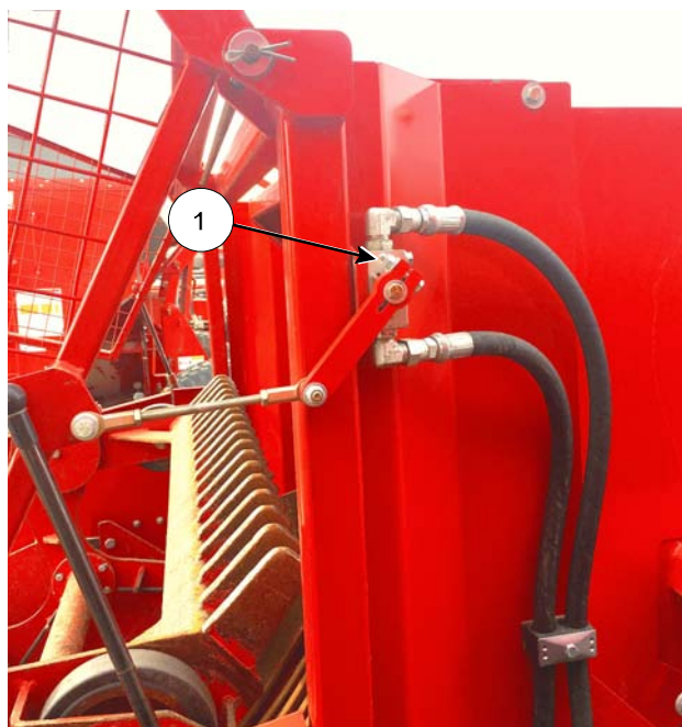
Reel Hydraulic Lockout Valve
