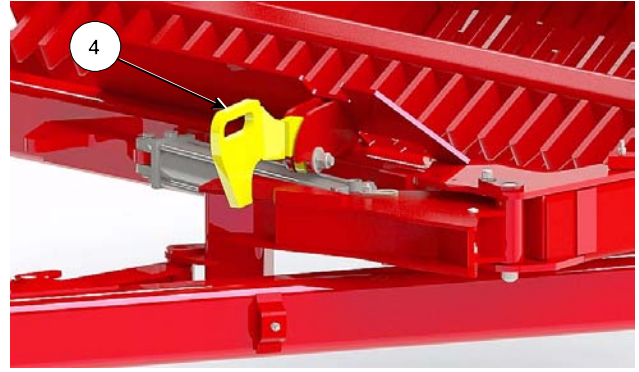
Engage Hitch Transport Lock
