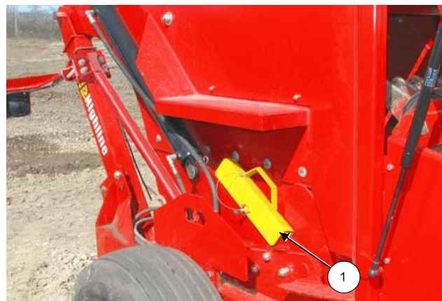
Bucket Lock in Storage Position
