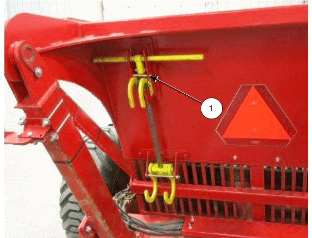
Compressor Tool in Storage Location
