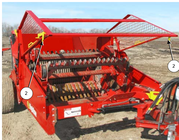
Unlock and Lift Reel Cage
