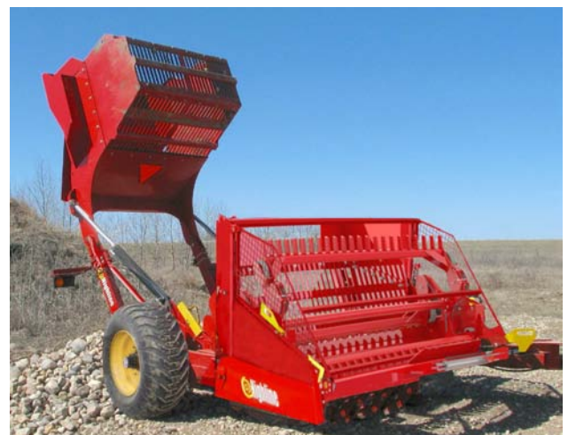
Rock Bucket in Dumping Position
