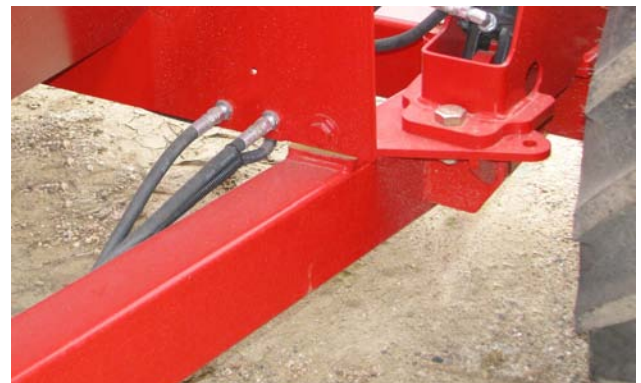
Bale Lift Hoses Connected to Bulkhead Fittings
