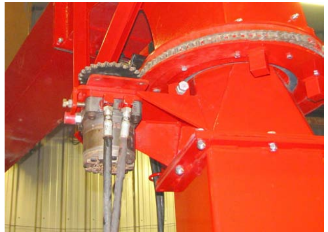
Connect Hoses to the Motor
