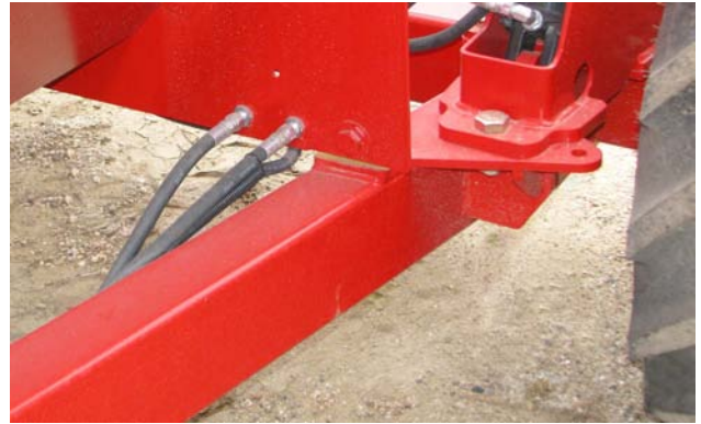
Disconnect Bale Lift Hoses
