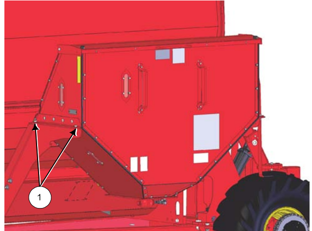
Lower the Tank and Attach to Support Brackets 216152C
