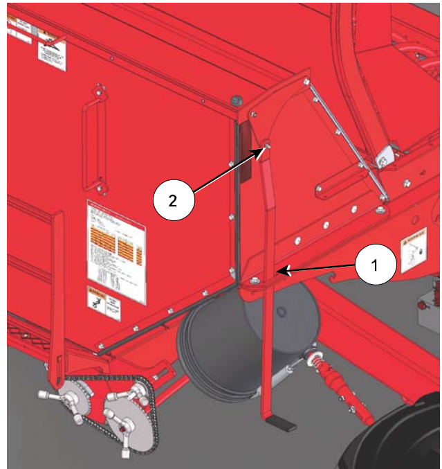
Attach the Tank Lid Handle
