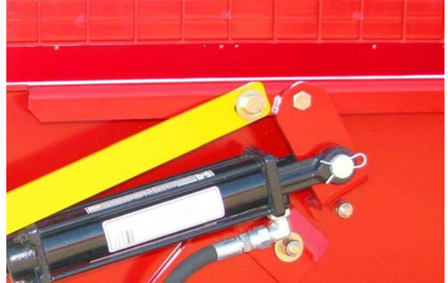
Install Cylinder Bracket & Lock Strap
