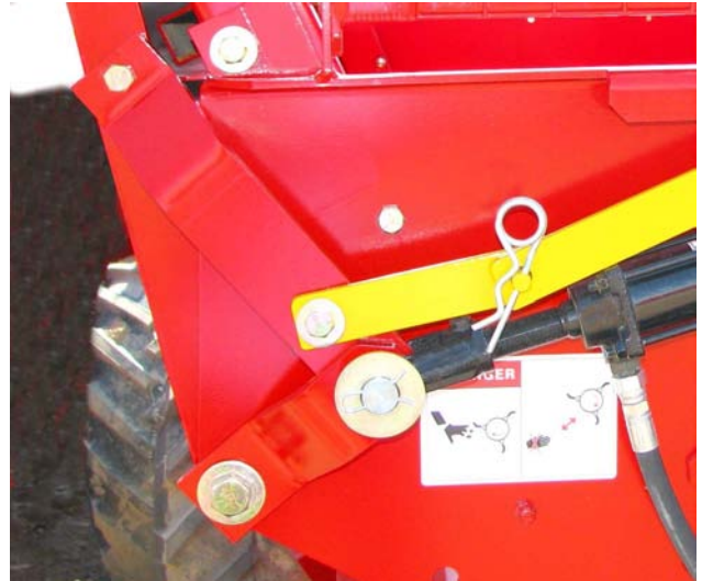
Install the Lock Strap and Door Lug
