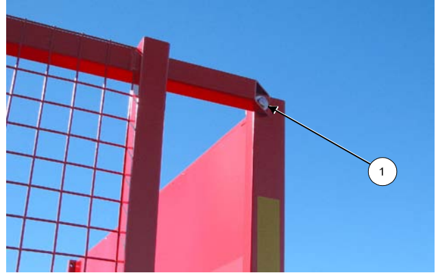
Remove Fasteners From Screen to Tub Wall 215090C
