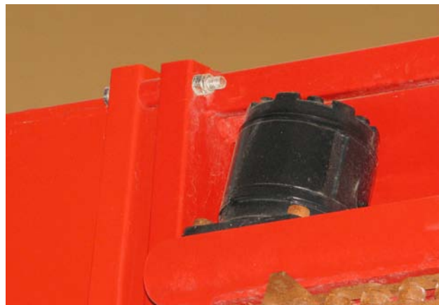
Remove Fastener and Spacer Between Walls 215101
