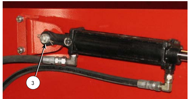
Connect Base of Cylinder to the Mount
