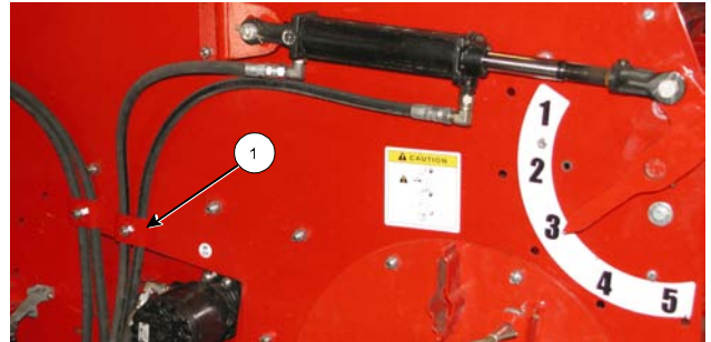
Fasten Hoses with the Hose Clamp
