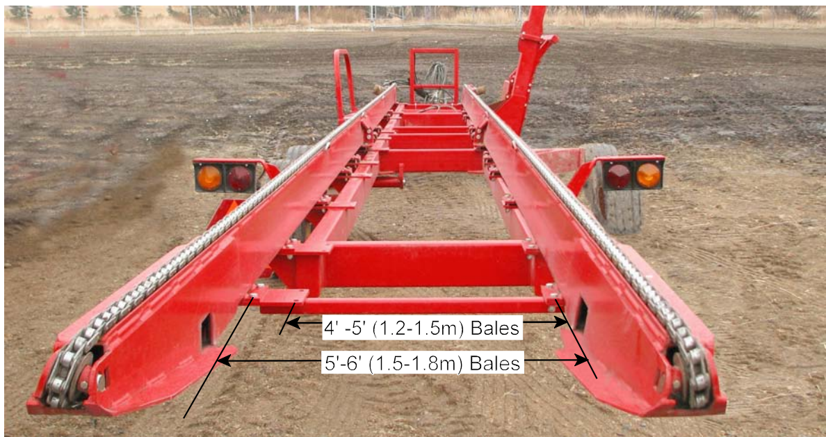
Suggested Rail Positions for Size of Bale. Adjust for Condition of Bale
