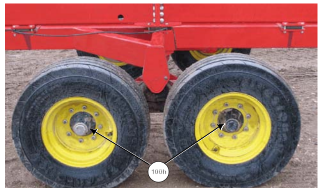
Grease Hubs on all Spindles
