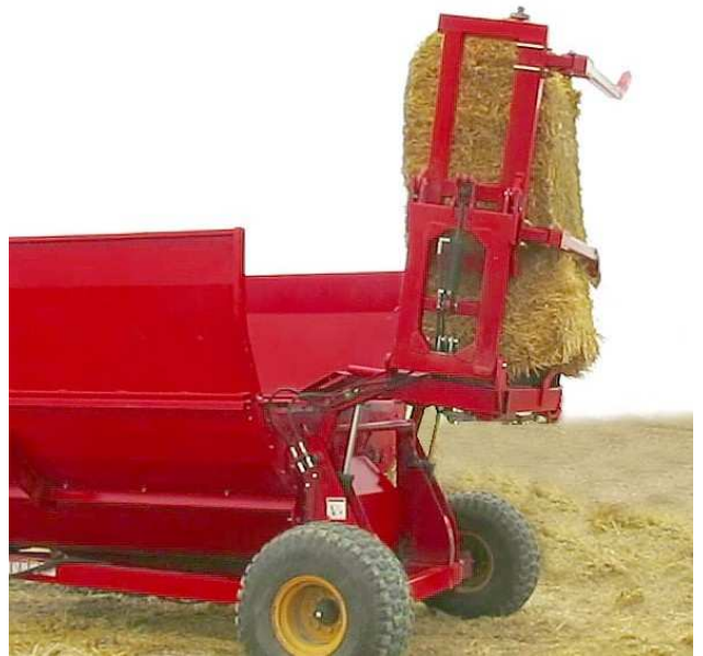
Stop the Feed Rollers Before Loading Bale
