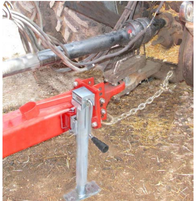
Adjust Height of Hitch Tongue
