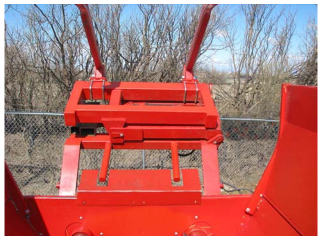
Rotate Forks to Closed Position Before Lowering
