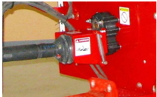
Ensure Driveline Shield is in Place
