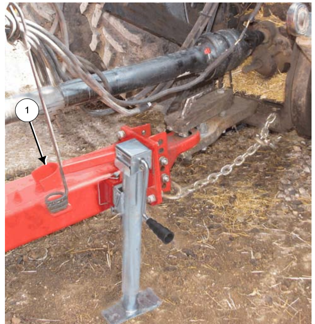
Connect Driveline to PTO
