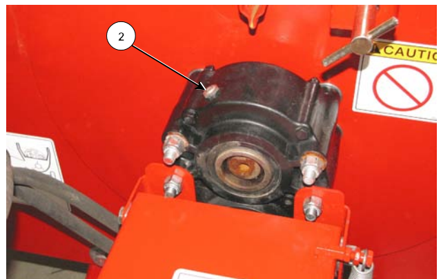
Add Oil at Top of Gearbox
