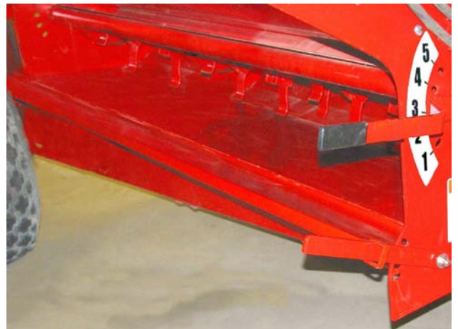
Set Level of Lower Discharge Deflector
