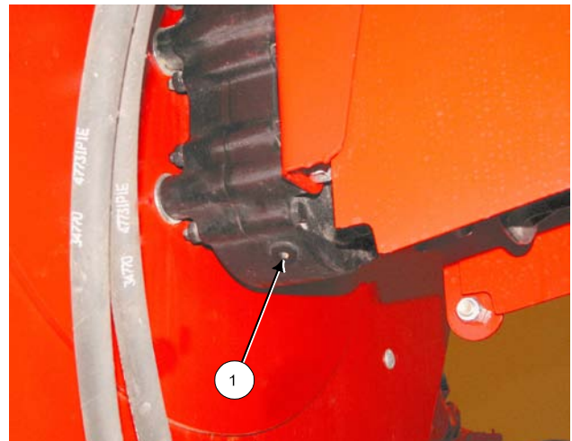
Drain Oil From Gearbox
