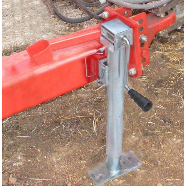
Lift Hitch with the Jack
