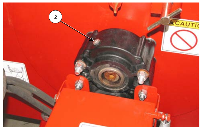
Add Oil at Top of Gearbox
