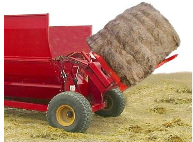
Raise the Bale into the Processor Tub
