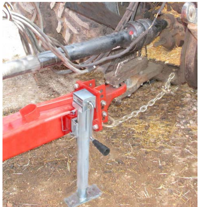
Jack on Hitch, Disconnect Driveline & Chain
