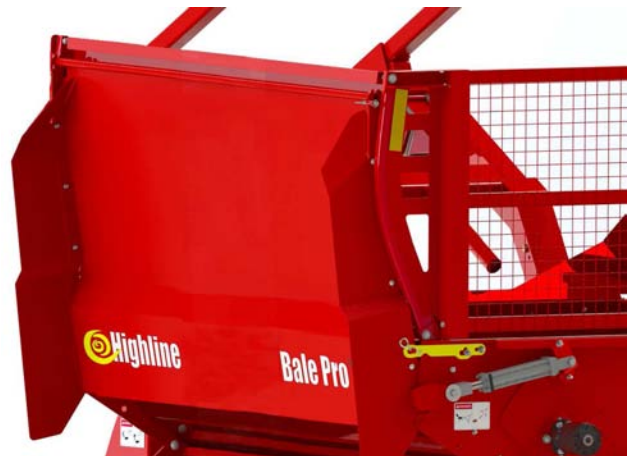
Discharge Door Raised - Rubber Secured
