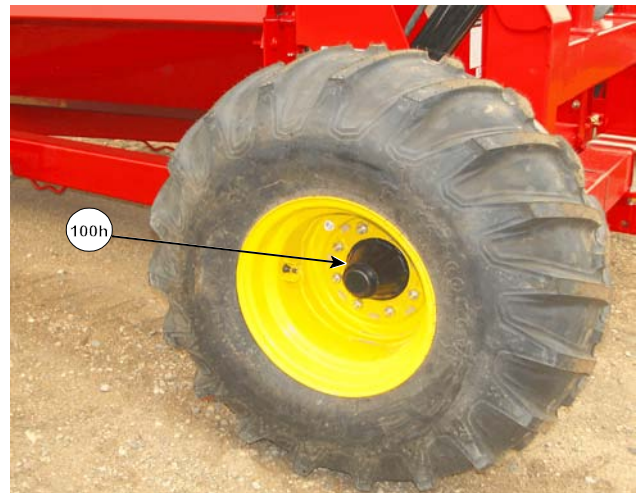
Grease Hubs on Both Spindles
