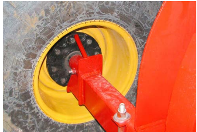
Remove Twine from the Spindle and Hub
