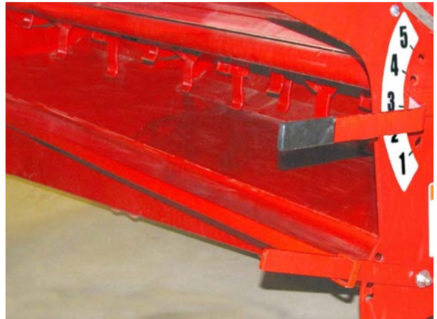
Re-Adjust Discharge Rate Lever (If needed)
