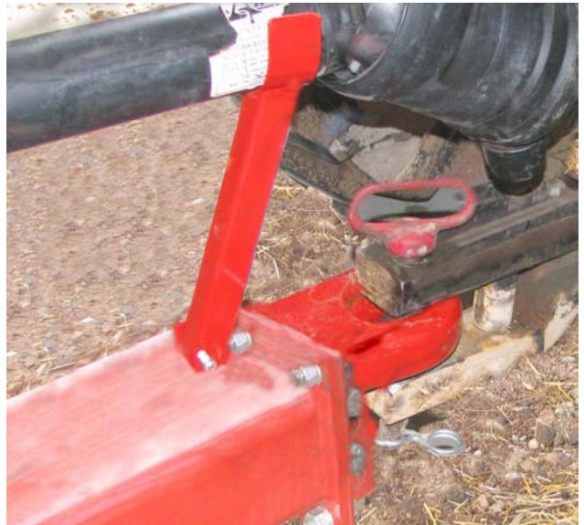
Connect Hitch to Tractor Clevis Drawbar
