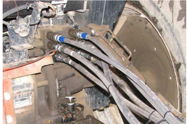
Disconnect Hydraulic Hoses
