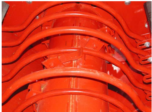
Move Flails Blocking the Knife Path
