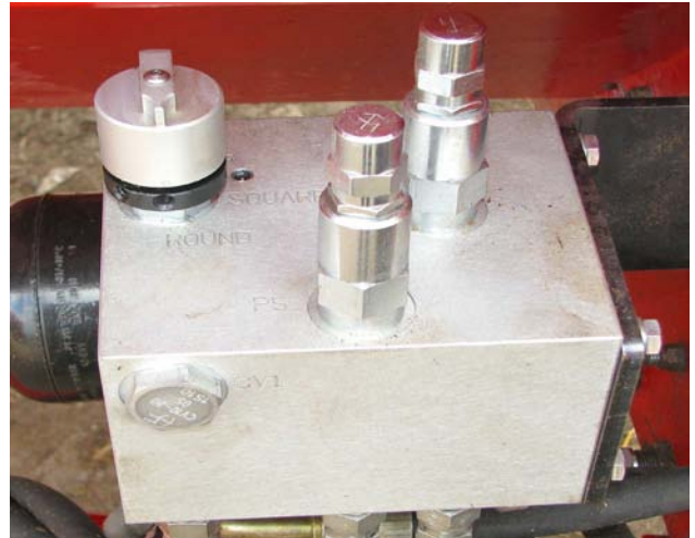
Select “Round” on 2 Valve Hydraulic Block
