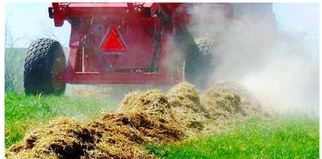
Door Lowered for Windrow Feeding
