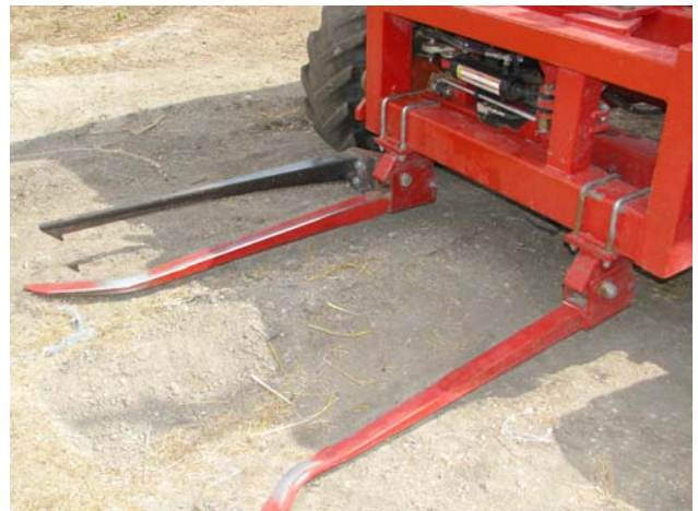
Forks Lowered and in the "Home" Position
