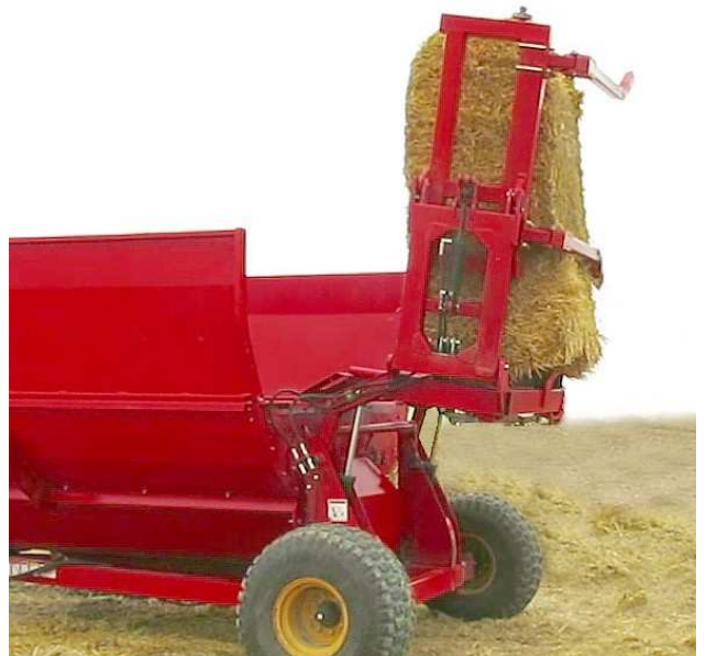
Stop the Feed Rollers Before Loading Bale
