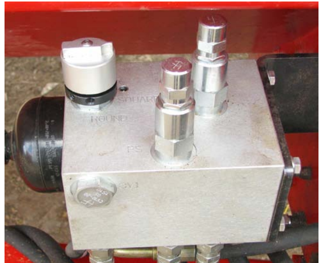
Select "Square" on 2 Valve Hydraulic Block
