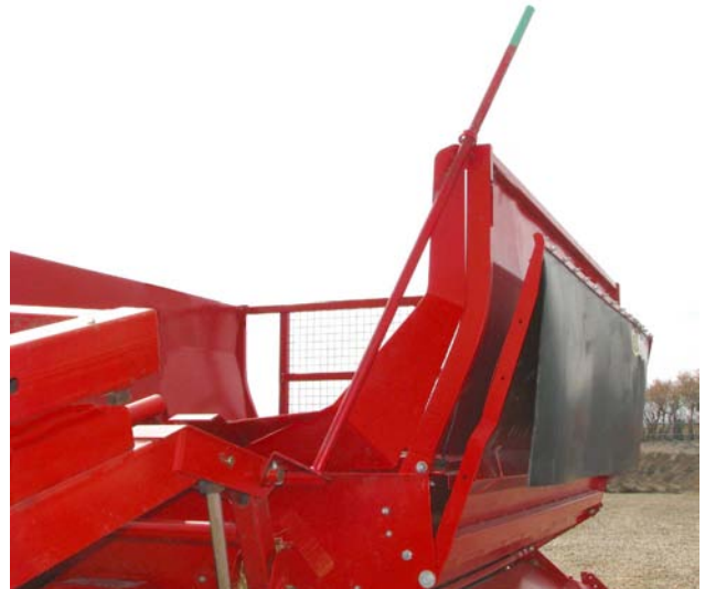
Fully Lower Forks - Indicator Rod
