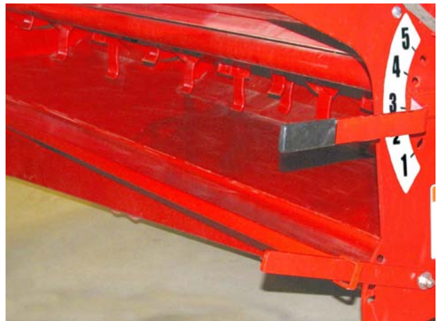
Re-Adjust Discharge Rate Lever (If needed)
