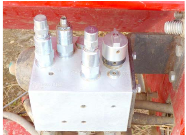
Select “RD” on 3 Valve Hydraulic Block
