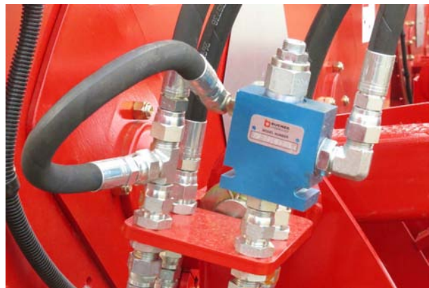
Lift Pressure Sequence Valve on Fork Pivot
