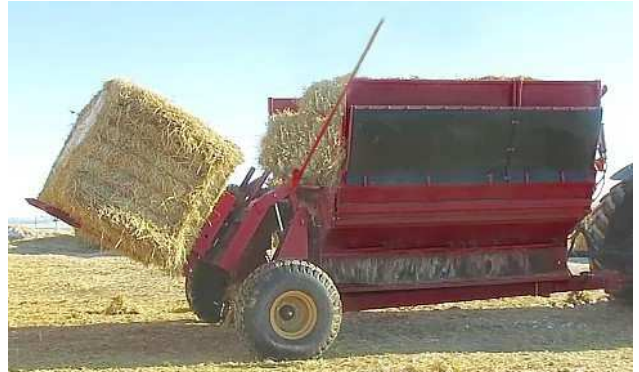
Second Bale On Forks - Non Rotated Position 214093
