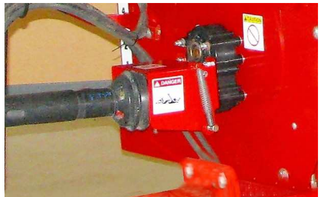
Ensure Driveline Shield is in Place
