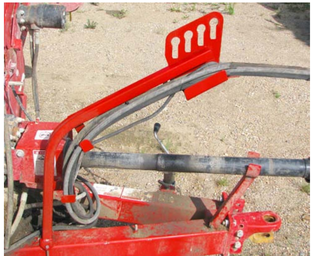
Hoses and Electrical in Support Arm
