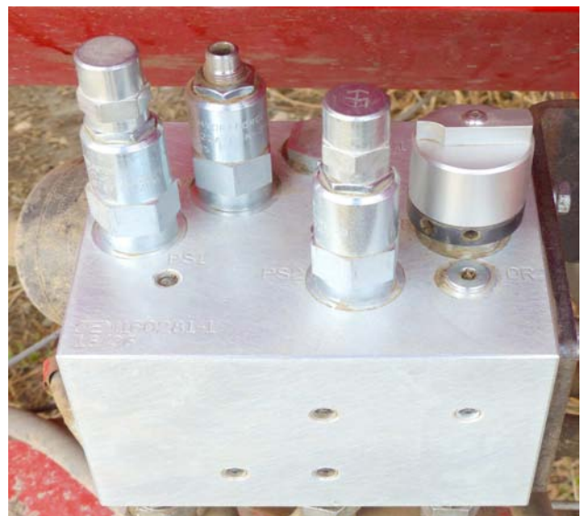
Select "SQ" on 3 Valve Hydraulic Block
