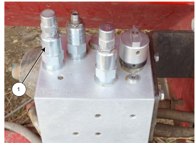
Adjust "PS1" For Rotation When Lowering
