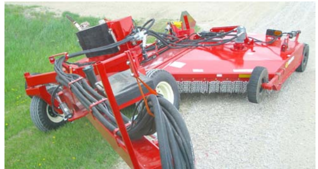
Swing Deck Into Cutting Area
