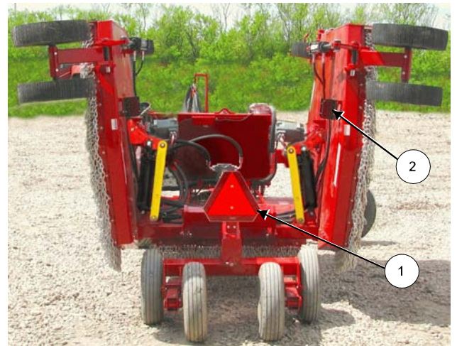
Ensure SMV is Visible & Lights are Working
