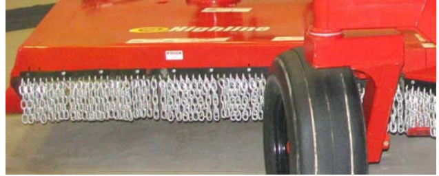
Check Condition of the Chain Guards
