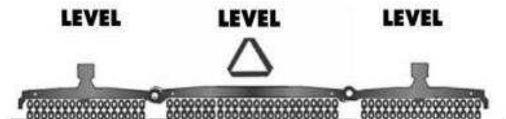
Level Ground Wing Adjustment - From Behind
