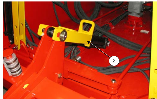
Height Cylinder Resting on Transport Lock
