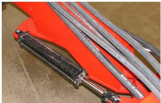
Remove Hitch Cylinder Locks
