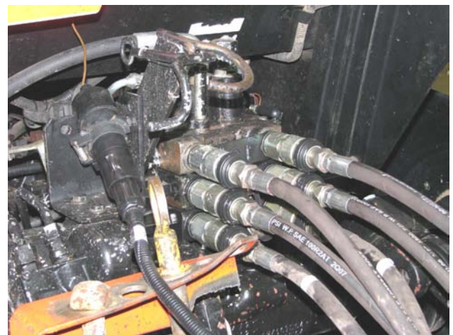
Disconnect Hydraulic Hoses & Electrical
