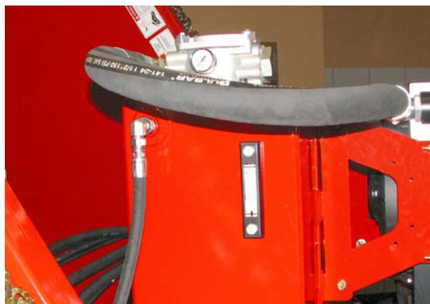
Check Oil Level After Filling
