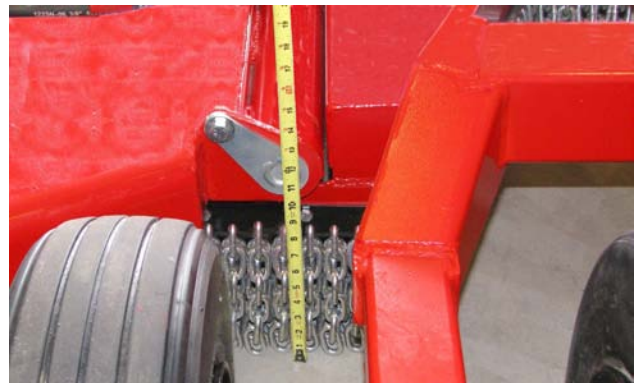
Height from Back Wing Pivot to Ground
