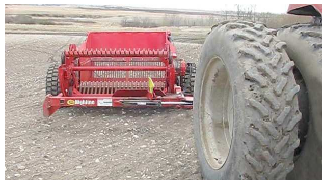
Rockpicker In Working Position
