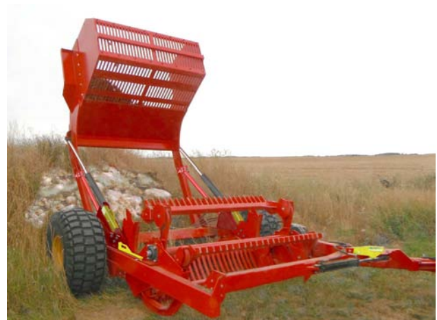
Rock Bucket in Dumping Position
