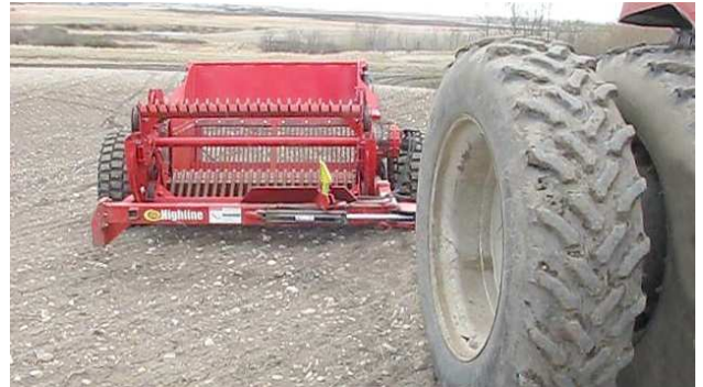
Hitch Position 1 - Dual Tractor Tires
