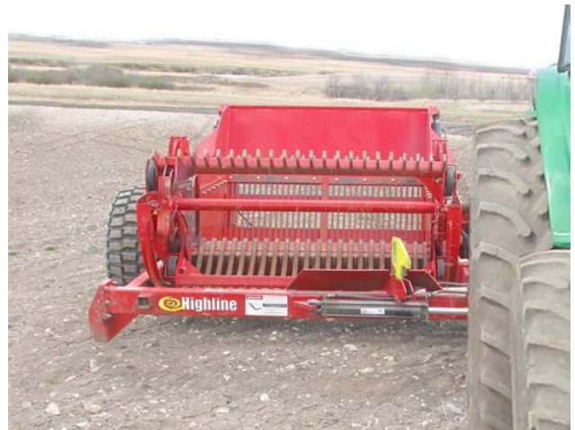
Hitch Position 2 - Single Tractor Tires
