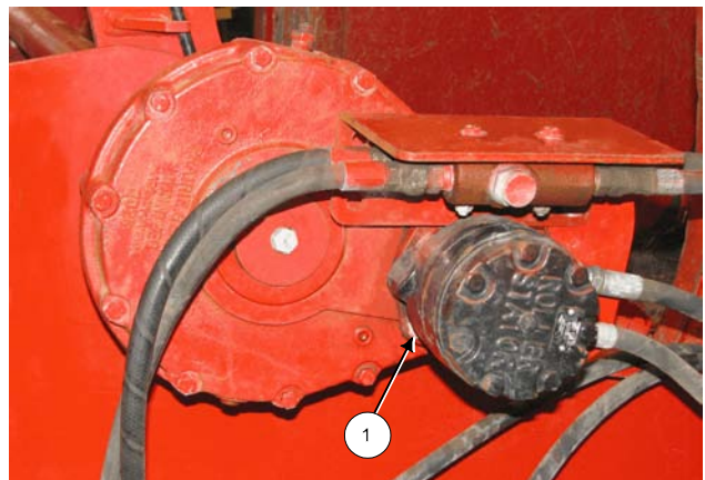
Check that Motor Mount Bolts Are Tight
