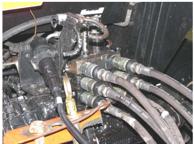
Disconnect Hydraulic Hoses & Electrical
