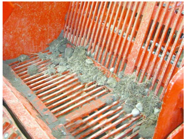
Remove Debris From Bucket
