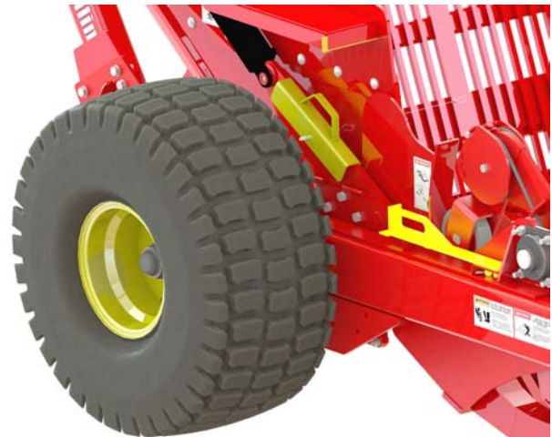
Check the Condition of the Tires & Pressure
