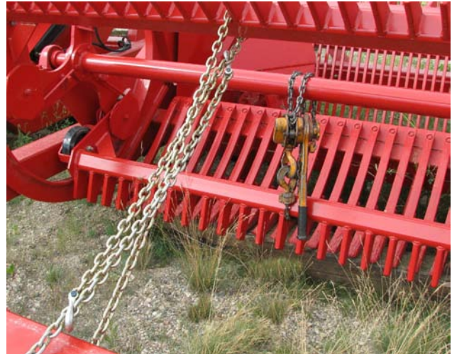
Winch The Lodged Bat-Remove Spring Pressure 08193
