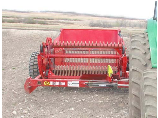
Hitch Position 2 - Single Tractor Tires
