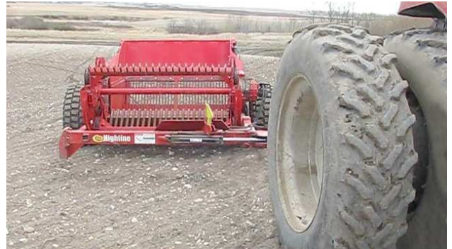
Hitch Position 1 - Dual Tractor Tires
