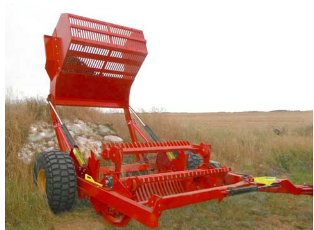
Rock Bucket in Dumping Position
