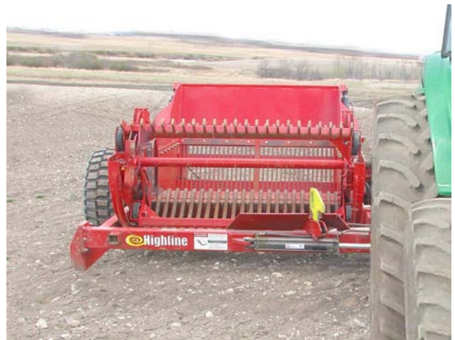
Hitch Position 2 -Single Tractor Tire
