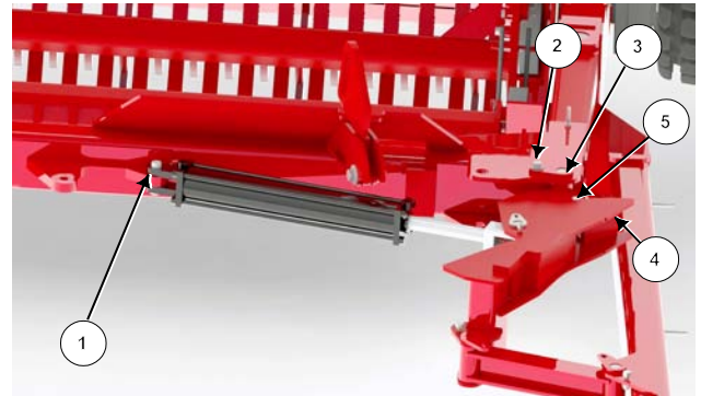
Remove Pins (Position 1) to Adjust Hitch Position 215254C
