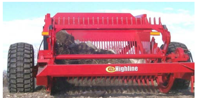
Reverse Reel & Raise Apron to Remove Rock 214011
