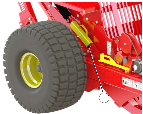
Bucket Lock in Storage Position
