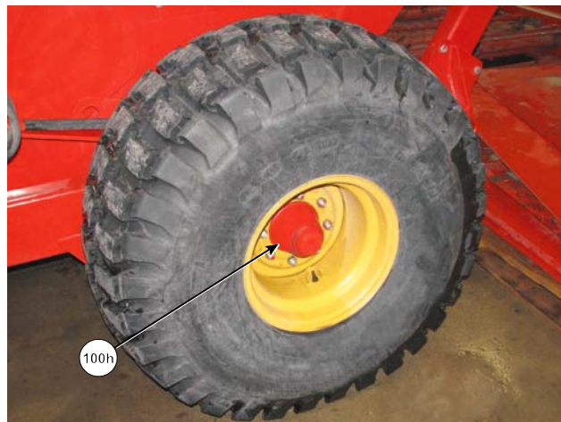
Grease Wheel Hubs
