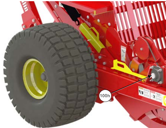
Grease the Reel Bearing - Right Side
