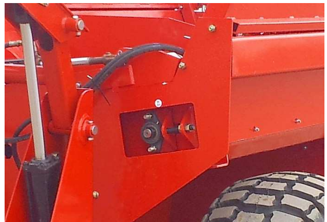
Remove Material - Upper Rear Bearing
