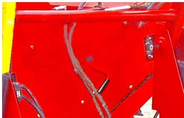
Replace Twine Cutter Into Storage Position
