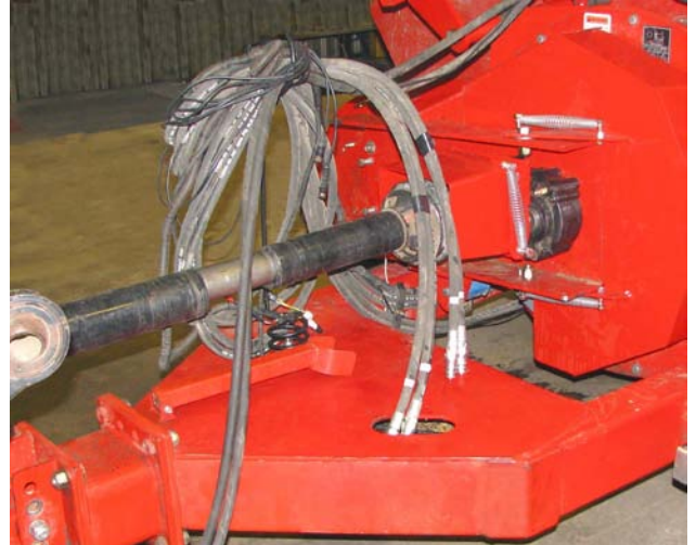
Hydraulic Hoses and Electrical In Holder
