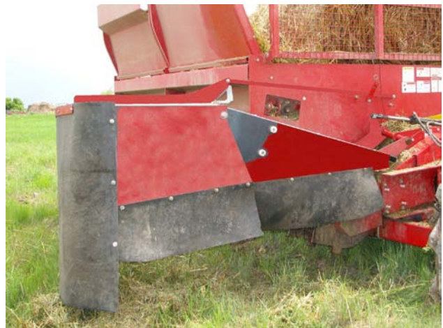
Deflector for Windrow or Bunk Feeding
