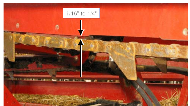
Adjust the Chain Tension
