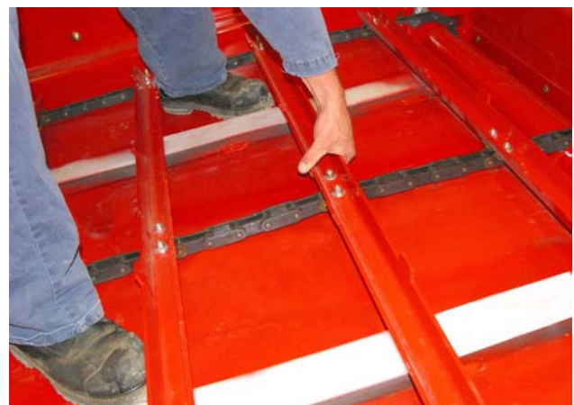
Check Tension of the Feeder Chain
