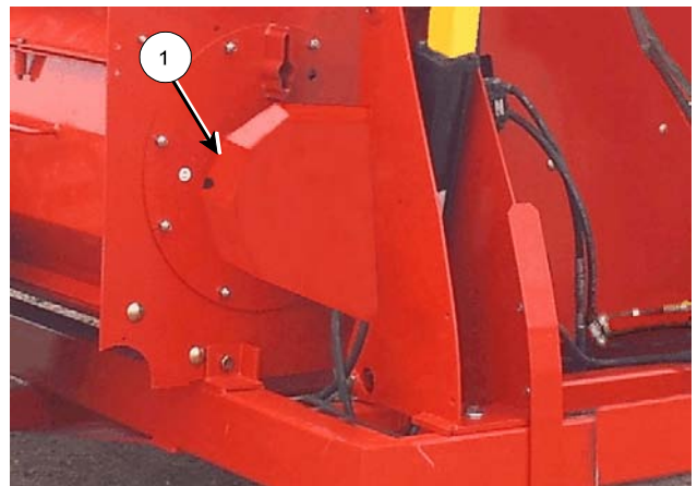
Remove Rear Upper Shield
