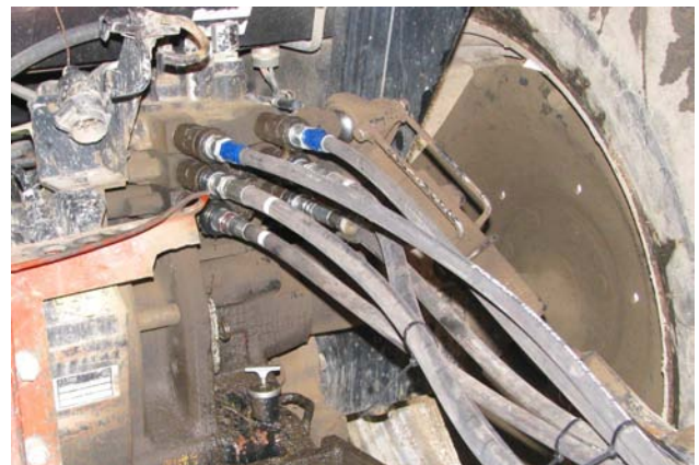
Disconnect Hydraulic Hoses & Electrical
