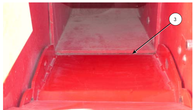
Ensure Door is Below Blower Exit
