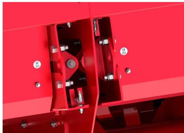
Adjust Front Feeder Chain Tension (Middle Wall) 213137
