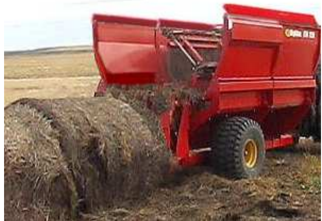
Rear Tub Bale Transfer Chains Rising
