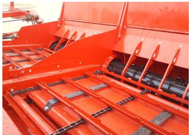
Check the Condition of the Feeder Chains
