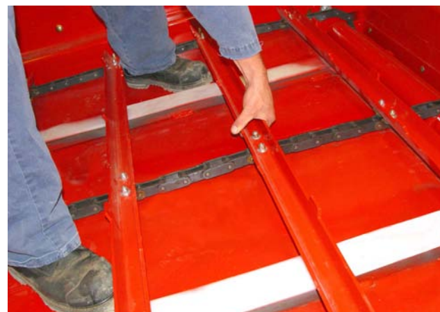
Check Tension of the Feeder Chain
