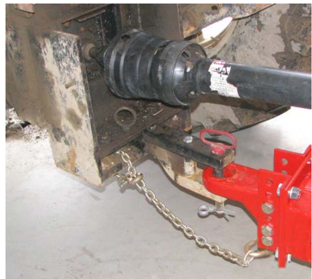
Connect Driveline to PTO
