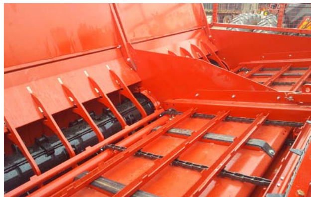
Oil the Feeder Chains to Prevent Rusting
