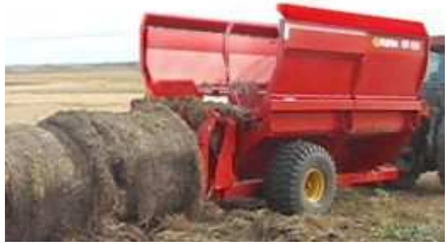
Align Bale to be Loaded
