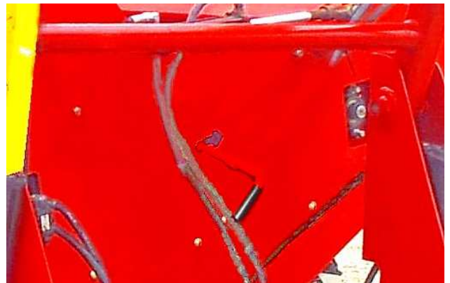
Remove Twine Cutter from Storage
