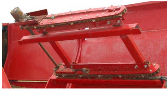
Remove Material & Oil Chains
