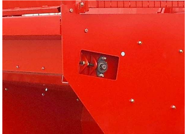
Remove Material - Upper Front Bearing
