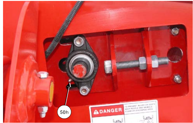
Grease Upper Feeder Chain Bearings
