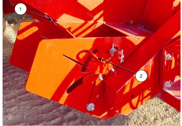
Door in an Upper Slot For Feeding
