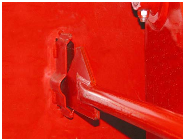
Insert Twine Cutter with Blade Up
