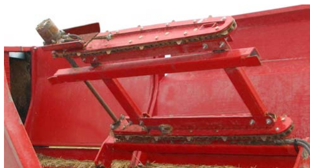
Bale Transfer In Rear tub
