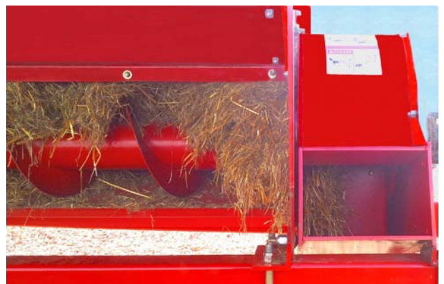
Remove Materials In Auger and Blower
