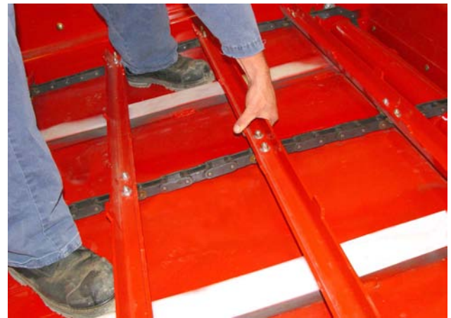
Check Tension of the Feeder Chains
