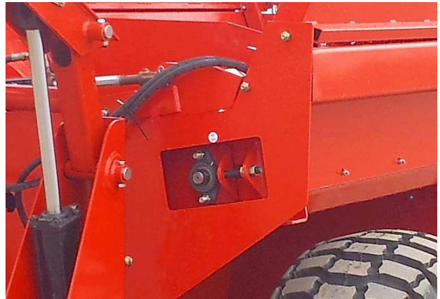
Remove Material - Upper Rear Bearing
