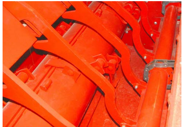
Move Flails Blocking the Knife Path
