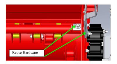
13) Starting at the front of the processor start to install the guard rods to the adjustment bar. Inset the bolts with the nut at the front side of the guard rod. Tighten the nut until it is secure on the bolt. Check to make sure the guard rod moves easily in the slot on the adjustment rod. The ears on the adjustment bar may need to be adjusted to allow the guard rod to move freely.
