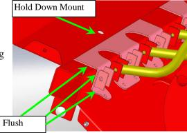
7) Insert the supplied carriage bolt into the top mounting hole. Measure the distance in between tabs. Distance should be 3  $1/16" \pm 1/16"$  inside mounting tabs or  $53/8" \pm 1/16"$  center to center. Tighten top carriage bolt.
