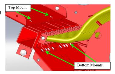
12) Install the new adjustment bar and mount the old handle using the old hardware.
