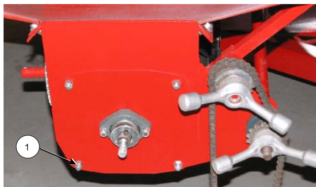
Fasten the Auger End Plate
