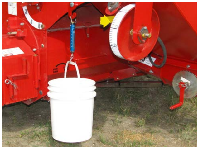
Weigh Sample, Subtract Empty Bucket Weight 212108
