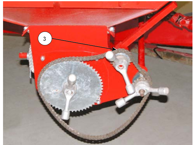
Loosen and Remove the Drive Chain
