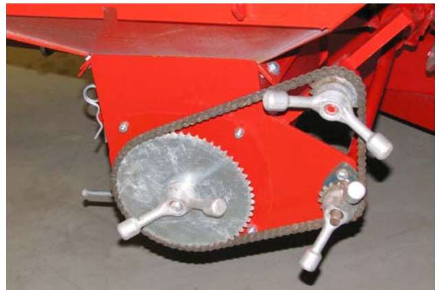
Lubricate the Auger Drive Chain
