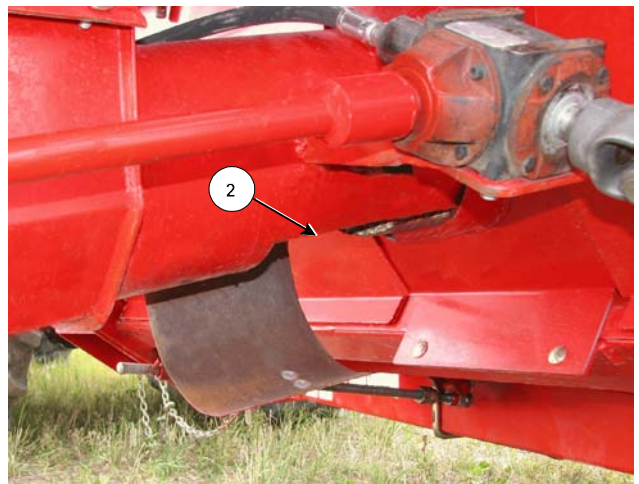
Open the Calibration Hole
