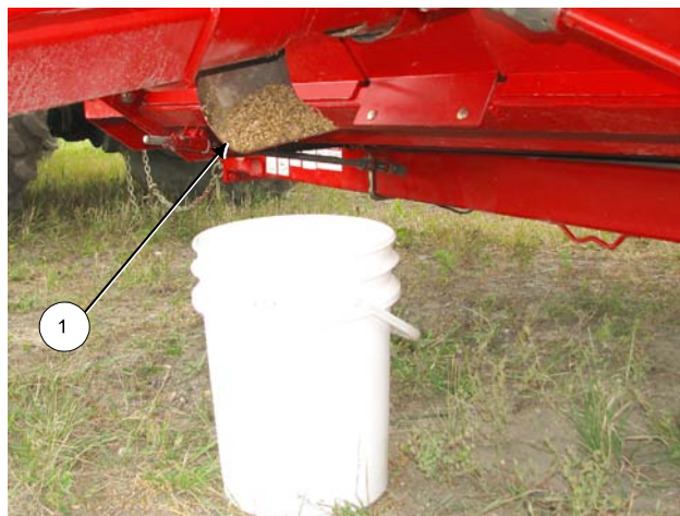
Auger Tube and Chamber Cleanout
