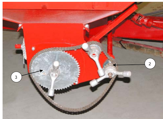
Install the Driving and Auger Sprocket
