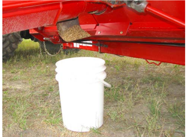
Place Collection Bucket Under Calibration Hole 220010
