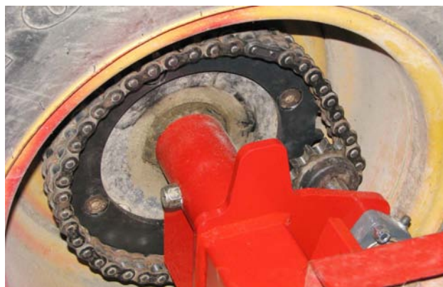
Remove Twine From Drive (CFR 651 Shown)
