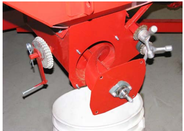
Pull Out Auger To Drain Tank
