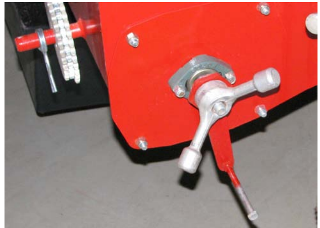
Install Auger Crank Handle
