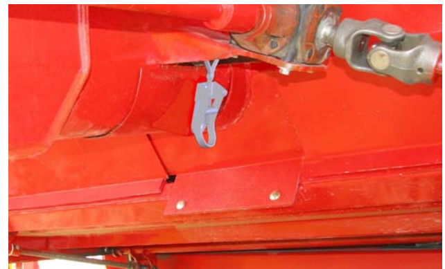
Replace the Cover on Calibration Hole 220008
