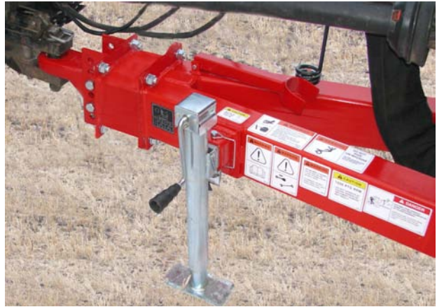
Jack on Hitch - Raise Hitch
