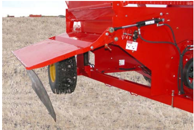
Set the Upper Deflector Door (Windrowing Shown) 212005
