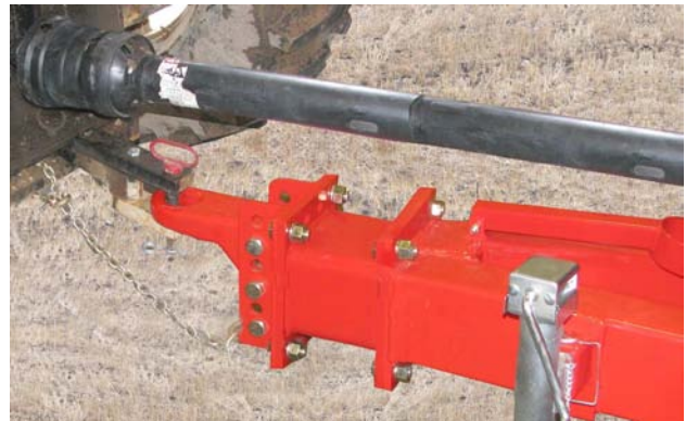
Remove Driveline and Safety Chain
