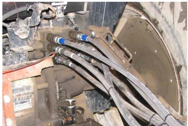
Disconnect Hydraulic Hoses & Electrical
