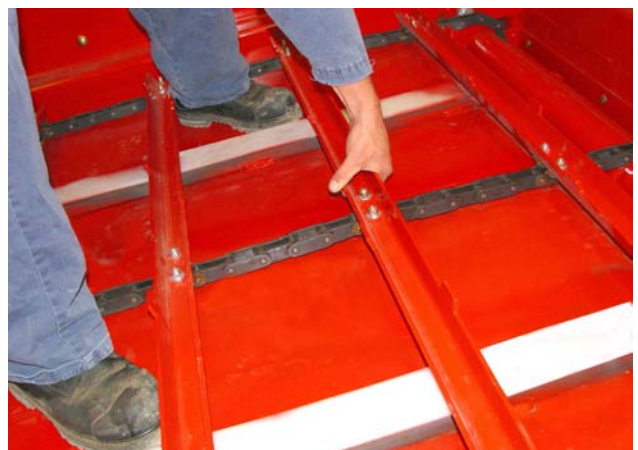
Check Tension of the Feeder Chain
