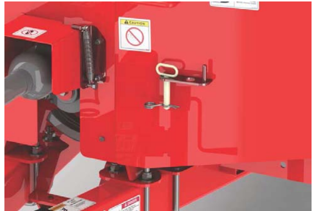
Store Lock Pin on Outside of Shield
