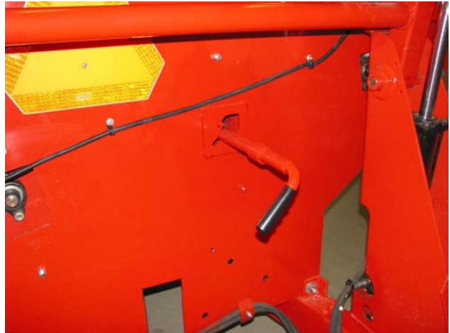
Replace Twine Cutter Into Storage Position
