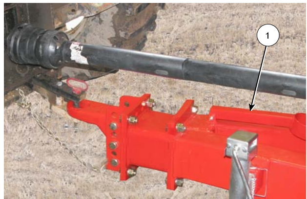
Connect Driveline to PTO
