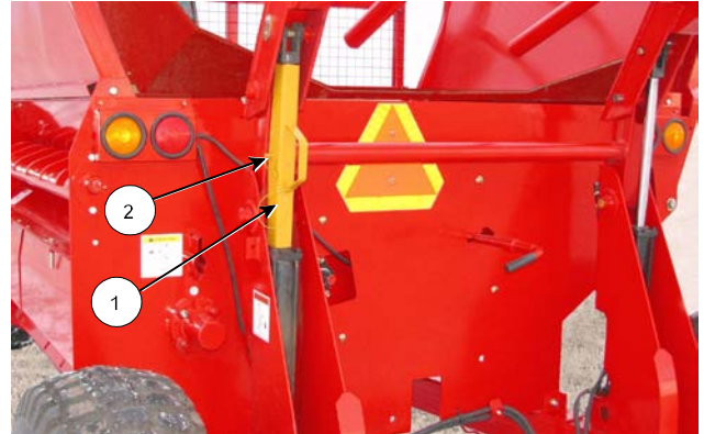
Fork Cylinder Resting on Lock
