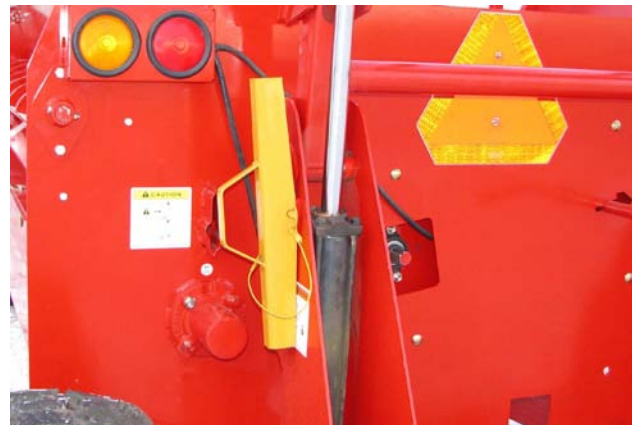
Remove & Store Cylinder Lock (No Feedchopper)
