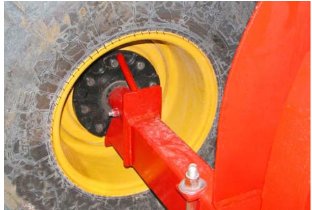
Remove Twine From the Spindle and Hub
