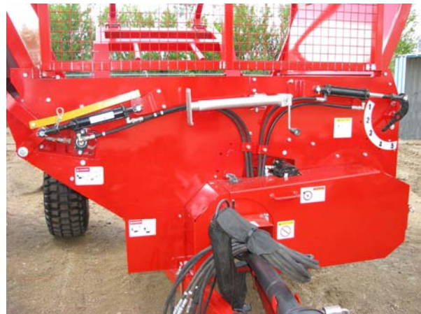
Check All Hydraulics
