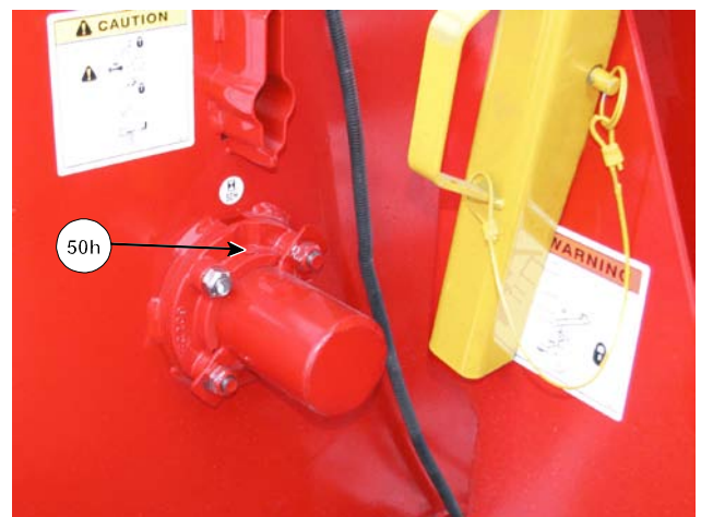
Grease Rear Flail Drum Bearing
