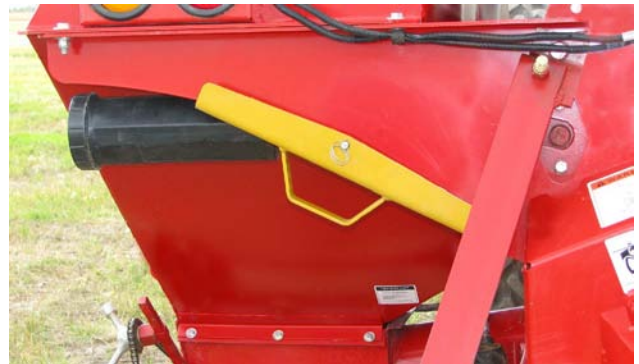
Cylinder Lock Stored (With Grain Tank)
