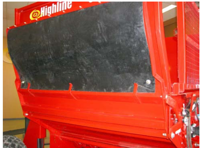
Raise Deflector Door to Transport Position
