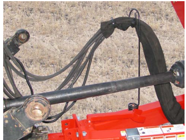
Hoses and Electrical in Support Arm
