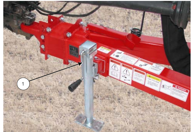
Lift Hitch with the Jack
