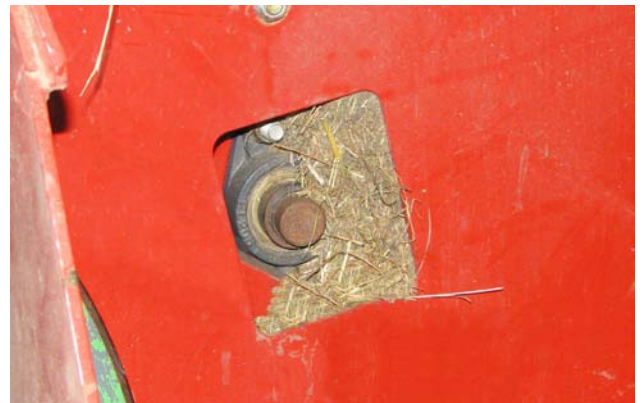
Remove Material - Lower Chain Bearing
