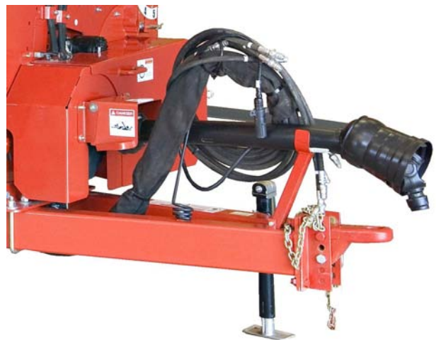
Hoses and Driveline in Supports
