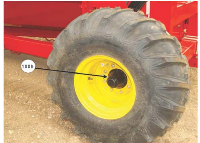
Grease Hubs on Both Spindles
