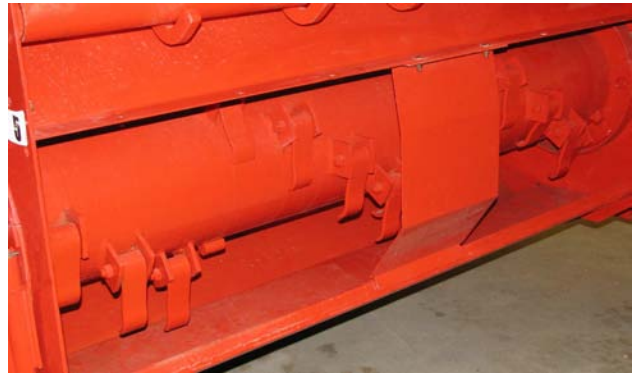
Clean Debris and Check Drum and Flails
