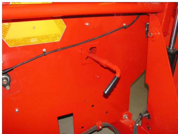
Replace Twine Cutter Into Storage Position
