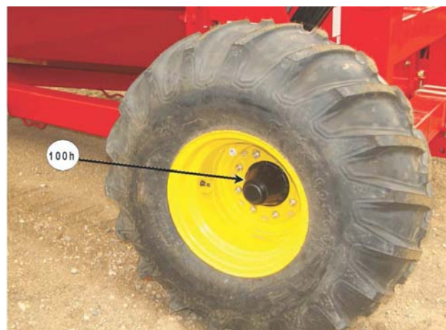
Grease Hubs on Both Spindles
