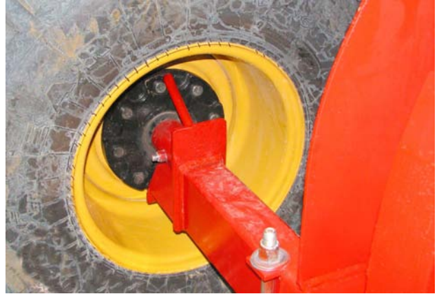
Remove Twine From the Spindle and Hub
