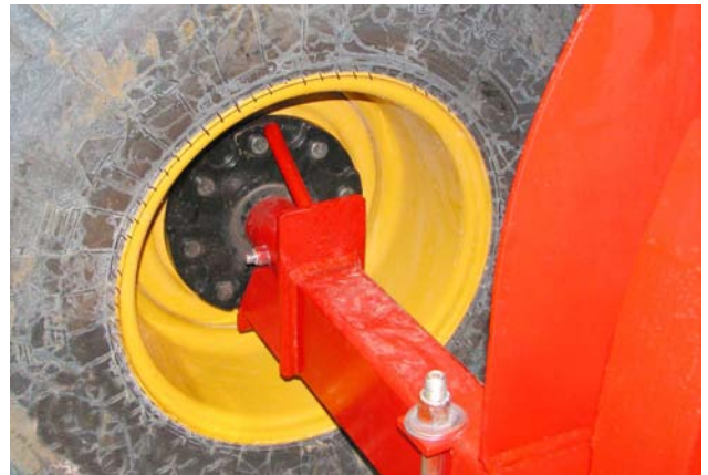
Remove Twine from the Spindle and Hub
