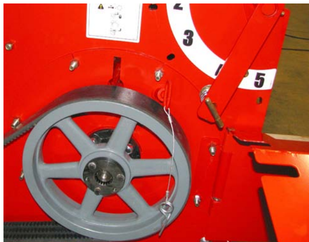
Move Flail Guard Rod Lever (to less than 5)
