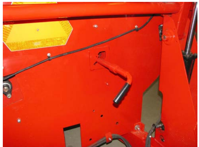
Remove Twine Cutter from Storage
