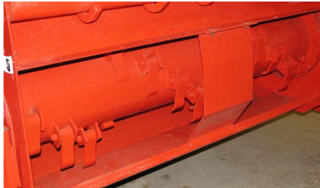
Clean Debris and Check Drum and Flails
