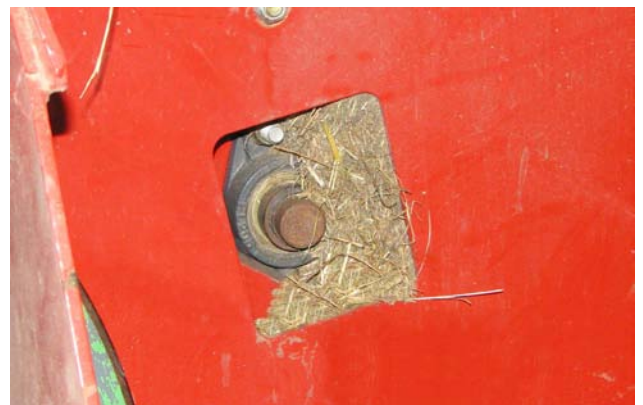
Remove Material - Lower Chain Bearing
