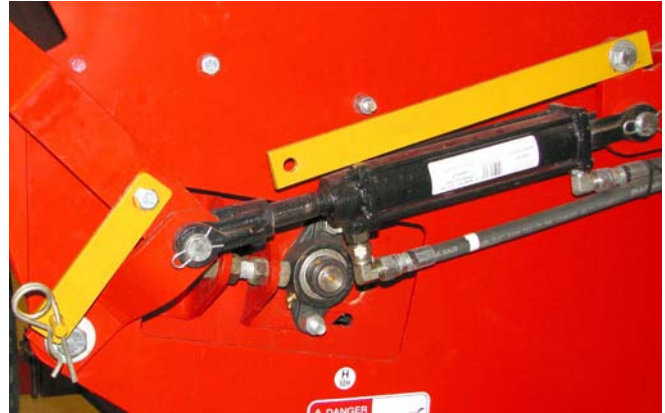
Remove Lock Pin on Deflector Door
