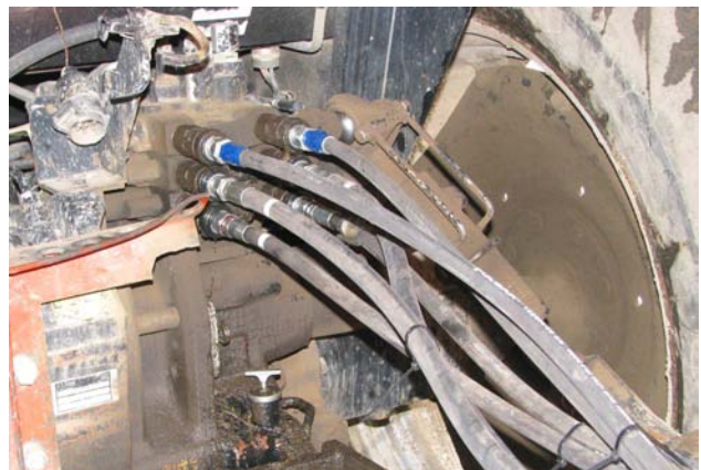
Disconnect Hydraulic Hoses & Electrical
