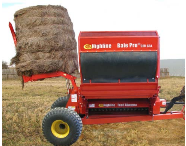
Raise Bale into Processor Tub
