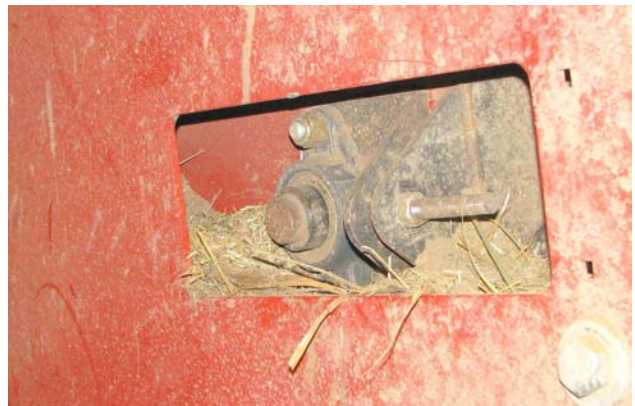
Remove Material - Upper Chain Bearing
