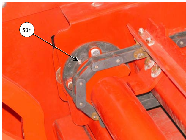
Grease Lower Chain Bearing (Inside Tub)
