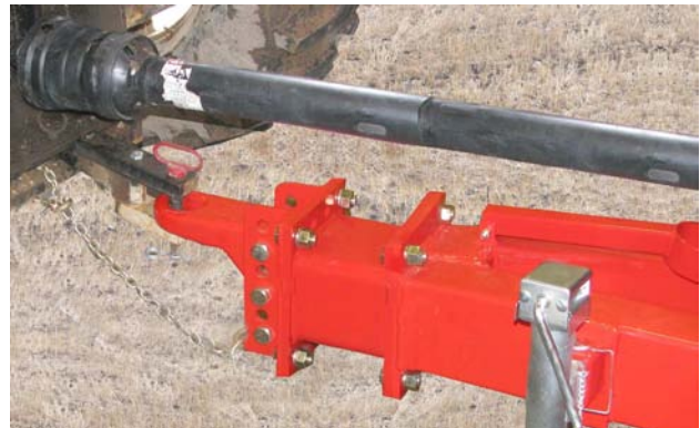
Remove Driveline and Safety Chain
