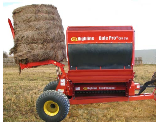
Stop the Feeder Chain When Loading
