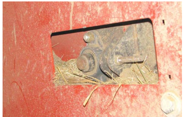
Remove Material - Upper Chain Bearing
