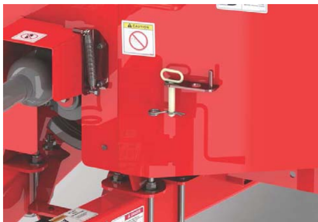
Store Lock Pin on Outside of Shield
