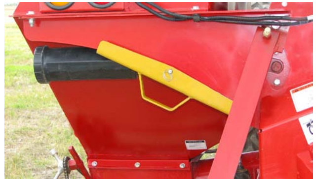
Cylinder Lock Stored (With Grain Tank)
