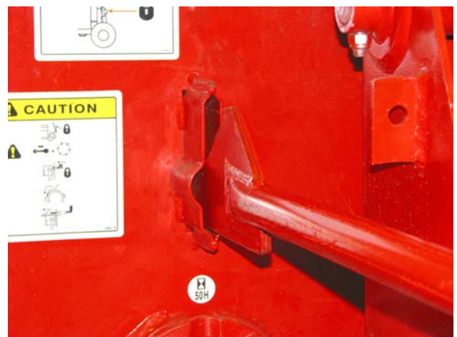
Insert Twine Cutter with Blade Up
