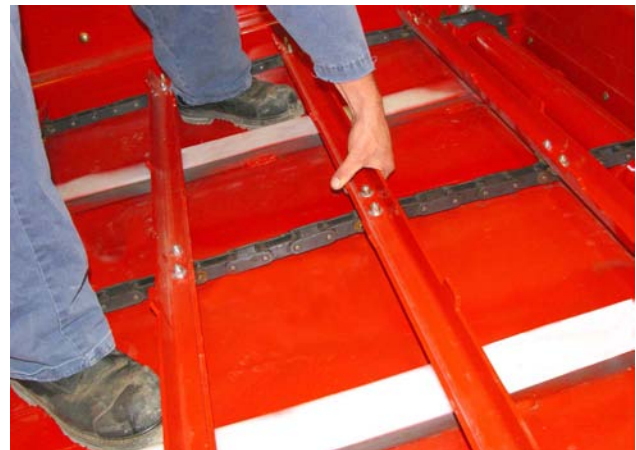
Check Tension of the Feeder Chain
