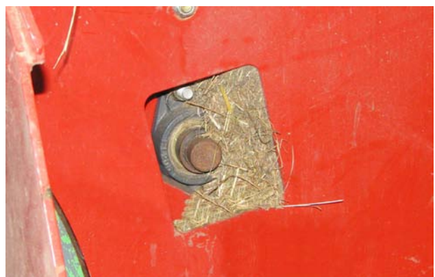
Remove Material - Lower Chain Bearing
