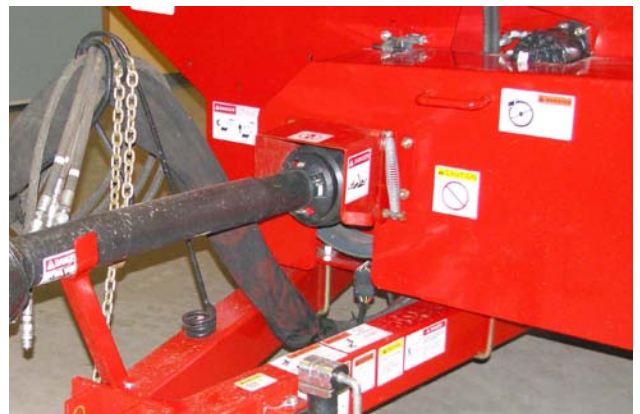
Ensure Driveline Shields are in Place
