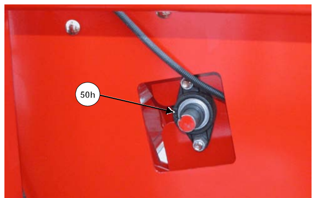
Grease Feeder Chain Bearing (Outside of Tub)
