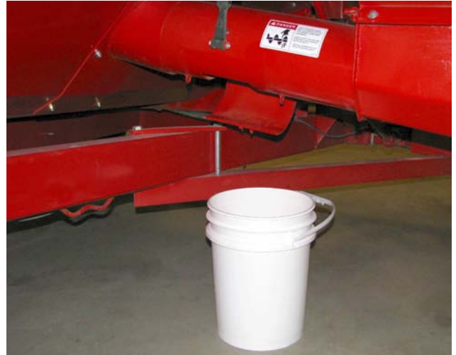
Place Collection Bucket Under Calibration Hole 211177
