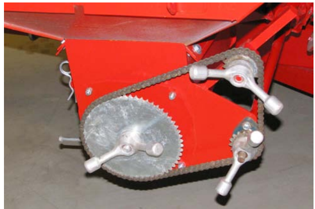
Lubricate the Auger Drive Chain
