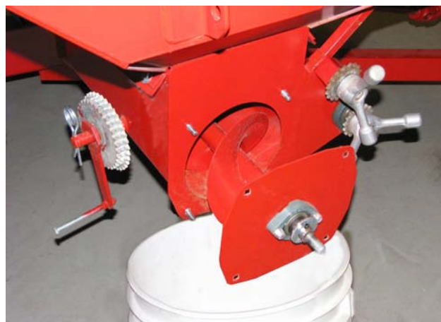
Pull Out Auger To Drain Tank
