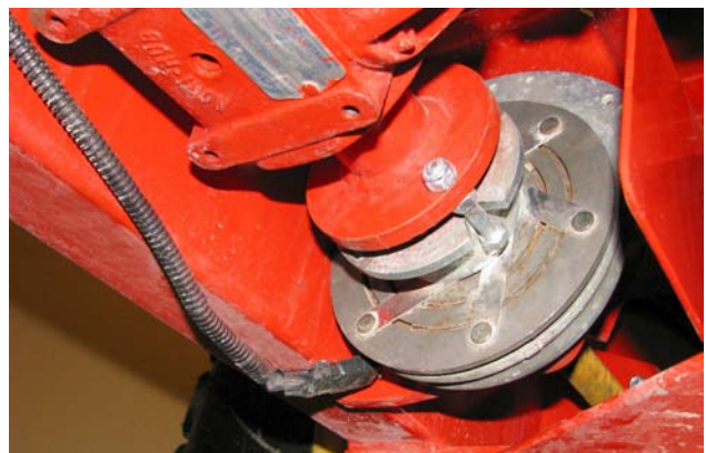
Remove Debris from Electric Clutch
