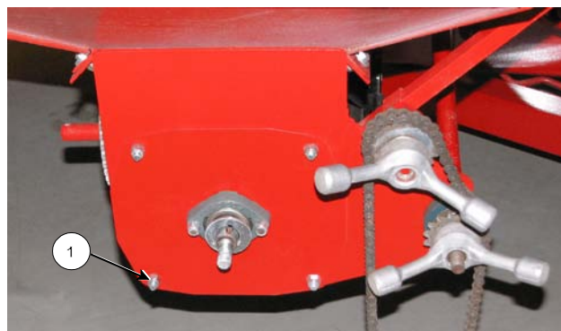
Remove Nuts From End Plate
