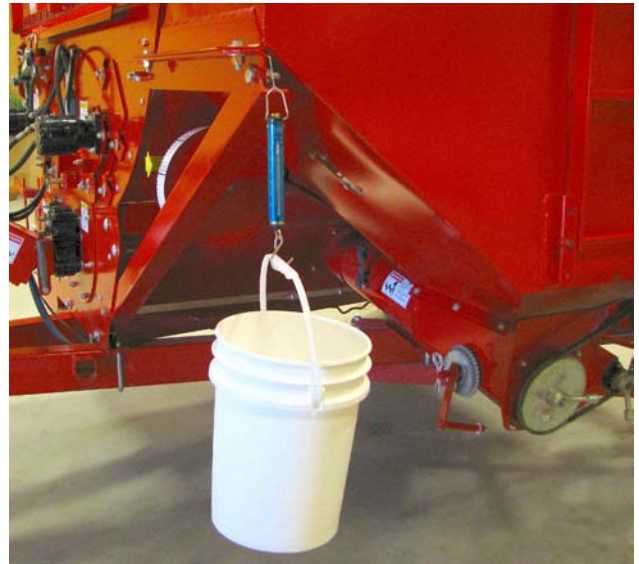
Weigh Sample, Subtract Empty Bucket Weight 211171
