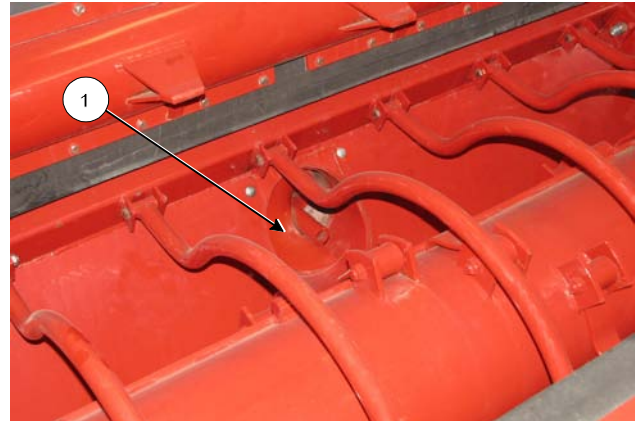
Check the Auger Discharge
