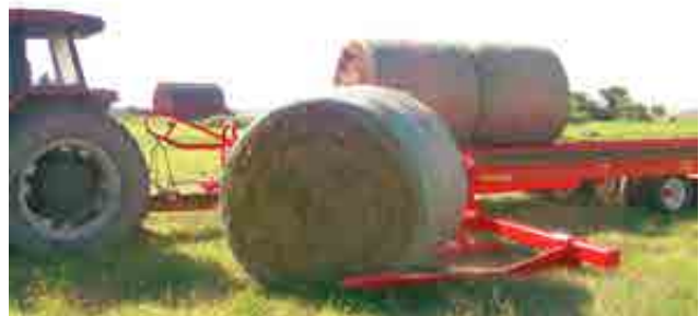
Figure 5.5: Bale can be rotated by the lift arm
