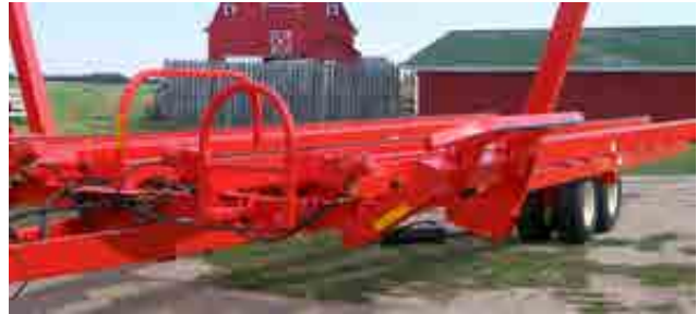
Figure 7.1: Park, clean and lower the Bale Mover bed onto the frame
