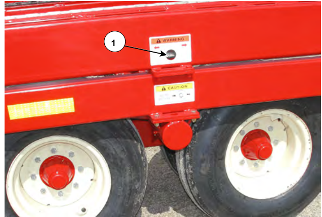
Check Tension of All the Chains
