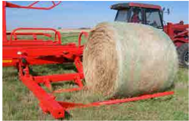
Figure 5.4: Drive up to a bale with the arm lowered
