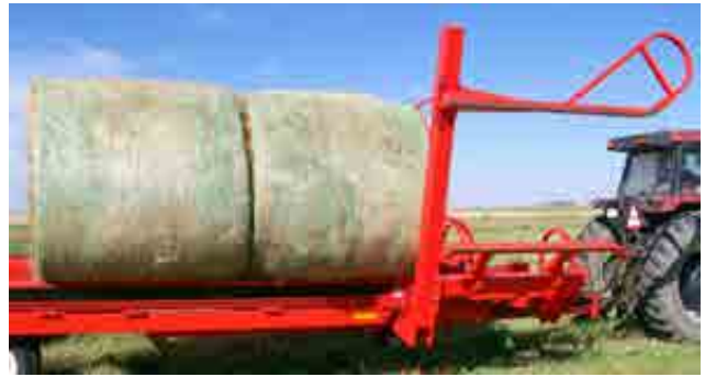
Figure 5.8: Move the bales back on the chain rails
