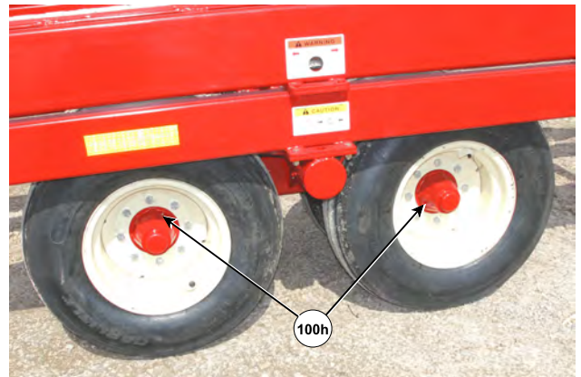
Grease Hubs on all Spindles
