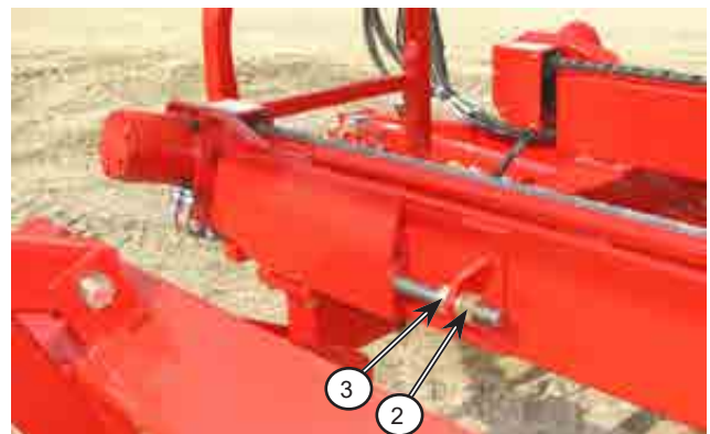
Figure 6.7: Adjust the chain tension
