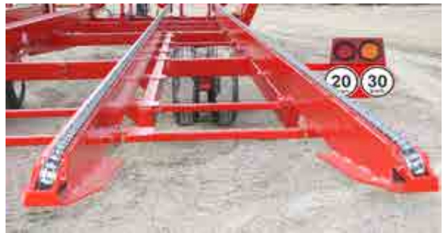
Figure 4.9: Check the condition of the bale chains
