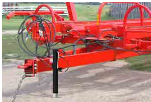
Figure 7.3: Raise the hitch with the jack
