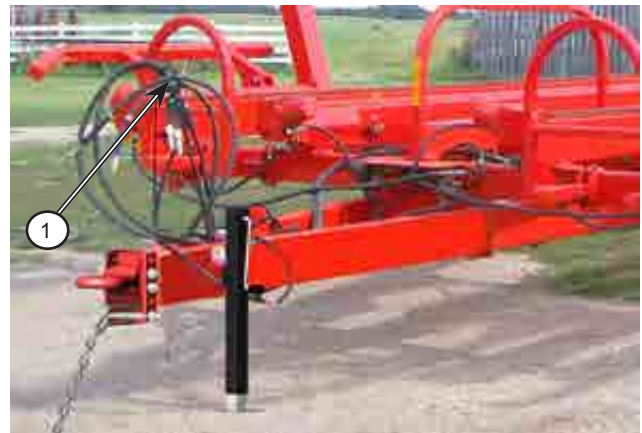
Figure 7.4: Secure hoses and cables to hose holder
