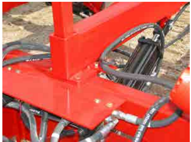
Figure 4.19: Check all hydraulic connections
