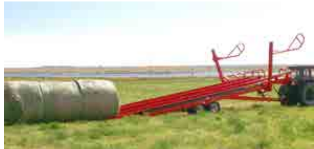
Figure 5.18: Tilt bed to fully raised position
