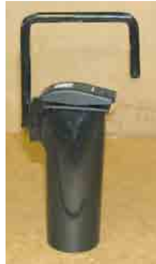
Figure 5.17: Control Switch - bed tilt and reload
