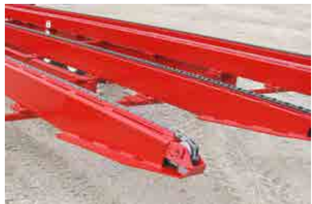
Figure 7.5: Oil the chains to prevent weathering
