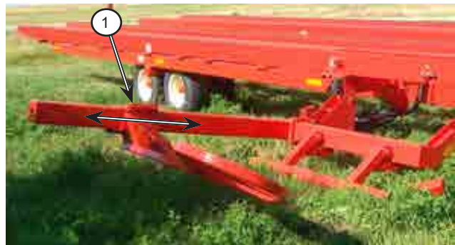
Figure 5.2: Slide clamp for bale width
