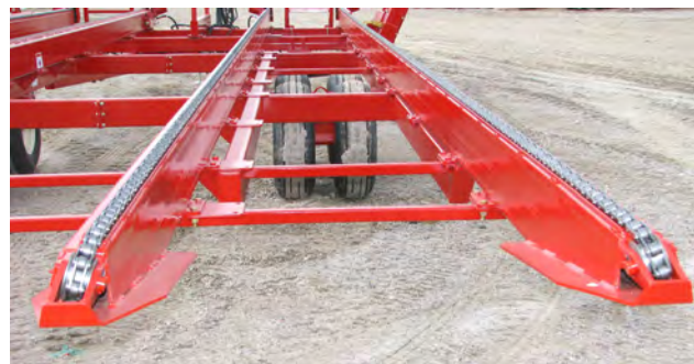
Lubricate the Bale Chains
