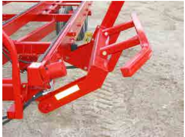
Figure 4.15: Check that the lift arm operates freely
