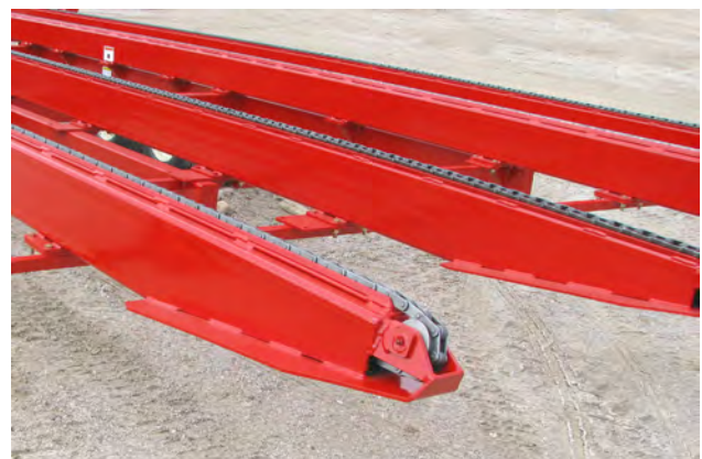
Oil the Chains to Prevent Weathering
