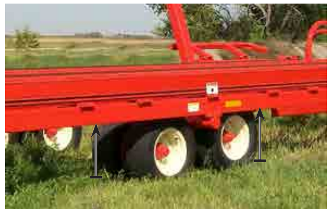
Figure 6.8: Jack on frame to change tires
