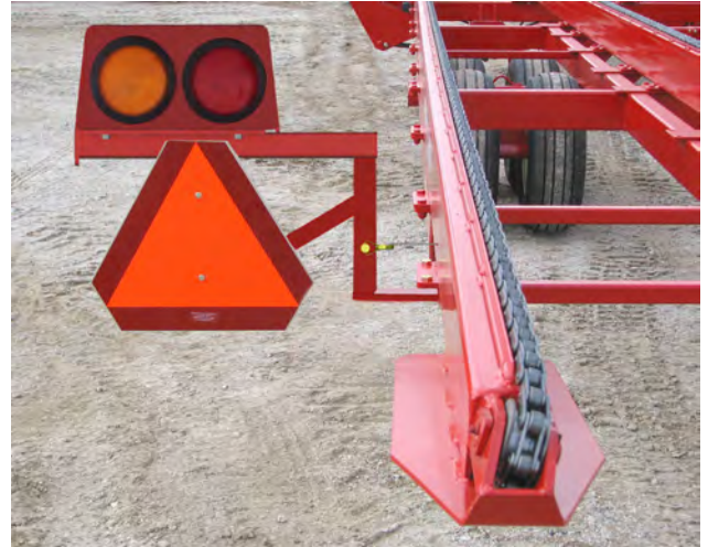
SMV/Light Bracket in Transport Position Ensure SMV is Clean and Visible Ensure the Lights are Working
