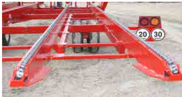
Figure 4.17: Check the operation of the bale chains
