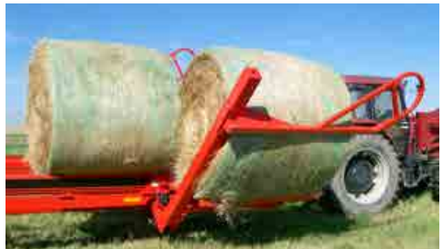
Figure 5.7: Lift the bale onto the bed
