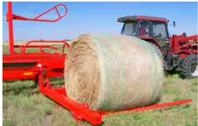
Figure 5.6: Drive forward until fork is under the bale
