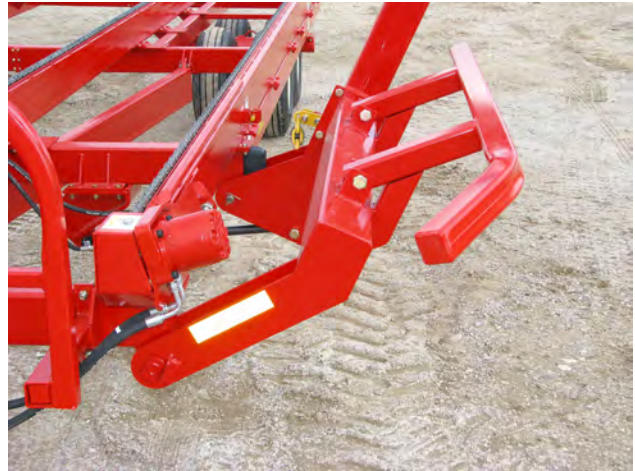
Check that Lift Arm Operates Freely
