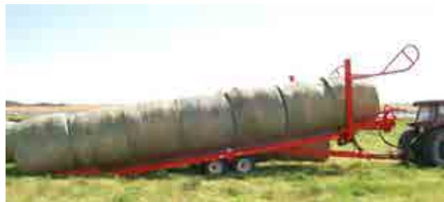
Figure 5.19: Engage the bale roller chains
