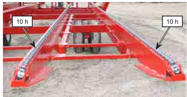
Figure 6.3: Lubricate the bale chains
