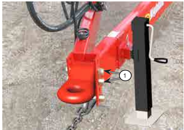
Figure 4.2: Adjust position of the tongue
