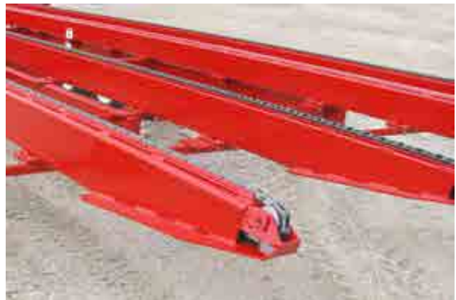
Figure 4.10: Chain is around the end roller
