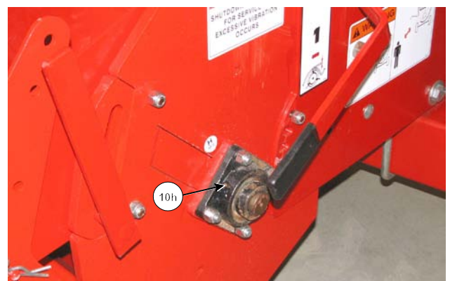
Grease Front Rotor Bearing
