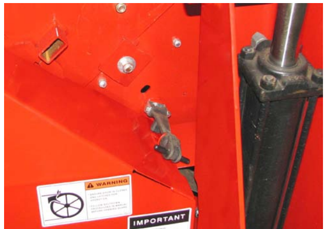
Close and Fasten Access Door
