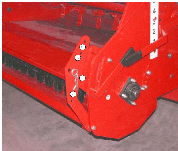
Lower Door to Pass Material Over Chopper
