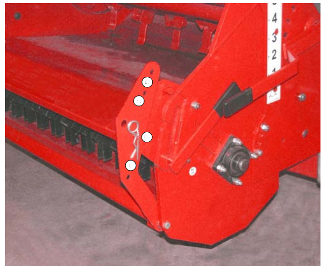
Lower Door to Pass Material Over Chopper
