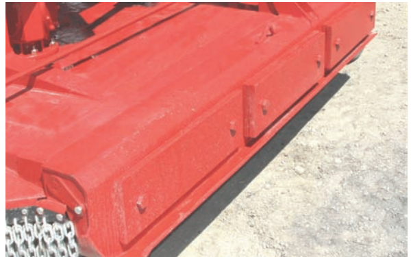
Inspect Center Skid & Counterweights (10 Foot)
