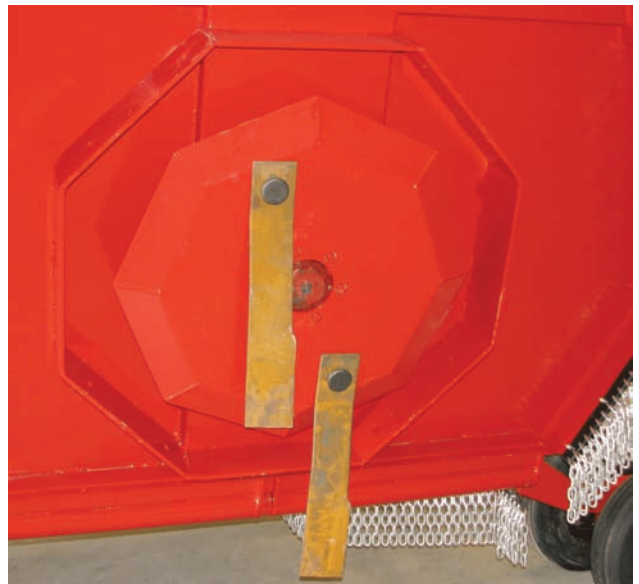
Inspect Blades & Hardware
