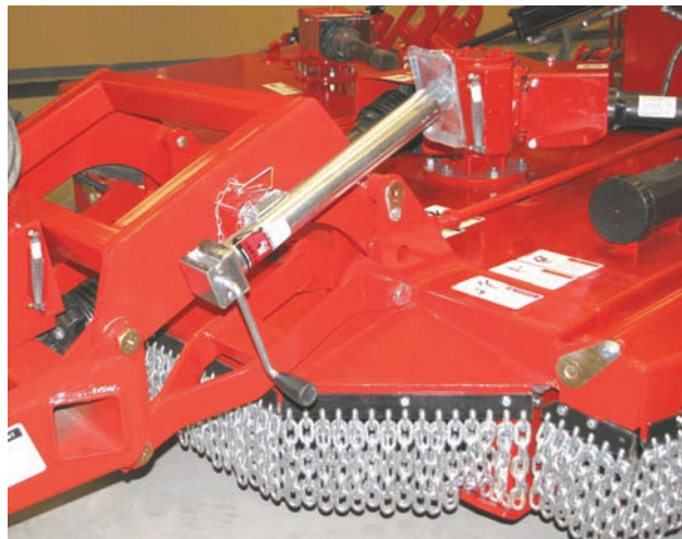
Hitch Jack in Storage Location (SL Shown)
