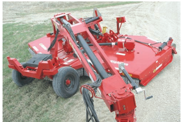
Rotate Deck Into Cutting Area
