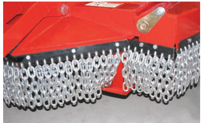
Inspect the Center Section Plates
