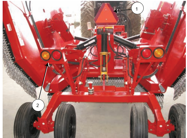
Ensure SMV is Visible & Lights are Working
