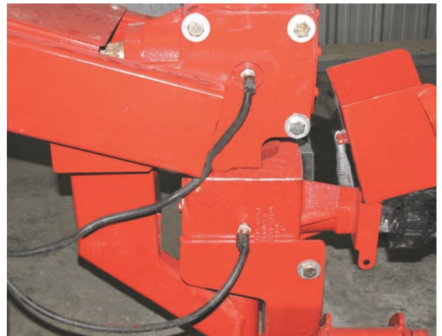
Check Sensors in Gearboxes (RCH Hitch)
