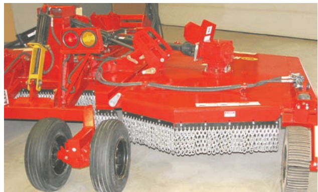
Inspect Hydraulic Cylinders and Hoses
