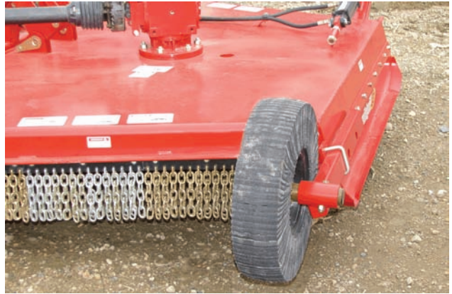
Inspect Wing Skid Plate Wheel
