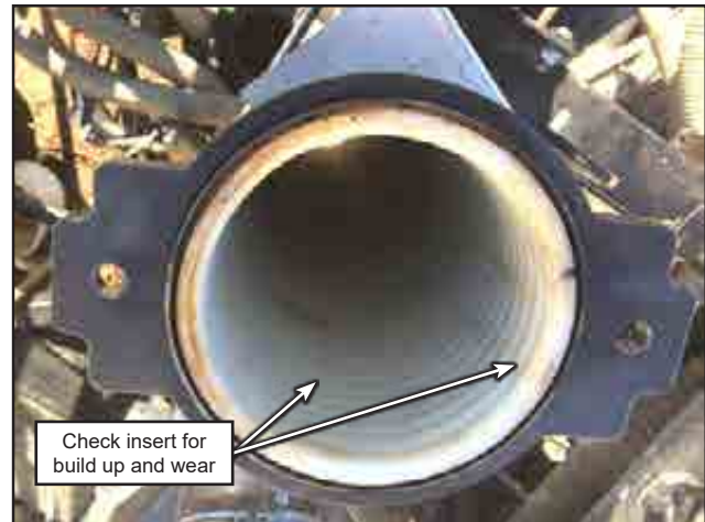
Figure 1.11 - EvenStream Insert Inspection
