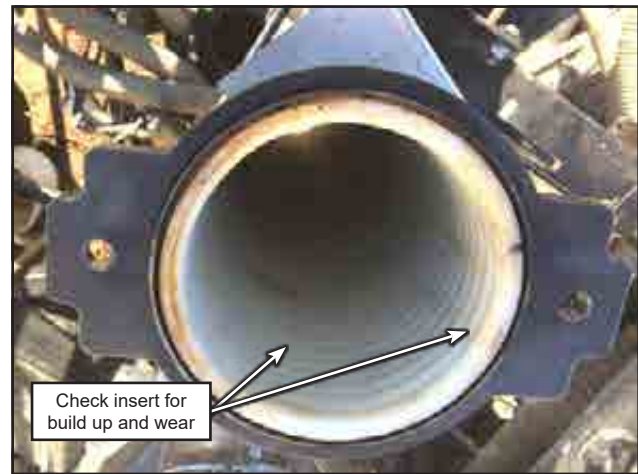
Figure 1.15 - EvenStream Insert Inspection
